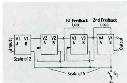
Fig. 5. Scale of 5 coupled to scale of 2 makes circuit into a decade counter.
