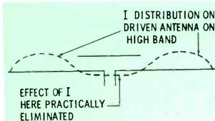
Fig. 10. On high band, parasitic element minimizes effect of reverse current.
