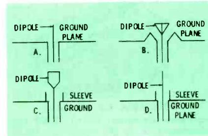
Fig. 2. "Sleeve-dipole" principle developed from whip-and-ground-plane array.
