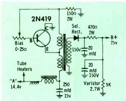
Fig. 5. Power supply of FM tuner uses 2N419 transistor as 400-cps oscillator.
