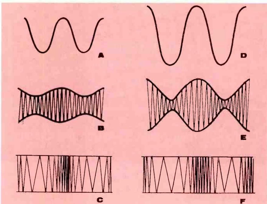
Fig. 1. Amplitude and frequency modulation of an RF carrier by 1-kc audio signals of two different strengths.
