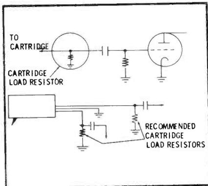
Fig. 6. Schematics indicating load resistors for monaural and stereo cartridges.
