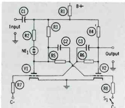
Fig. 1. Eccles-Jordan will change conduction status with each negative pulse.
