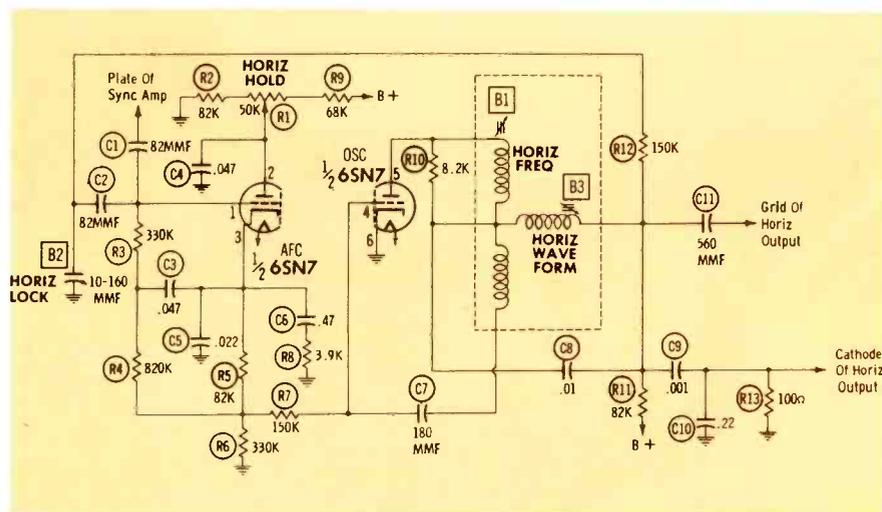
Fig. 1. Schematic of popular pulse-width AFC and oscillator circuit.
