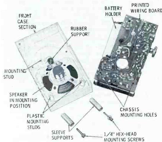
Fig. 6. Westinghouse H-655P5 chassis removed from the front section of its plastic case.
