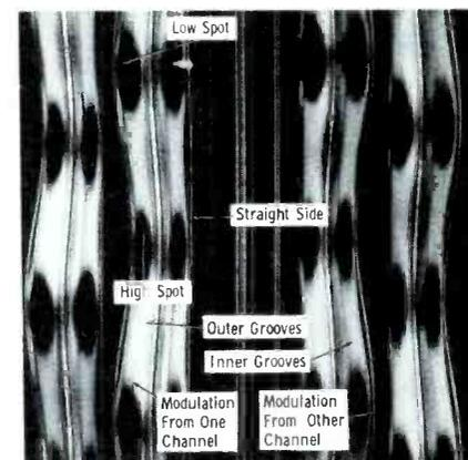
Fig. 3. Photomicrograph of stereo grooves cut with single modulation frequency. (Courtesy of Westrex Corp.)
