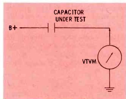
Fig. 4. Setup for testing paper capacitors for leakage uses VTVM and B+ source.
