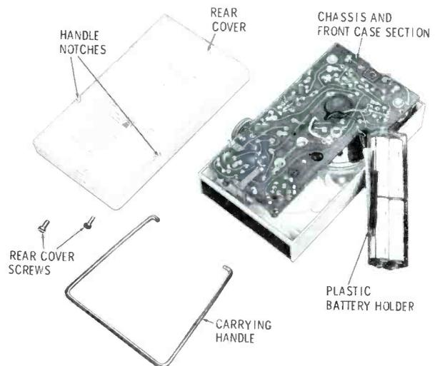
Fig. 3. To get at the batteries of the Westinghouse H-655P5, the handle, two screws, and the rear cover must be removed.
