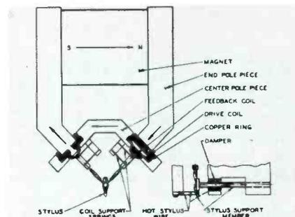
Fig. 2. Basic recording head showing coil placement and attachment to stylus.
