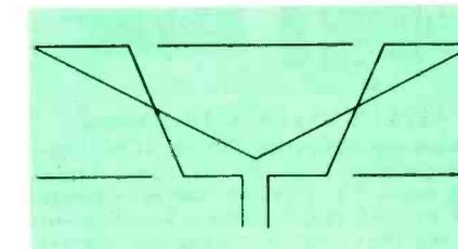
Fig. 6. Wing dipole in final form. Decoupled reflectors are sometimes omitted.
