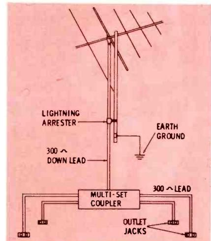
Fig. 1. Shop antenna system for strong signal areas where noise level is low.
