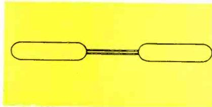
Fig. 11. In actual Finney arrays, parasitic element takes the form of "bowtie."
