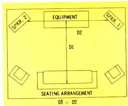
Fig. 7. Example of speaker placement with respect to listening area for stereo.
