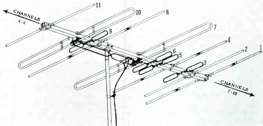
Fig. 13. Finney TCR-1 array receives selected signals from opposite directions.
