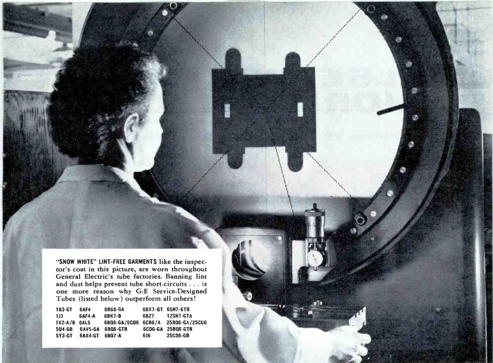
"SNOW WHITE" LINT-FREE GARMENTS like the inspector's coat in this picture, are worn throughout General Electric's tube factories. Banning lint and dust helps prevent tube short-circuits . . . is one more reason why G-E Service-Designed Tubes (listed below) outperform all others!
