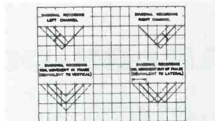
Fig. 1. Basic record cuts using the Westrex 45/45 system of stereo recording.
