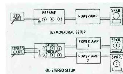
Fig. 4. Block diagram comparison between monaural and stereo playback systems.
