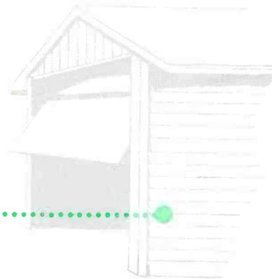
Before you begin an actual installation of a garage-door opener, here are some hints that will save you time and trouble. First of all, almost any door-operator mechanism has a minimum headroom requirement. By headroom, we mean the space above the high-arc point (highest point in the door's travel). Check this clearance and make sure it is sufficient for the unit you plan to use.
