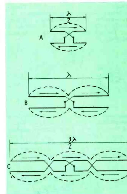
Fig. 4. Steps used in developing broad-band response for Trio's wing dipole.
