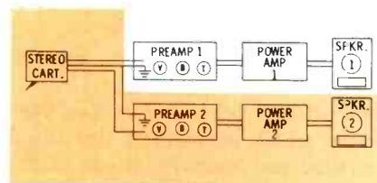
Fig. 5. Block diagram of changes necessary to convert monaural system to stereo.
