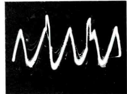
(B) AFC grid waveform.
