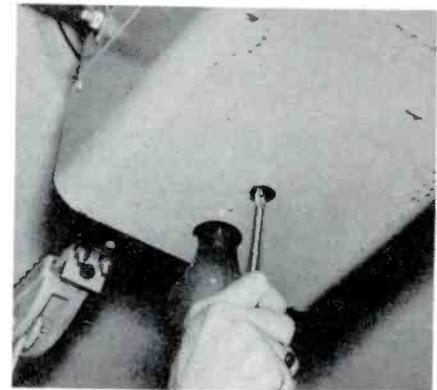
**Adjusting Perma-Power Clutch**
