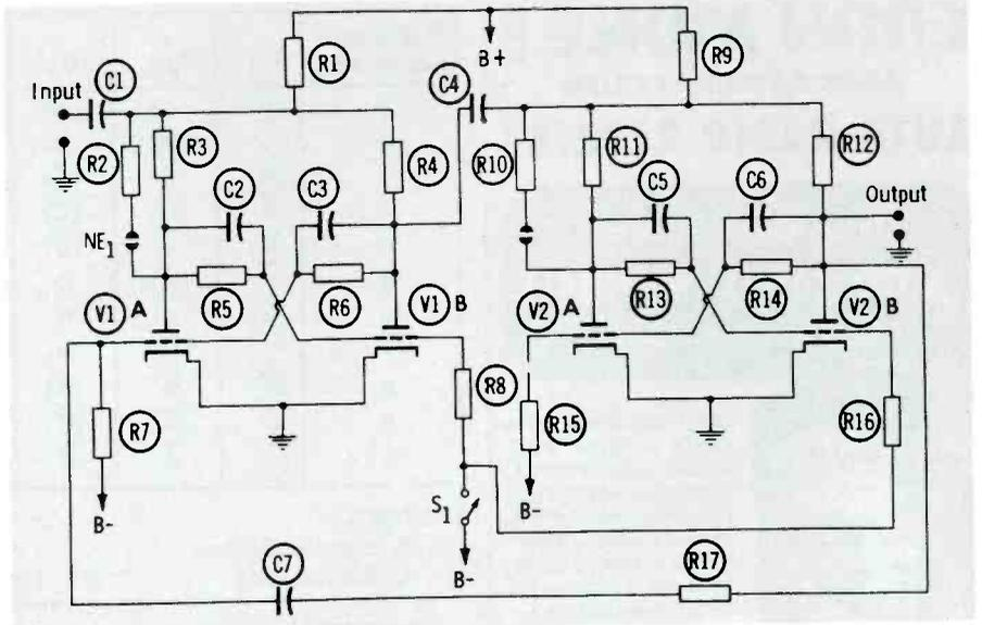
Fig. 3. Positive feedback from 2nd Eccles-Jordan reduces scale from 4 to 3.
