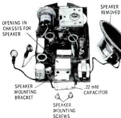
Fig. 8. Speaker of Silvertone 9202 must be removed to make parts accessible.
