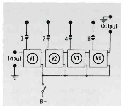
Fig. 2. Four Eccles-Jordan stages in series provide a reduction factor of 16.
