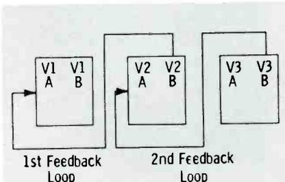
Fig. 4. Two consecutive feedback loops change reduction factor from 8 to 5.
