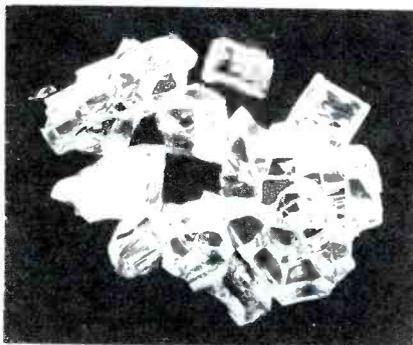
*Chalk up another one for the cowboys! Seriously, our guess is that the glass was installed in such a way as to place it under excessive strain. After the receiver had been in operation for some time, heat evidently caused expansion of the frame holding the safety glass, thus increasing the strain on the glass to the breaking point.*
