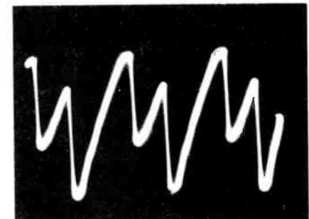
(B) Oscillator plate waveform.
