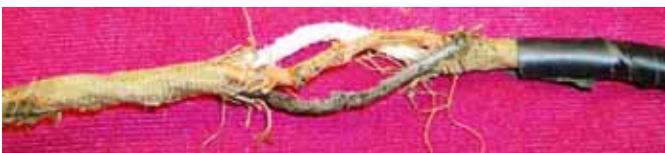
Photo of a badly worn resistance line cord
