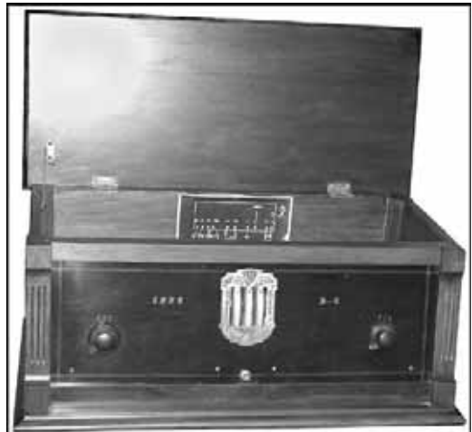
Figure 1. The Long Model B5, ca. 1926, has NA-ALD brand dials, five Type 01-A tubes, three binocular coils, and a thumbwheel dial.
