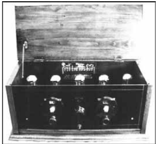
Figure 2. The Long Model F5, a 5-tube TRF with two Kurz-Kasch style dials, with the lid up.
