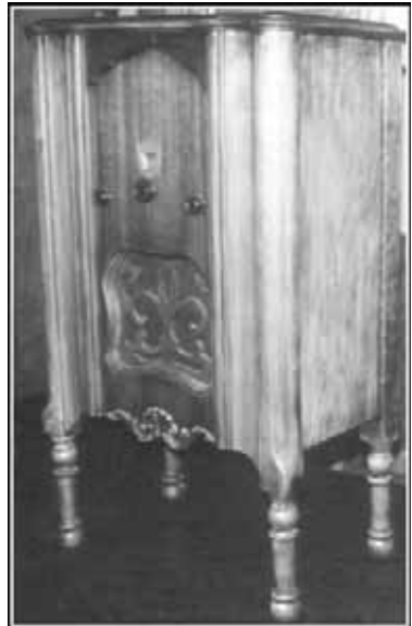
Figure 4. This 6-tube console with a Jensen electrodynamic speaker has no visible model number.
