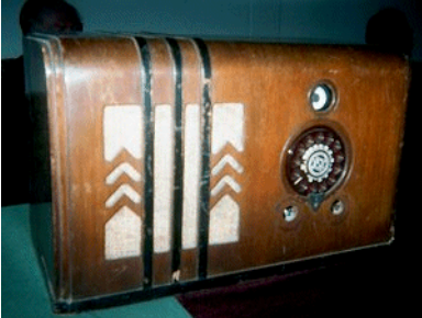
Myron White: Montgomery Ward 6V farm set with sync. vibrator and 150 ma tubes.
