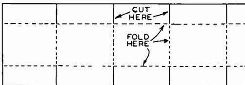
FIG. 1. Wooden form and fish-paper liner for winding transformer. Fish-paper is cut to size and wrapped around block, held in place with Scotch cellulose tape or cord. Cut on all solid lines so sides come up to protect windings. Use round washers cut from sheet aluminum or heavy fish-paper to keep sides of winding vertical.
