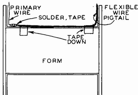
FIG. 2. Attaching the pigtail lead at start of winding. Place flexible lead all the way across form as shown, then wind wire over it, soldering the small wire to the exposed end. Tape and varnish this well. Windings go over this pigtail, thus preventing its pulling out.
