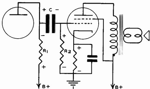
FIG. 6. Voltage drop polarities with a leaky coupling capacitor.
