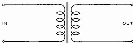
FIG. 3. Schematic representation of isolation transformer. Both primary and secondary have equal number of turns.
