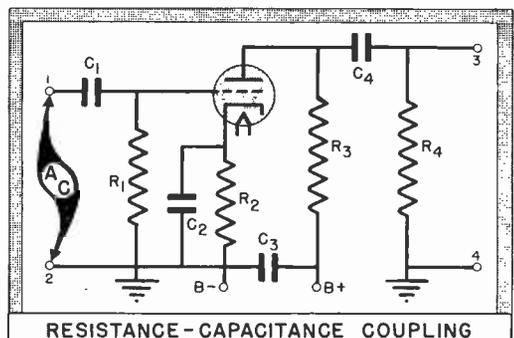
FIG. 1. An R-C coupled audio amplifier stage.
