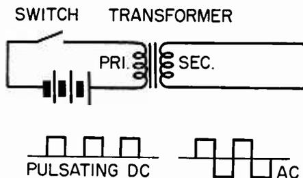
Fig. 10. Using a Switch to give Pulsating DC in a Transformer Winding.
