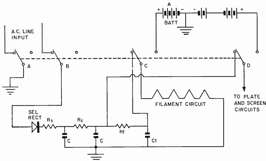
Fig. 9. Typical Portable Radio Power Supply and Power Transfer Switch.
