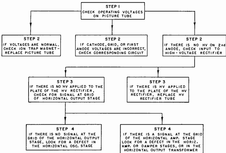
Fig. 8. A Servicing Procedure for use in TV sets where there is no raster.
