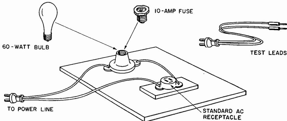
Fig. 3. A Simple Power Transformer Tester You Can Build Yourself.
