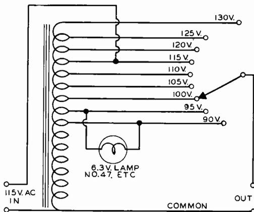
FIG. 4. Schematic of "auto-transformer." This may be used to raise and lower the line voltage as needed for test purposes. Only one winding is used, with taps for the various voltages. Tap switch is shown, so that the output may be adjusted as necessary. The input line goes to the taps marked "Common" and "115-v," if the line voltage is 115 volts.
