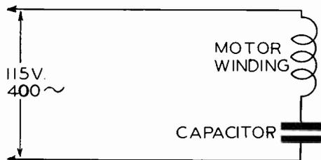
FIG. 3. A motor winding and capacitor in series.
