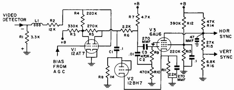
FIG. 2. A typical TV Sync amplifier-separator stage.
