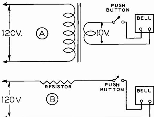
FIG. 2. A doorbell circuit using a step-down transformer and the same circuit using a series resistance.
