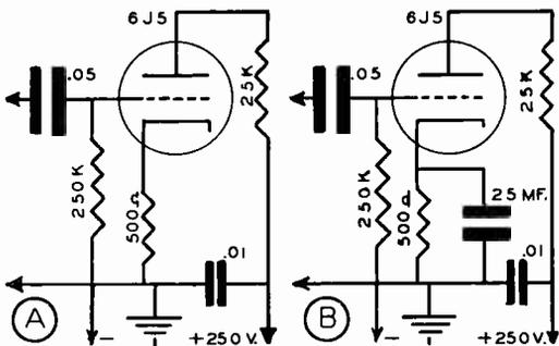
FIG. 5. Typical audio amplifier circuits.
