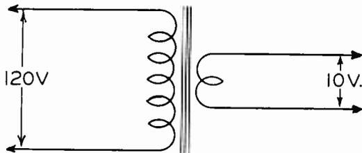
FIG. 1. A step-down transformer diagram showing voltage ratios.
