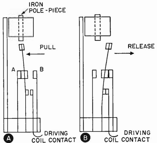
Fig. 12. Pull and Release Positions of a Vibrator Reed.
