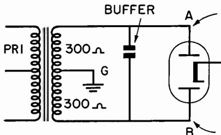
Fig. 14. Resistance of Transformer Secondary and Placement of Buffer Condenser.
