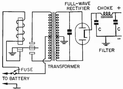
Fig. 13. Complete Vibrator Power Supply.
