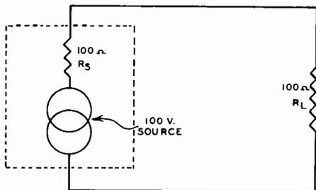
FIG. 4. An ac generator and its internal resistance in series with a load.
