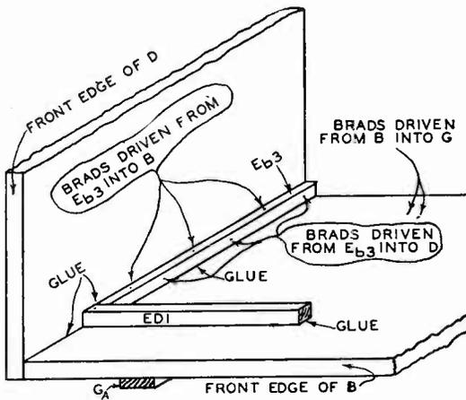
Sketch Fc (Above). Although small nails (brads) are used to reinforce the glued strips, these brads do not show anywhere on the outside of the cabinet.
