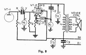
prod to ground. The voltage value should be about 15 volts in a circuit of this kind. (You may refer to the manufacturer's voltage data covering a particular set for exact information.)
