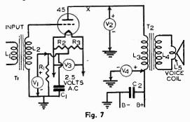
Also, because of power supply overloading caused by the reduction in the bias, voltmeter  $V_4$  would indicate a lower than normal value of tube resistance by indicating excessive loading and, therefore, reduced B supply voltage. Voltmeter  $V_4$  is a d.c. voltmeter connected across the B supply output circuit and condenser  $C_2$ .
