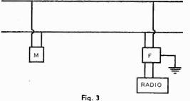
inserted in the receptacle in the filter and the plug of the line noise filter is then inserted in the electric outlet. A ground wire must be attached to the filter. Usually, a ground post is provided on the filter for easy connection of a ground.
