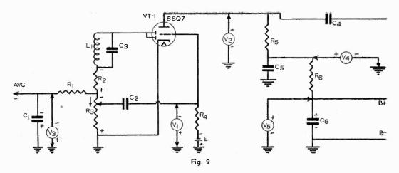
across  $C_5$  if this condenser is leaky. To check,  $C_5$  can be disconnected. If  $V_4$  gives no reading, even on a low range,  $R_6$  is open. (Assuming there is normal voltage across  $C_{6^{\circ}}$ )
