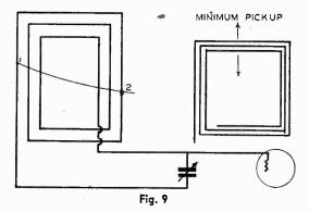
find it necessary and desirable to take advantage of the directional characteristic of the loop to minimize noise pick-up. In many typical General Electric receivers the so-called "Beam-O-Scope" is used and may be adjusted for minimum noise pick-up. This loop is one having an electrostatic shield.
