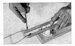
The half-wave open-wire antenna is constructed from two 5' lengths of  $\frac{1}{2}$ " aluminum tubing. Make a smooth right-angle bend at the midpoint of each tube to form the Q-matching transformer.
