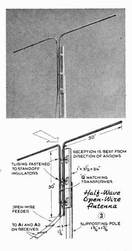
but to link it to the antenna, you will need a simple Q-matching transformer that is nothing more than two vertical legs. The combination is the half-wave antenna, open-wire line, shown in Fig. 3. Bend two aluminum tubes and bolt them to standoff insulators through 3/16" holes drilled in the tube walls. The vertical portions of the tubes must be perfectly parallel, and spaced  $1\frac{1}{4}"$ from center to center. Accuracy of the Q-matching depends on this distance.
