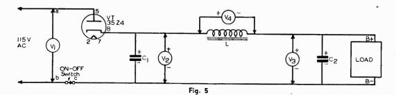
attached to the rear of the volume control. With the switch in the "on" position, approximately 115 volts should be measured by  $V_1$ . Presence of voltage from "a" to "b" and not from "a" to "c" indicates a bad "off-on" switch.
