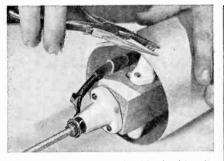
The shield of the coaxial cable should make contact with the aluminum cylinder. A piece of wire inserted between the clamp and the top of the cylinder is recommended.
