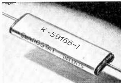
in turn is encased in a metal jacket. The positive contact between wire and bakelite, and in turn with the metal jacket, provides exceptional heat dissipation. The new Series MPT Clarostat fixed resistors measure  $1\frac{1}{2}$ " long by  $\frac{1}{2}$ " wide by  $3/16$ " thick. They are available in resistance values from 10 to 10,000 ohms. The wattage rating is 3 watts. Pigtails facilitate their use in point-to-point wiring.
