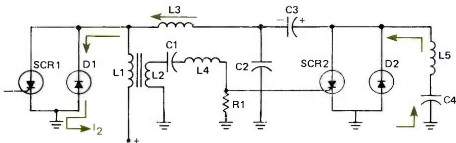
**FIGURE 10. CURRENT FLOW DURING THE INTERVAL T6 TO T7 WHEN D1 IS CONDUCTING.**
