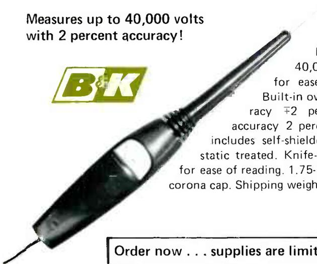
For fast, accurate, and safe high-voltage measurements up to 40,000 volts. Extremely lightweight for ease in handling, yet very rugged. Built-in overload capability. Tracking accuracy  $\pm 2$  percent of full scale. Reading accuracy 2 percent at 25 kv. Meter movement includes self-shielded bar magnet. Housing is anti-static treated. Knife-edge pointer and large numbers for ease of reading. 1.75-inch probe tip for reaching under corona cap. Shipping weight 1½ pounds.
