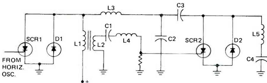
FIGURE 3. SIMPLIFIED SCHEMATIC OF HORIZONTAL SWEEP.
