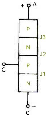
FIGURE 1. THE SCR HAS FOUR SEMICONDUCTOR REGIONS AND THREE JUNCTIONS.
