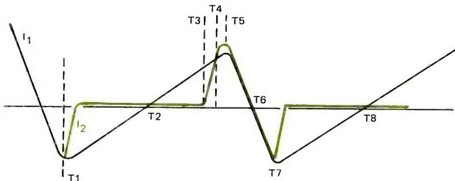
FIGURE 4. THE HORIZONTAL TRACE AND RETRACE CYCLE.
