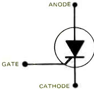
**FIGURE 2. SCHEMATIC SYMBOL OF SILICON CONTROLLED RECTIFIER.**
