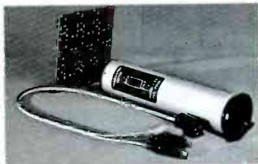
This recently introduced transistor tester can be a real help in locating defective transistors. It places the transistor under test into actual operation without removing it from the circuit. It operates upon contact and emits a clear tone if the transistor is good. No visual observation to make. The absence of a tone indicates a shorted or open transistor. Save time and effort with this low-cost service aid.
