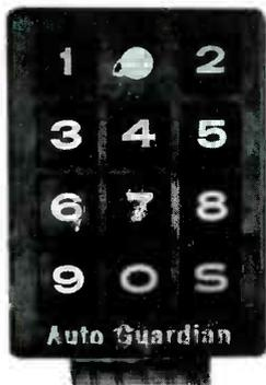
Auto Guardian is a precision solid-state subminiaturized electronic system designed specifically to prevent auto theft. The unique computer keyboard is programmed for a four-digit number combination which is exclusively yours. A light touch of the keyboard for each digit, in the right combination, will immediately allow the ignition system to become operable. It cannot be deactivated at will. For maximum security, it is always on guard. Your car will start only if the correct code is used!
