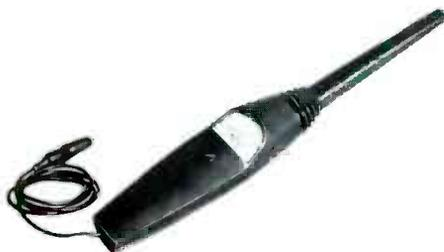
For fast, accurate, safe high-voltage measurements up to 30,000 volts. Extremely lightweight for ease in handling, yet very rugged. Built-in overload capability. Tracking accuracy,  $\pm 2\%$  of full scale. Reading accuracy, 2% at 25 KV. Meter movement includes self-shielded bar magnet. Housing is anti-static treated. Knife-edge pointer and large numbers for ease of reading. 1.75" probe tip for reaching under corona cap. Shpg. wt., 1 1/2 lbs.
