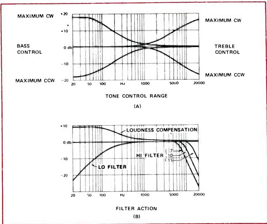
FIGURE 6. GRAPHS SHOWING THE EFFECT OF TONE CONTROLS AND FILTERS ON AMPLIFIER FREQUENCY RESPONSE.
