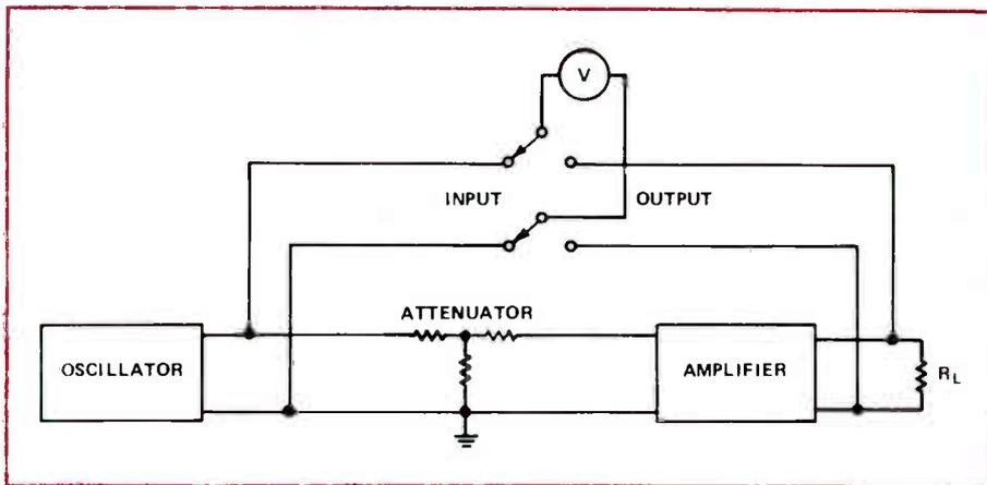
FIGURE 4. METHOD OF MEASURING THE FREQUENCY RESPONSE OF AN AMPLIFIER.
