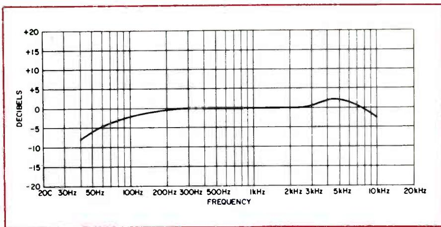
FIGURE 5. AMPLIFIER FREQUENCY RESPONSE.
