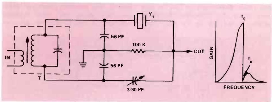
FIGURE 3. CW FILTER AND RESPONSE.
