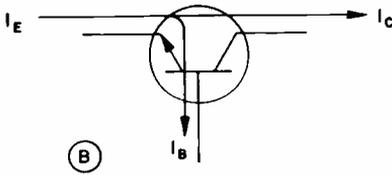
**Fig. 3. Direction of electron flow in an NPN transistor.**
