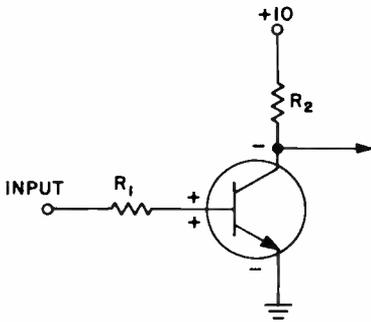
Fig. 10. A transistor switch.
