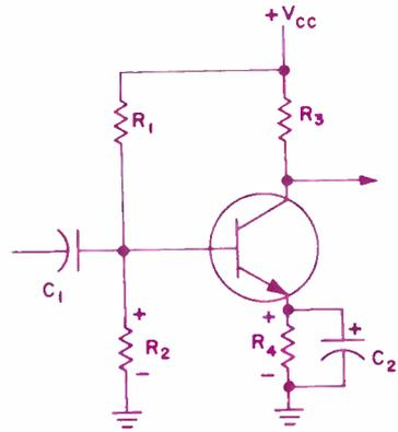
Fig. 8. The preferred transistor bias circuit.
