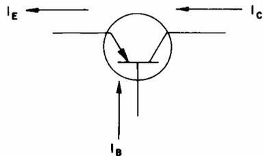
**Fig. 4. Direction of electron flow in a PNP transistor.**
