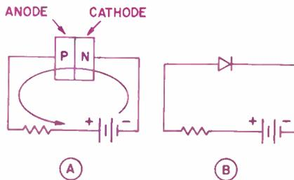
Fig. 1. A forward biased semiconductor diode.
