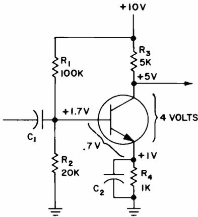
**Fig. 9. A typical amplifier circuit with representative voltage and component values.**
