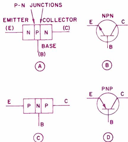
Fig. 2. NPN and PNP transistor symbols.
