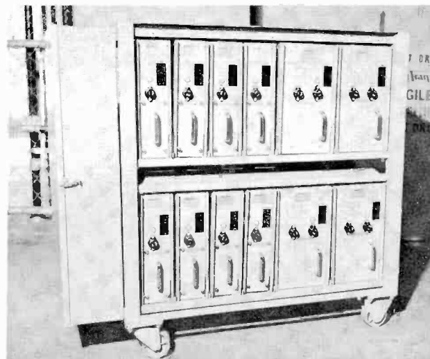
Figure 36: Portable rack on casters with 8-3K and 4-6K plug-in dimmers. Each dimmer can be used as an individual unit, away from rack, with adapter shown in figure 31.
