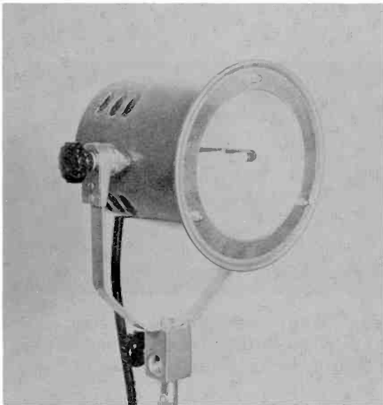
Figure 19: ColorTran Multi-Beam (code LQF-6): A 650-watt Quartz-Iodine variable beam light which produces up to 800 foot-candles at 10 feet.
