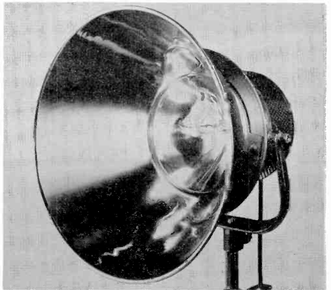
Figure 5: ColorTran Hi-Spot - produces 160 foot-candles at 100 feet used 1-kilowatt Quartz-Iodine Lamp.
