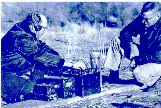
C. MEASURING ANTENNA RESISTANCE.
