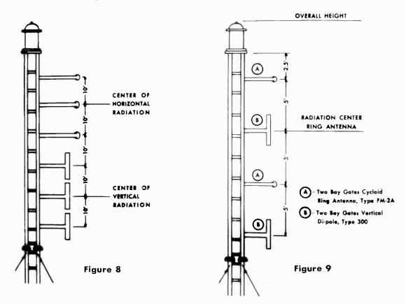
A second method, figure 9, is intermingling of the horizontal and vertical bays. This requires less tower space and places the vertical center of radiation approximately five feet below the horizontal.
