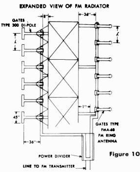
We have not mentioned power dividers. Our discussion has centered around the description of the antenna, installation, and combinations thereof. Normally, we have one transmitter supplying RF to the antenna.
