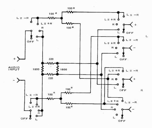
Figure 3. Stereo Test Matrix
