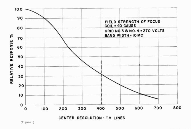
AMPLITUDE RESPONSE STANDARD VIDICON GL7735A FOR UNCOMPENSATED HORIZONTAL SQUARE WAVE
