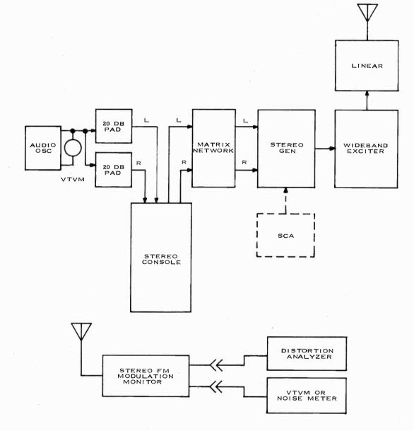
Figure 4. Typical Stereo System and Test Setup
