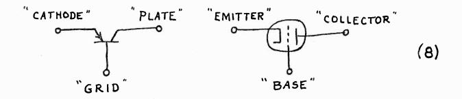
One should not infer, however, that these equivalences are anything but approximate. For example, consider the difference between a grid and a base. A grid, in normal negative-biased operation, draws no current. The total cathode current flows in the plate circuit:
