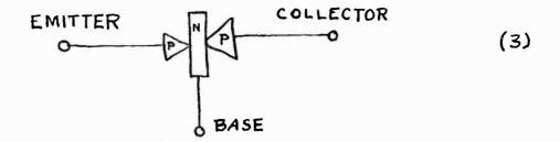
The three elements of the transistor are connected to separate leads, and are labeled <u>emitter</u>, <u>base</u>, and <u>collector</u>, as shown. In a few transistor types of symmetrical design, the emitter and collector have identical properties and may be freely interchanged, but in most transistors the collector junction has a larger area than the emitter junction, leading to differences in electrical characteristics.
