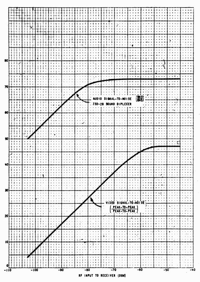
FIGURE ISC - SIGNAL-TO-NOISE RATIO
