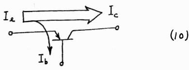
Since the current that flows (for a given voltage) is an indication of the impedance of a circuit, the fact that the base draws current while a grid does not leads to the conclusion that the impedance seen looking into a base would be very much smaller than the impedance seen looking into a grid. The conclusion is correct: a typical vacuum tube, it is well-known, has a grid impedance of several megohms, while a typical transistor may have a base impedance of less than 2,000 ohms.
