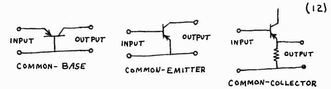
hese three basic configurations are superficially equivalent to the vacuum-tube configurations commonly known as grounded-grid, ground-cathode, and cathode fol-.ower, respectively.
