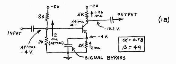
Because of the 2,000-ohm emitter resistance, the d-c resistance looking into the base of the transistor is 102,000 ohms, just as in the case of Figure (15). This high resistance is negligible when shunted across 2,000 ohms, so the current in the voltage divider in the base circuit is nominally equivalent to the supply voltage (-20) divided by the total resistance (10K), or 2 ma. The voltage on
