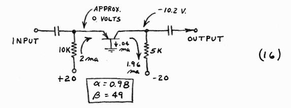
Since the emitter input resistance of only 40 ohms is negligible in series with the 10K bias resistor, the emitter bias current is determined by dividing the bias supply voltage (20) by the resistance (10K), giving 2 ma. If the transistor
