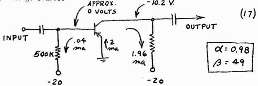
Since the 2,000-ohm input resistance looking into the base of the transistor is negligible in series with the 500K bias resistor, the nominal bias current is determined by dividing the supply voltage (-20V.) by the bias resistance (500K), giving .04 ma in the direction indicated. The collector current is beta times as great, or 1.96 ma, and the collector voltage is determined by subtracting the drop across the load resistor from the supply voltage.
