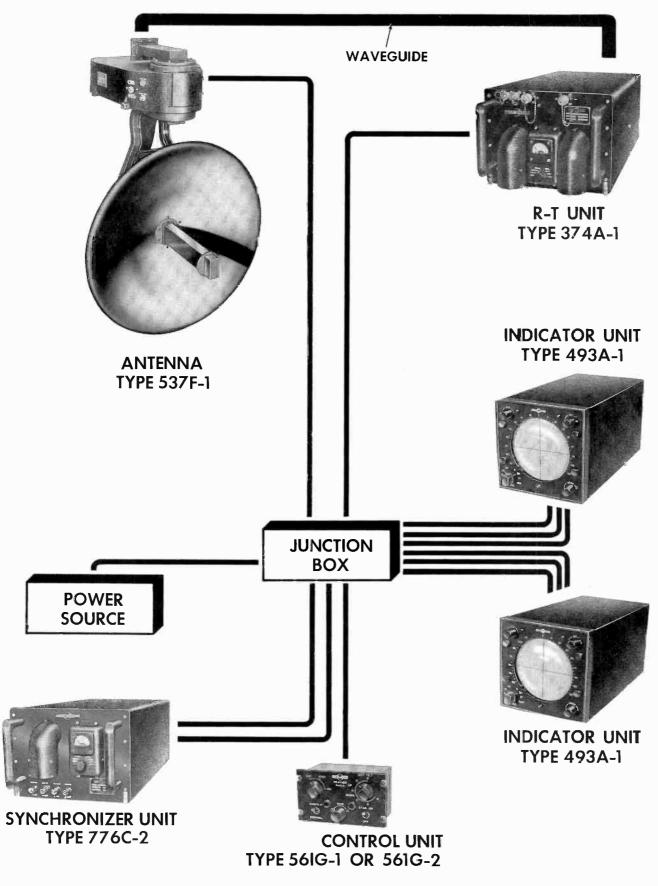
Figure 1. Units of the WP-101 Weather Radar System.
