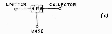
This arrangement is known as an NPN transistor. The major difference between the two types lies in the fact that the various voltages applied to a PNP transistor must be reversed for an NPN transistor.
