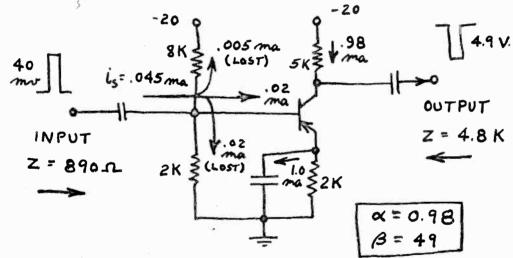
In summary form, the key features of this circuit are: (1) a current gain of about 22, which is less than the beta of the transistor primarily because of the loading effect of the base bias network, (2) a voltage gain of about 122, assuming that the output is not loaded down appreciably by the following stage, (3) a reversal in the polarity of the signal, (4) an input impedance appreciably higher than that of a common-base amplifier, but considerably lower than the 2,000 ohm
