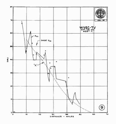
Figure 9 - WVEC-TV field intensities versus distance (reduced to 1 kw radiated) for the 325° bearing.
