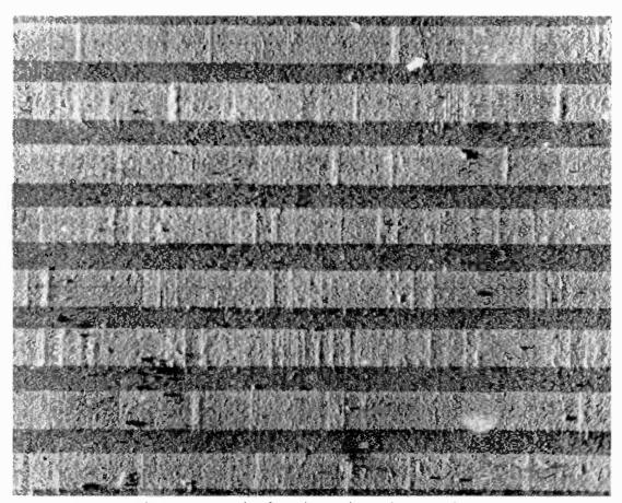
Fig. 9. Photomicrograph of a 1/8 x 3/16 inch area of video tape showing video modulation. (Courtesy of Reeves Soundcraft)
