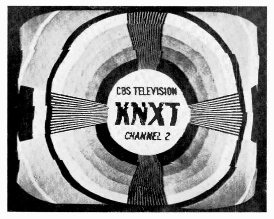
Fig. 6. Picture degradation caused by playing tape back on different head than used for recording.
