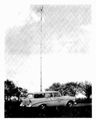
Figure 2 - Mobile unit with mast extended to 30-foot height. A UHF antenna is mounted on the mast.
