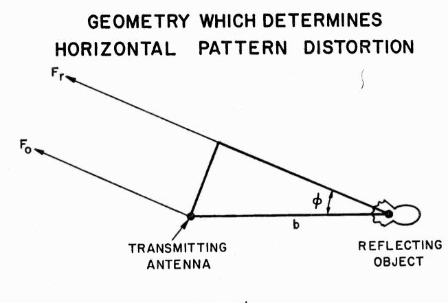
$$\Delta \varphi = 2\pi \frac{(1+\cos\phi)b}{\lambda} + \varphi_r(\phi)$$
