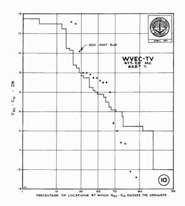
Figure 10 - Distribution of the antenna height-gain function  $E_{30}-E_{10}$  for the measurements of Figure 9.
