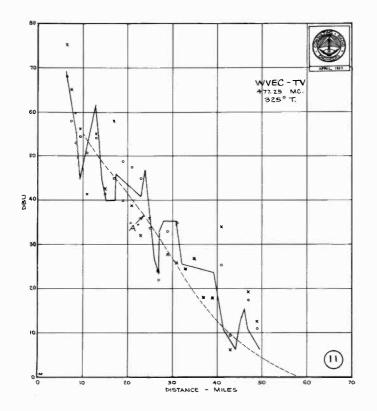
Figure 11 - Continuous 10-foot mobile measurements along the 325° bearing increased by height-gain factors.
