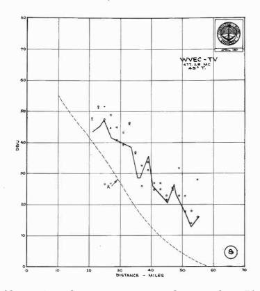
Figure 8 - Effect of applying height-gain factors from Figure 7 to continuous 10-foot mobile recordings. The circles are  $E_{10}$ +6 db, and the crosses are  $E_{10}$  plus individual height-gain factors. The solid line is the long  $E_{30}$  analysis shown in Figure 6.
