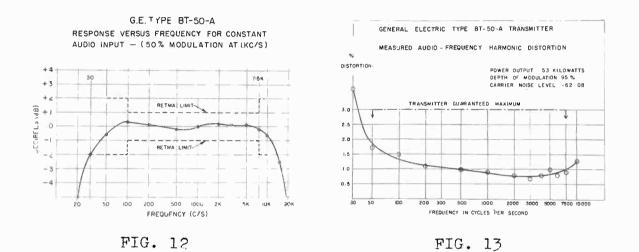
In figure #13 you will note that our feedback system is very effective. This type of performance can be repeated without readjustment following tube changes. There are no critical adjustments to be maintained.
