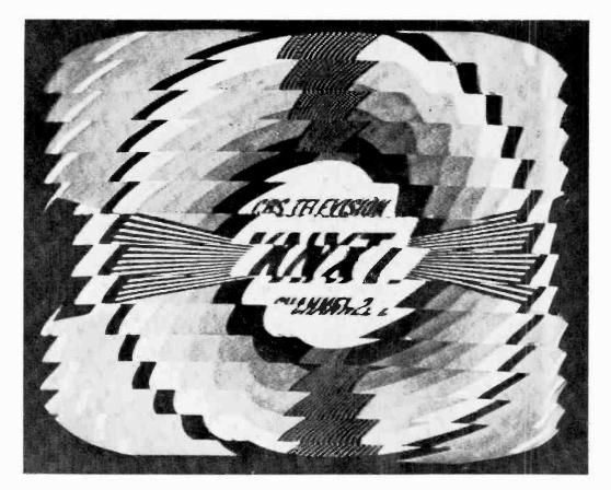
Fig. 5. Picture degradation caused by improper head-to-tape pressure.
