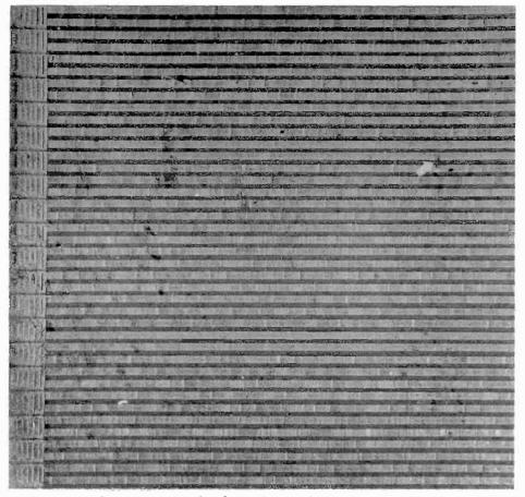
Fig. 8. Photomicrograph of a 5/8 x 11/16 inch area of video tape showing video and control tracks. (Courtesy of Reeves Soundcraft)
