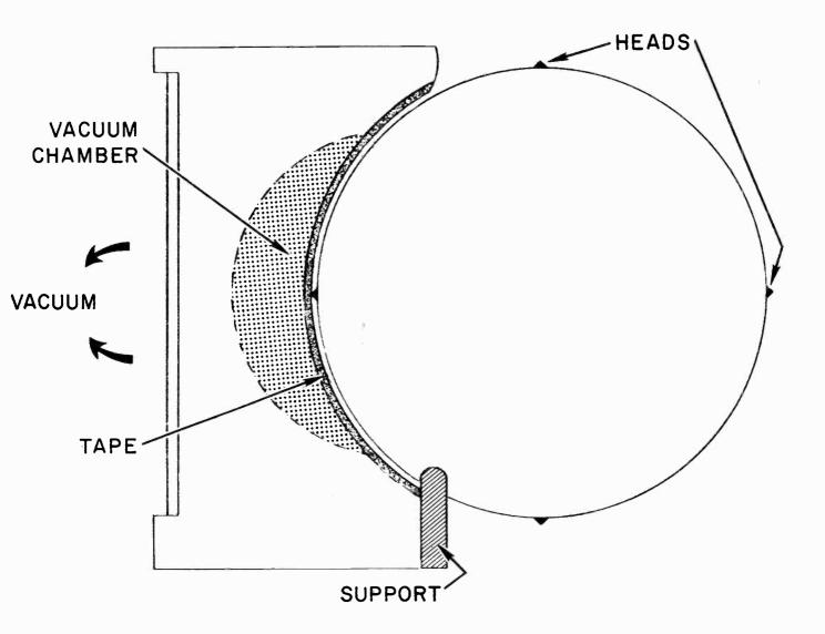
Cross - Sectional Diagram of Rotary Heads & Vacuum Guide
