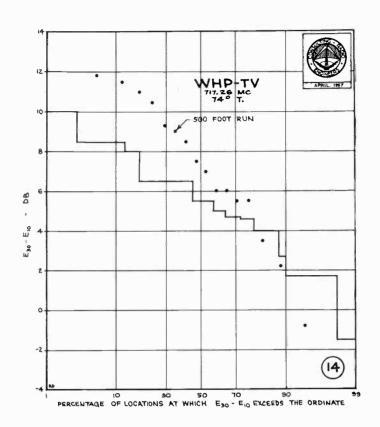
Figure 14 - Distribution of the antenna height-gain function  $\rm E_{30}{}^{-}\rm E_{10}$  for the measurements of Figure 13.
