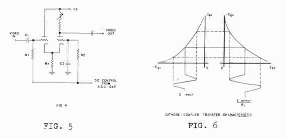
This effect has been substantially reduced in this unit by using a cathode-coupled stage and applying the DC Omin-Control voltage to both grids, as shown in figure 5. The plate currents of both sections are then reduced to lower the gain. Signal currents are 180 degrees out-of-phase, and curvature of the  $E_g - I_p$  characteristics tend to cancel, as shown in figure 6. The operation is similar to a push-pull stage.
