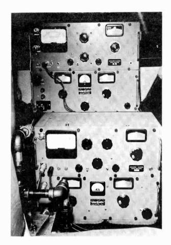
Figure 3 - Interior of mobile unit showing field intensity meters.
