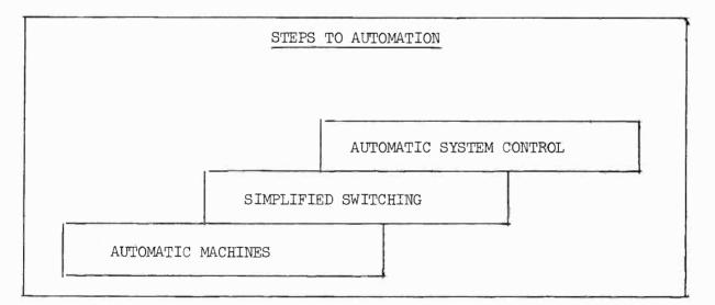
to build toward automatic programming by first taking the step of obtaining individual basic equipments that are automatic or in some instances modifying existing equipments to make them automatic. Second, take further advantage of the automatic machines by simplifying the manual control to ease the human operating problem. Third, based on the foundation of the first two steps add automatic system control and achieve the goal of automatic programming through system evolution.
