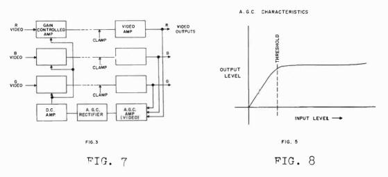
To increase the compression ratio, that is the glatness of the inputoutput curve, the rectifier is followed by a DC amplifier to increase the AGC loop gain. The input-output characteristic is shown in figure 8.
