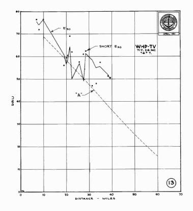
Figure 13 - Plot of 30-foot mobile measurements on WHP-TV on 717.26 mc reduced to 1 kw along a bearing of 74° True. The line marked "A" is from FCC Report 2.4.16.
