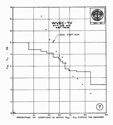
Figure 7 - Distribution of the antenna height-gain function  $E_{30}-E_{10}$  for the measurements of Figure 6.
