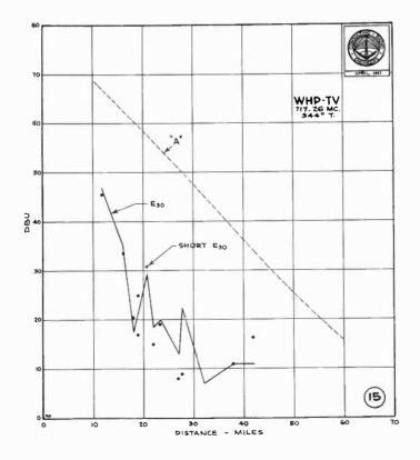
Figure 15 - Plot of 30-foot mobile measurements on WHP-TV on 717.26 mc reduced to 1 kw along a bearing of 344° True. The line marked "A" is from FCC Report 2.4.16. This is in very rugged terrain.
