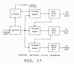
The Keying-Generator is shown in figure 13. There is but one timing multivibrator in the entire circuit, which is the three-to-one divider. It is extremely stable and requires no adjustment.
