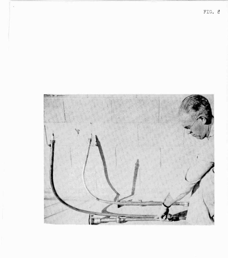
The matching harness is made from Andrew type S-450 7/8" co-ax. This line is available from the factory with dipole end terminals, using gas tight construction. The junction box ends of these lines may be cut and soldered on the job, depending on local measurements.
