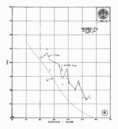
Figure 6 - Field intensity versus distance for WVEC-TV, Hampton, Virginia, on 477.25 mc (reduced to a radiated power of 1 kw) in the direction 45° True. The solid line joins the median field intensities for the long measuring sectors. The circles are the median field intensities for the first 500 feet of each mobile run. The line marked "A" is the median field intensity given by the Commission's TRR Report 2.4.16.
