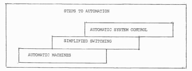
three logical, progressive steps to automatic programming are first, automatic machines; second, simplified switching; and third, automatic system control.
