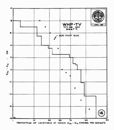
Figure 16 - Distribution of the antenna height-gain function  $E_{30}-E_{10}$  for the measurements of Figure 15.
