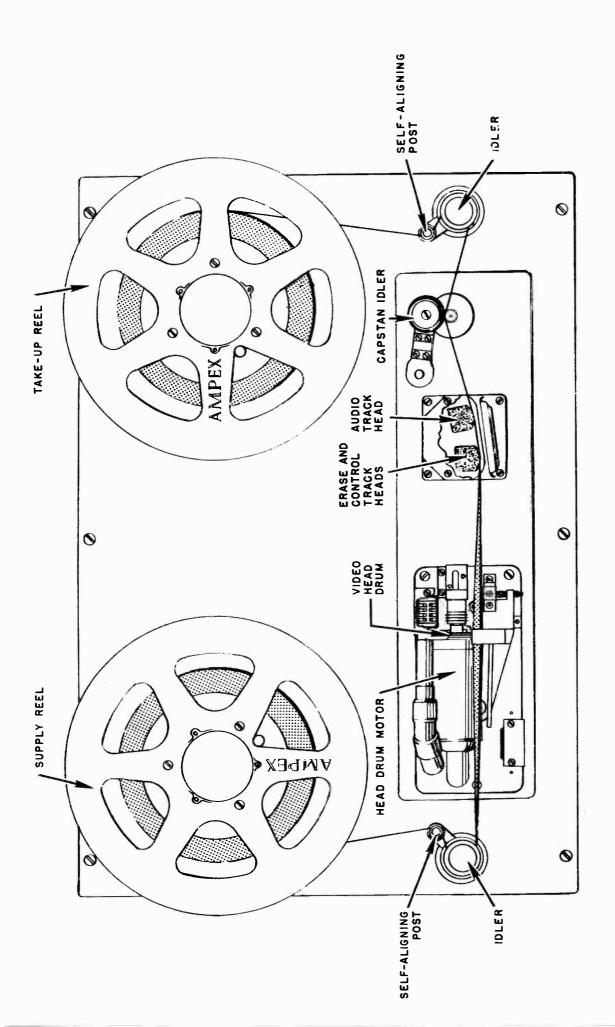
Layout of Video Tape Recorder Transport Mechanism.
