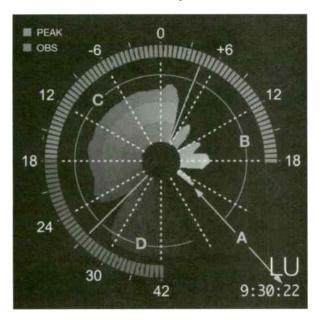
Fig 8. Loudness Meter explained. "Radar head", A, is moving clockwise, one revolution (e.g.) per minute. The outer ring shows current loudness at around -12 VU.
