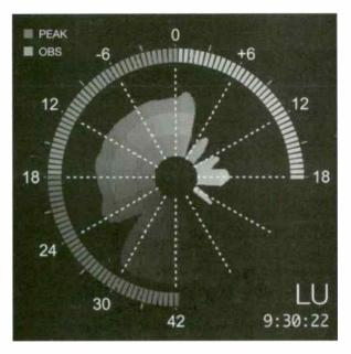
Fig 7. Loudness meter with fourness history in the "radar view" and color coded in accordance with the HDTV targets of Fig 2.
