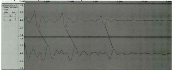
Figure 2: Off-air captured sample, in split mode (left is digital, right analog), with three possible points of comparison, all with different offsets at the sample level.
