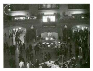
*Fig 9.* Loudness meter superimposed onto a TV picture. The outer ring shows short-term loudness, the arrow shows long-term loudness. For both indicators, 12 o' clock represents Reference loudness. The red center indicator would normally be off. It signifies notable channel differences, and electrical low or high level.
