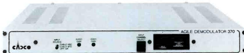
The CADCO Model 370T is a precision agile Demodulator used to demodulate any NTSC audio/video signal to baseband audio and video signals for use in Demod/Remod configurations:
