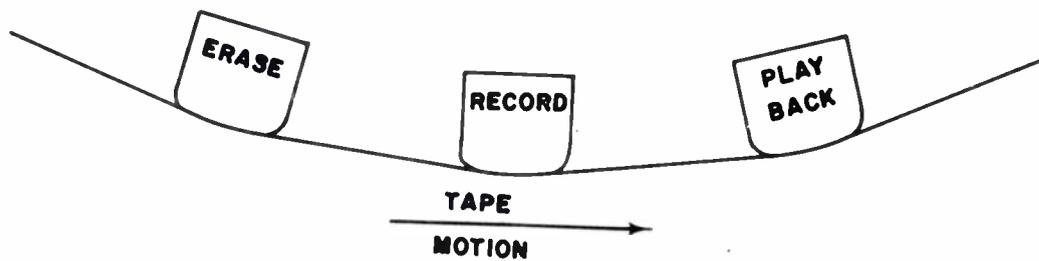
Fig. 1. Normal head arrangement.
