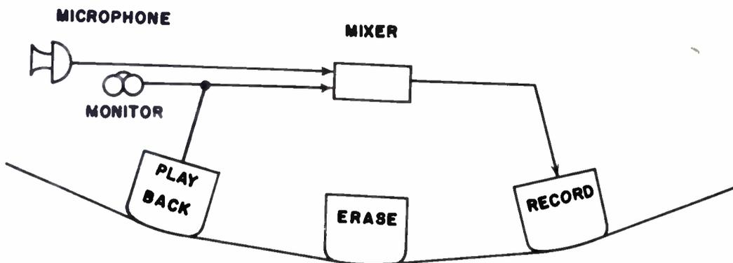
Fig. 2. Modified head arrangement for sound-on-sound recording.
