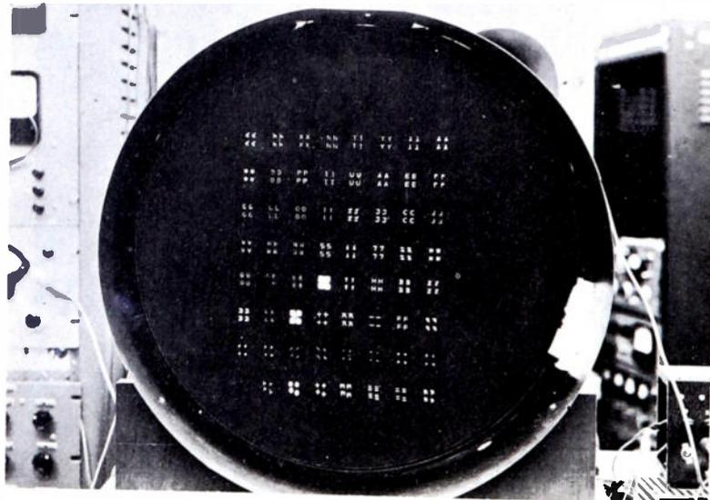
Fig. 14. Stored characters on 21-inch Typotron tube.
