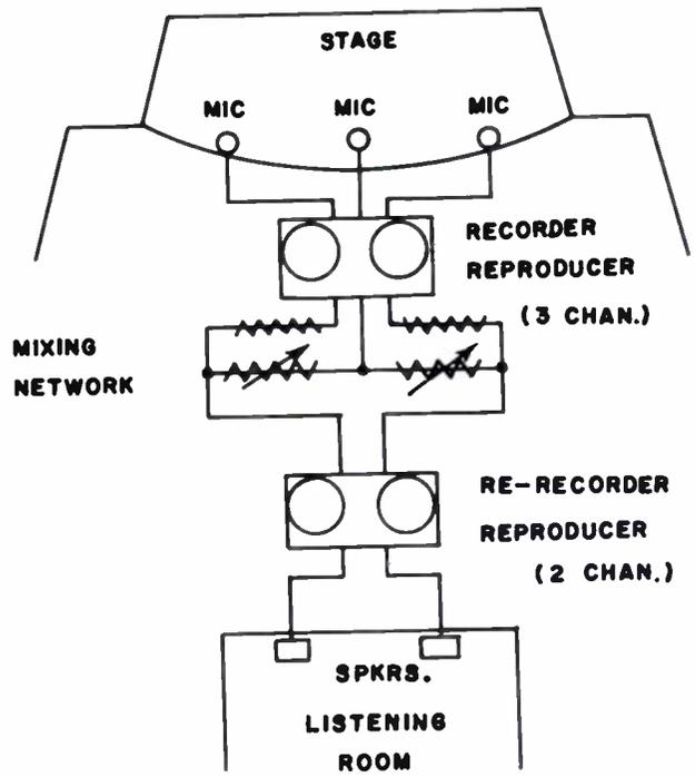
Fig. 4. Method of using three-channel recorder for two track stereo releases.
