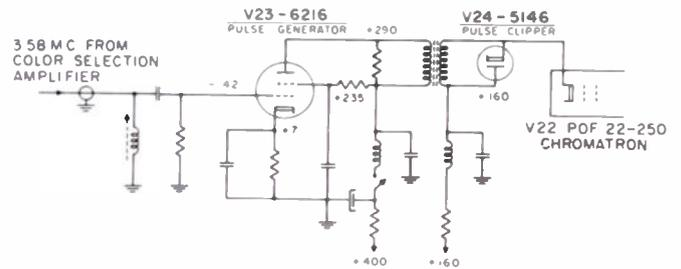
Fig. 6. Schematic anti-blue pulser.
