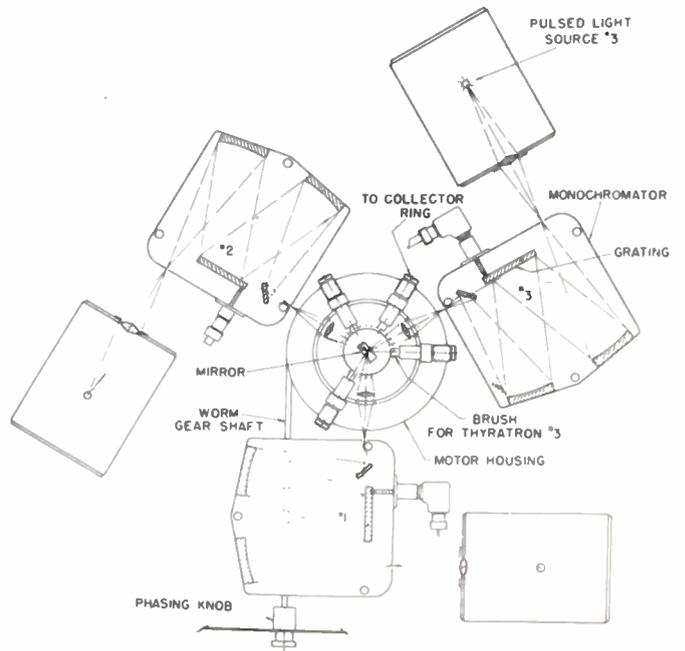
Fig. 5 Diagram of Illuminating System.
