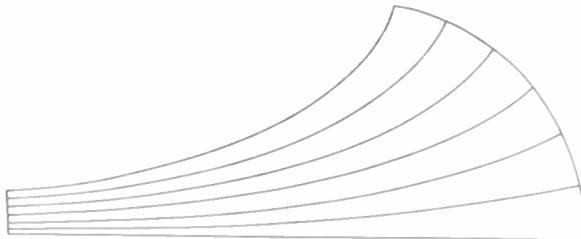
Fig. 4. Revised version of horns, with all horns terminating normally to spherical surface.
