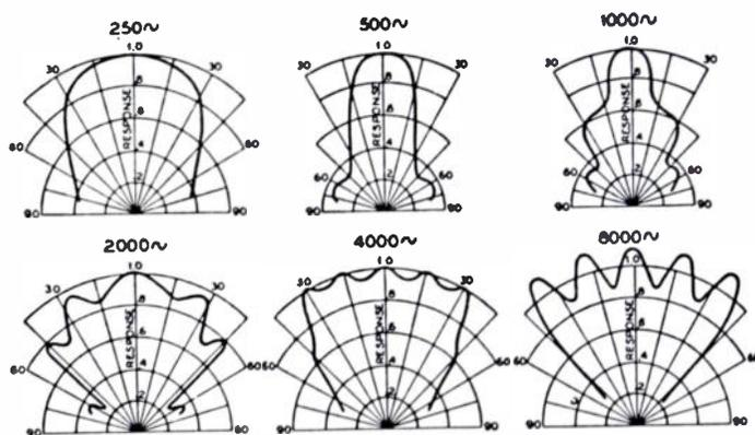
Fig. 2. Directional characteristics of the 15-cell horn shown in Fig. 1 in a plane containing the line A-A and the axis of the center horn. The sound pressure for the angle 0 degrees is arbitrarily chosen.
