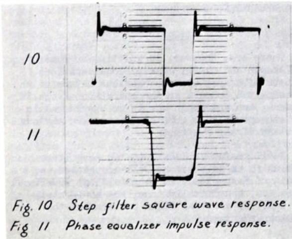
Fig. 10 Step filter square wave response.
