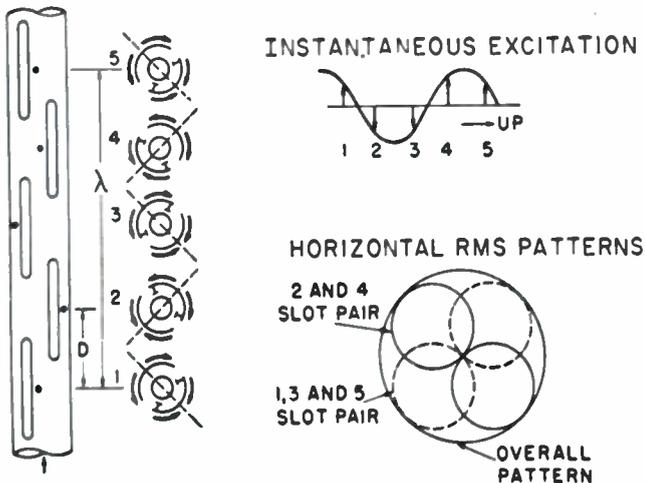
Fig. 7—Excitation and horizontal pattern formation of traveling-wave antenna.
