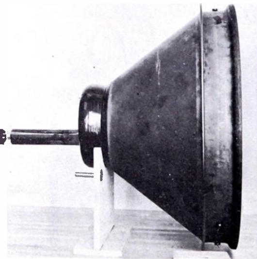
Fig. 9. 21-inch Tonotron tube.
