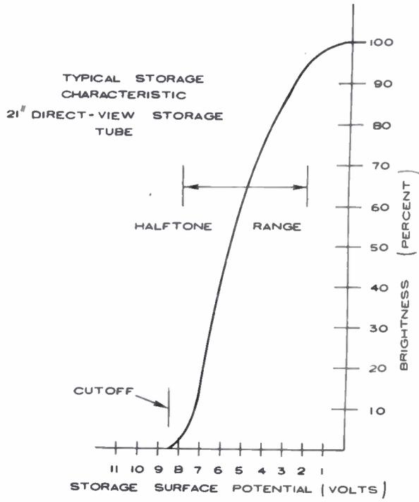
Fig. 2. Typical storage characteristics.
