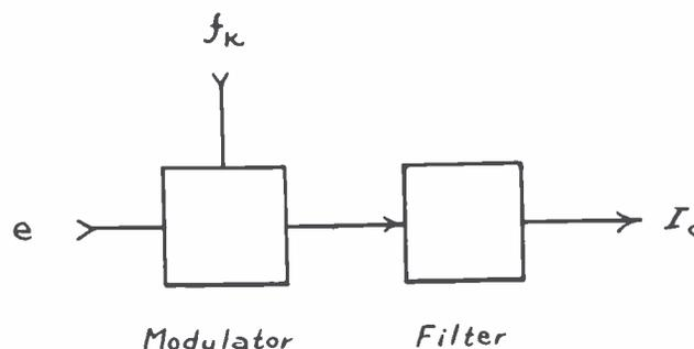
Fig. 1. Block diagram of product detector.
