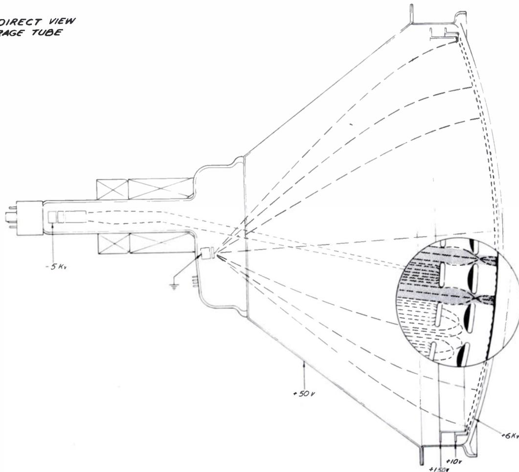
Fig. 1. Schematic of the 21-inch Tonotron tube.
