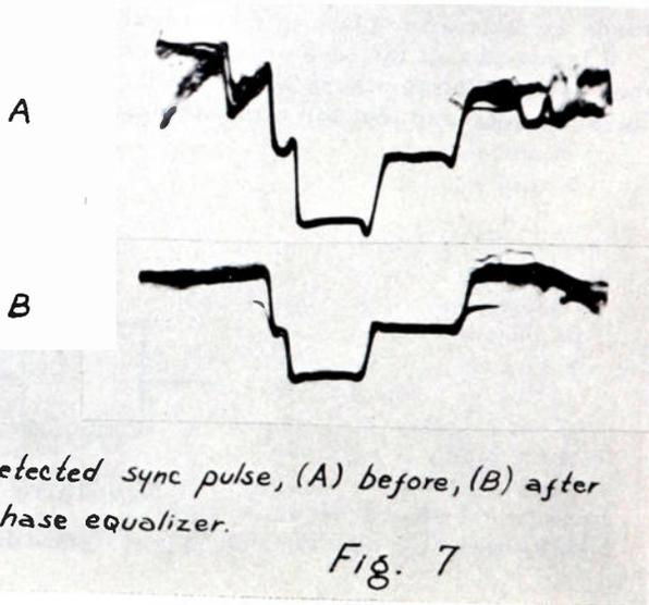
Detected sync pulse, (A) before, (B) after phase equalizer.
