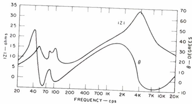
IZI  $\angle \theta$  OF AN 8-ohm 12" COAXIAL SPEAKER IN A BASS REFLEX CABINET
