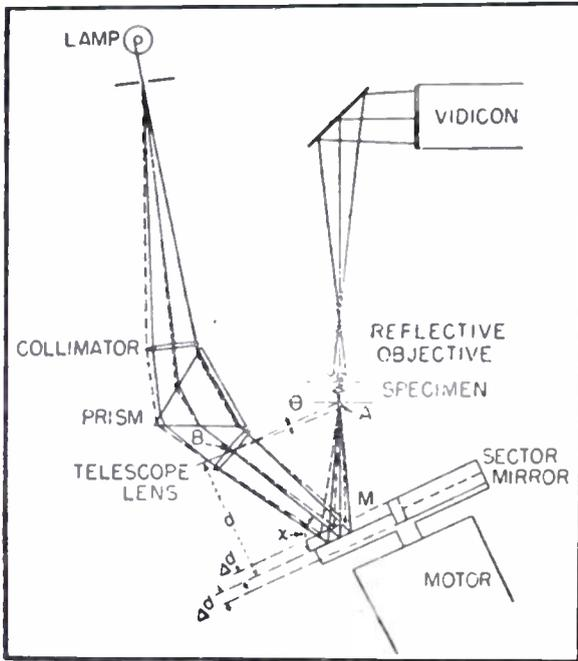
Fig. 2 Wavelength Selection in Single-Source Color Translating Microscope.
