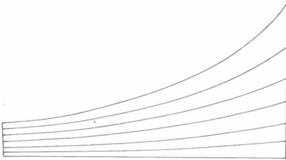
Fig. 3. Half cross section of early version of horns, showing plane surface at mouth.
