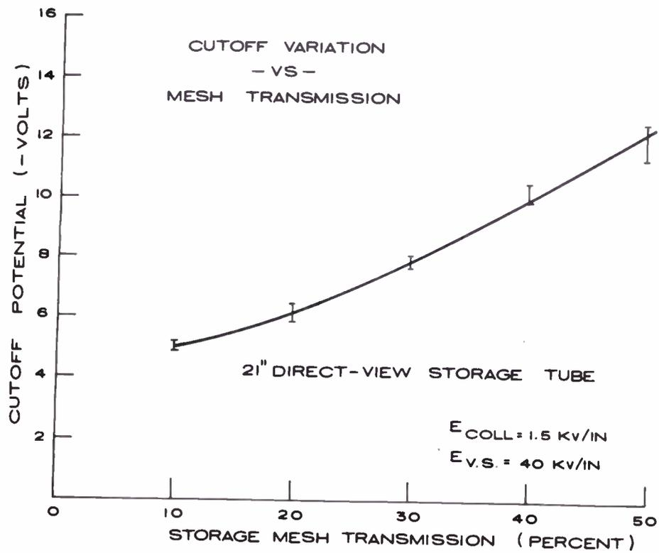
Fig. 8. Cutoff variation with storage mesh transmission.
