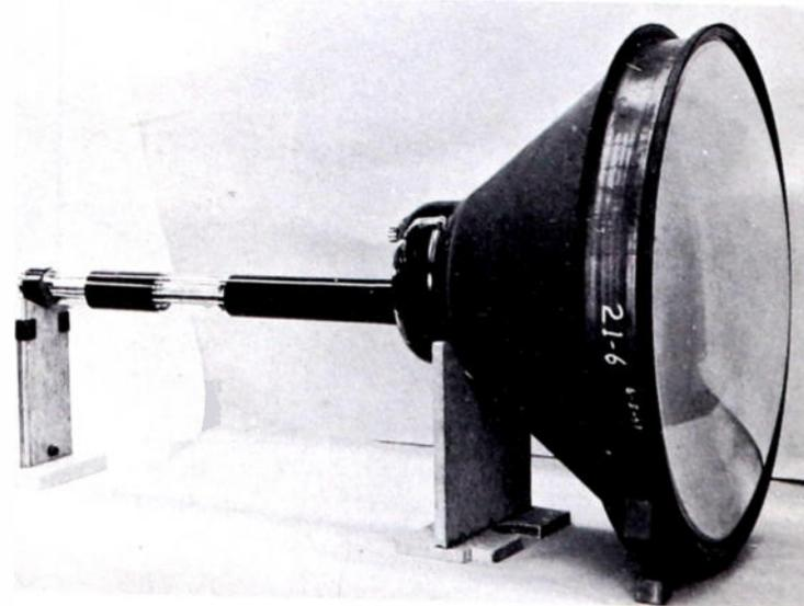
Fig. 10. 21-inch Typotron tube.
