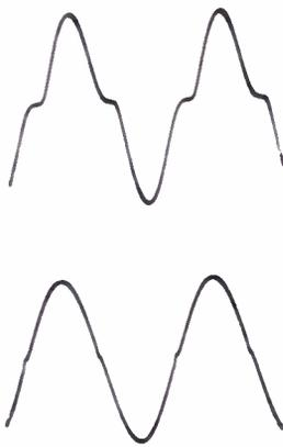
Fig. 2 Collector current waveforms
