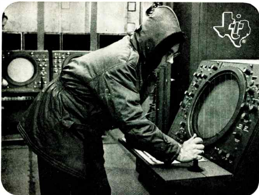
Environmental testing of TARMac ASR-4 Airport Surveillance Radar System, developed and produced for the Federal Aviation Agency.
