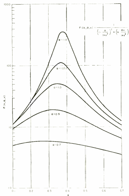
Fig. 3—Regenerative gain of straight-through amplifier as a function of the normalized idler frequency and of the stability parameter \alpha for k = 0.4 , where k denotes the normalized input susceptance.
