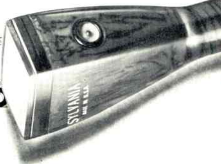
Sylvania 3BGP1, 3BGP2, 3BGP7, 3BGP11 . . . feature direct-view rectangular faces, electrostatic deflection and focus, high deflection sensitivity.
