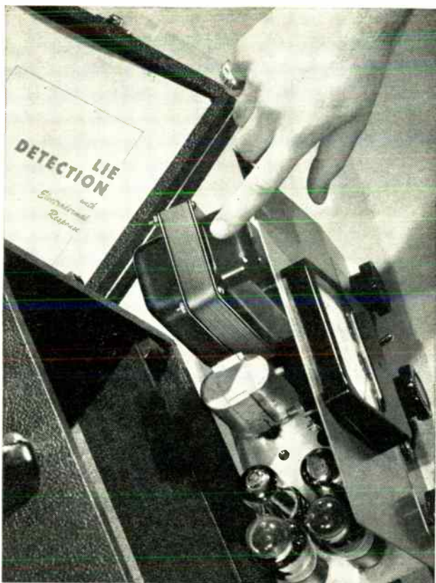
Above—Sola plate-filament transformer is built-in component of B & W Associates lie detector. It supplies plate and filament voltage regulated within \pm 3\% even when line voltage varies from 100 to 130 volts . . . helps assure accurate operation in field.
