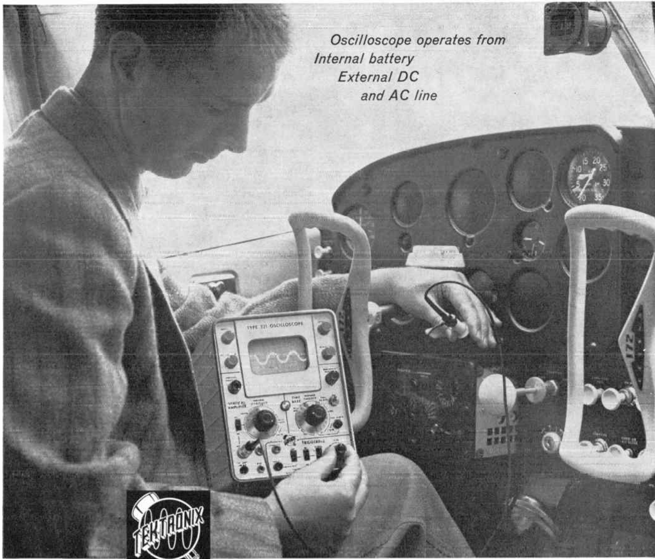
Using a Type 321 to check the omni-directional navigation aid feature of an aircraft transceiver.
