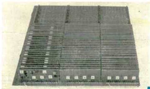
Plug-in module, shown mounted on matrix panel utilizing Elco Varicon contacts.
