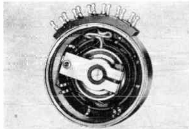
2" Ball-Bearing Precision Potentiometer
