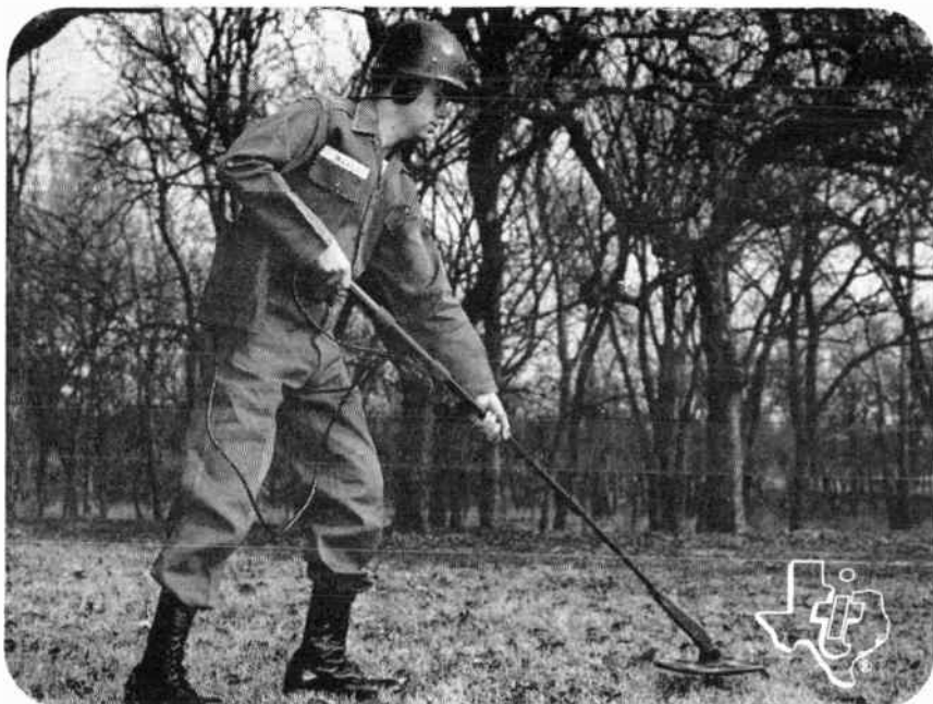
19 Anti-personnel Mine Detector AN/PRS-3 (XR-12) designed and built for the Corps of Engineers by Texas Instruments.
