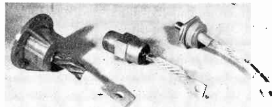
Fig. 2—Large power silicon rectifier units.
