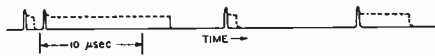
Fig. 3—Simultaneous oscillograph tracings of diode current and output of microwave receiver. The dotted curve is the current and shows a slight initial overshoot. The overshoot as well as the observed rise and fall times are characteristic of the measuring circuit. The solid curve is the 9-kmc receiver output. In every case the pulse rise results in a pip from the receiver.
