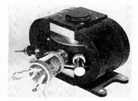
Fig. 17-Industrial model of an "M" Carcinotron.
