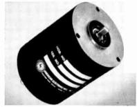
The motor operates on 400 cps. It is excited with 115 v on the fixed phase and 24 v on the control phase. Torque at stall is 2.9 inch/ounces with a power factor at stall torque of 50 per cent. No load speed is 5,100 rpm. Temperature range:  $-55^{\circ}$ C to 90°C. Weight is 13.7 ounces. Additional data is available from the manufacturer.
