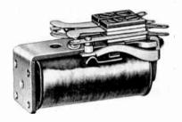
Friction-creating hinge pins are eliminated, and the use of a beryllium copper armature retaining spring insures positive contact between armature and pivot point at all times.
