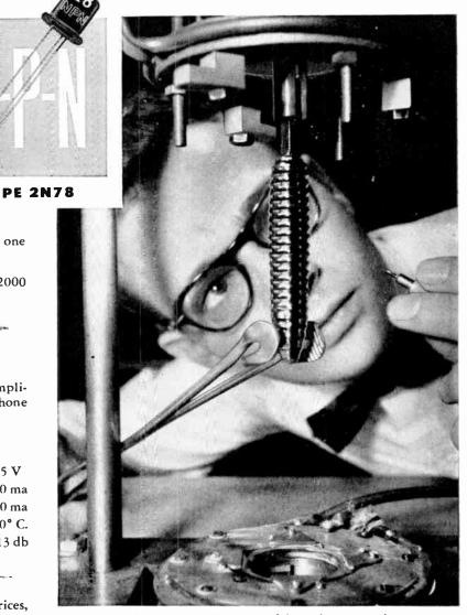
Billet of germanium is removed from furnace, prior to cutting into enough tiny pellets for 2000 transistors.
