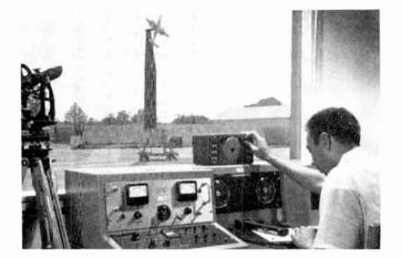
Electronics Research Engineer Irving Alne records radiation antenna patterns. Twenty-two foot plastic tower in background eliminates ground reflections, approximates free space. Tower is of Lockheed design, as are pattern integrator, high gain amplifier, square root amplifier, logarithmic amplifier.
