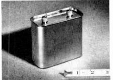
STANDARD COMMERCIAL For motors, filters, communication equipment, luminous-tube transformers, industrial control. Rolings dual rated units (a-c or d-c) rated at 0.01-50 uf, at 236-660 v. a-c, 400-1500 v. d-c. Single rated units also available. Tolerance  $\pm 10\%$ . Temp. range -55 to  $+85^{\circ}$  C. BULLETIN GEC-809.
