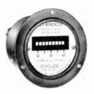
"Standco" panel frequency meters are made in 3 styles of cases, molded bakelite case, metal case and hermetically sealed case. They come with 5, 7, 9, 11, 21, 36 or 41 reeds for normal frequencies of 25, 50, 60 and 400 cps. Other ranges from 15–1500 cps can be supplied. Accuracy of calibration  $\pm 0.5$  per cent. Request bulleting 805 from the manufacturer.
