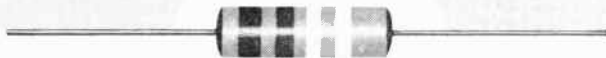
WIRE WOUND —molded Bakelite shell. 3 sizes, 0.47 to 10 \Omega , 1/3 to 1 watt, to 11 volts. Standard tolerance \pm 5 and 10%.
