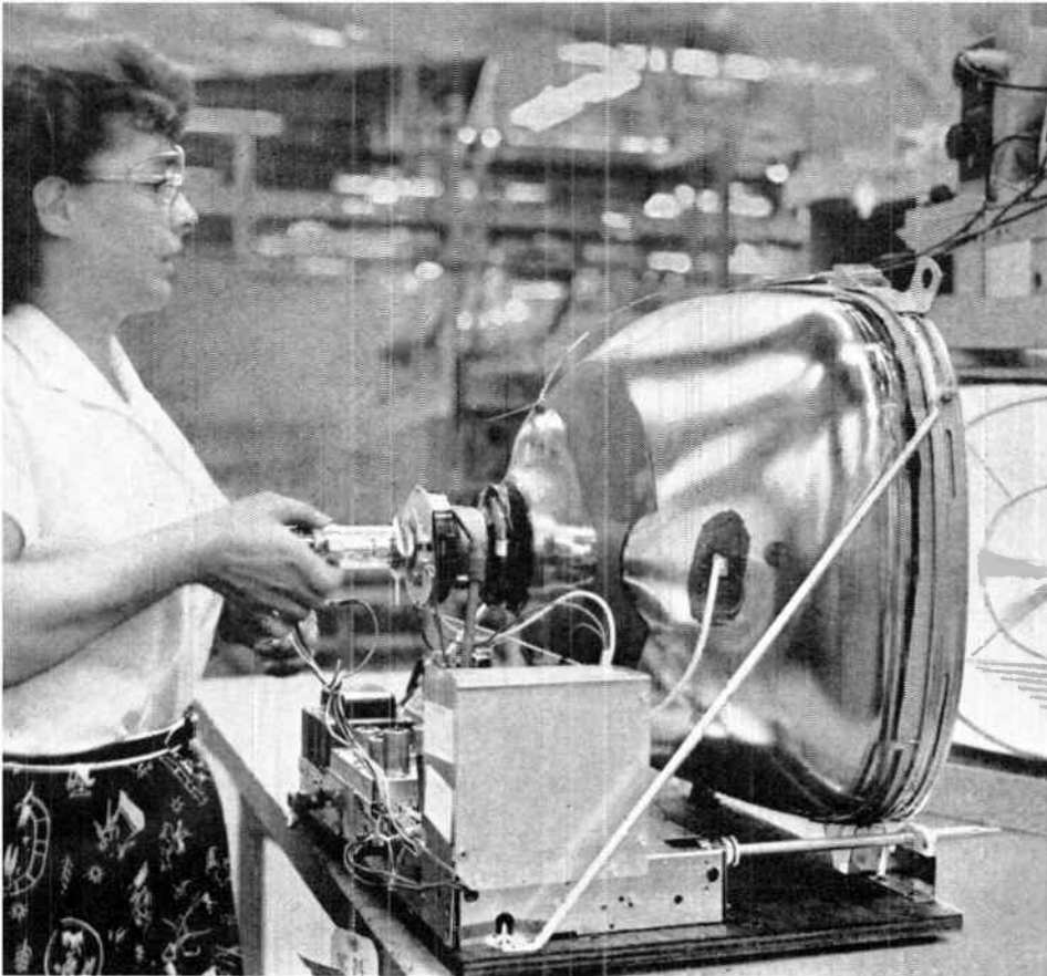
You can cross this operator (ion-trap magnet adjustment) off your list of production processes, with General Electric straight-gun picture tubes. Cost of magnet is a further saving.
