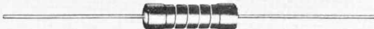
NOBLETTE —Axial Leads - Metal Film, Vitreous-Clad. 4 sizes, 1 \Omega to 10 Meg \Omega 1/2 to 2 watts, to 750 V. Standard tolerance \pm 1 .
