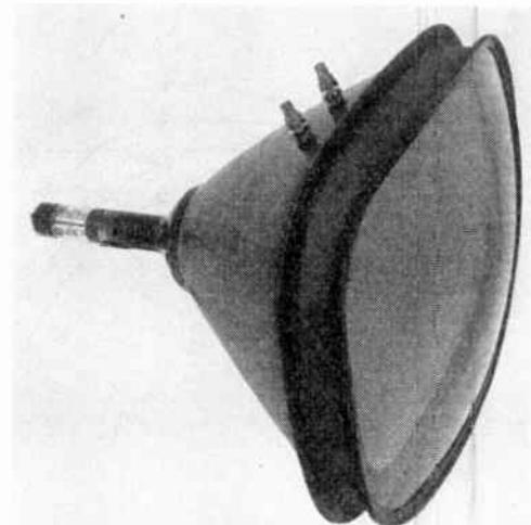
Fig. 8—Photograph of completed 24 inch metal rectangular tube.
