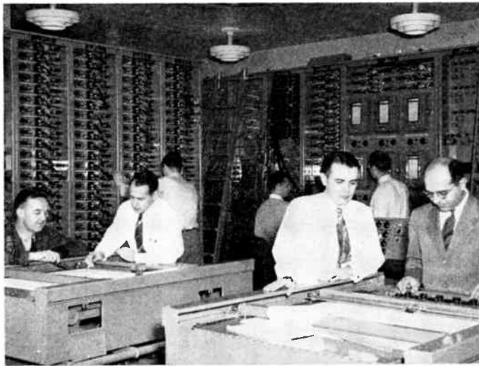
Fig. 8—The Typhoon Computer, developed and built by the RCA Laboratories Division of the Radio Corporation of America, in operation at the Naval Air Development Center at Johnsville, Pennsylvania. The Typhoon has extreme flexibility of design, and has been adapted to unusual uses.
