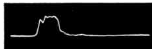
Pulse through Model 202P Wide Band Chain Amplifier and Model 214 Chain Pulse Amplifier (50 db gain). Note reproduction of fine detail.
