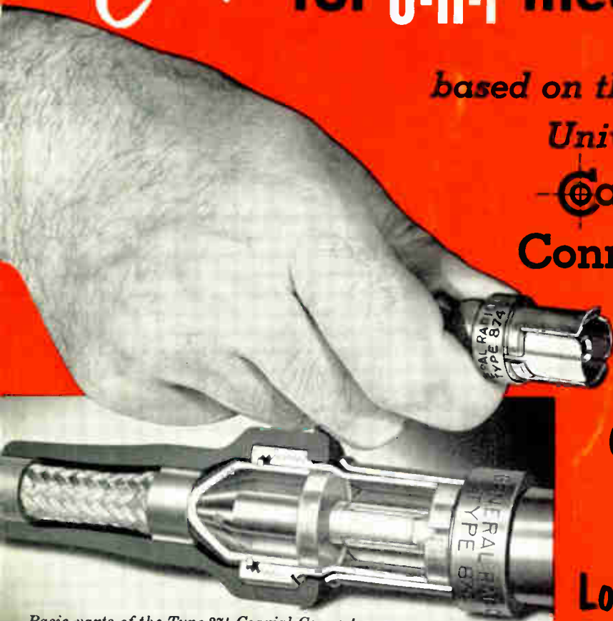
Basic parts of the Type 874 Coaxial Connector: inner conductor, outer conductor and supporting polystyrene bead. The overlapping portion of the connection is a uniform coaxial section.
