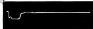
0.06 \mu sec complex pulse applied directly to oscilloscope plates. Rise time approx. 0.001 \mu sec.
