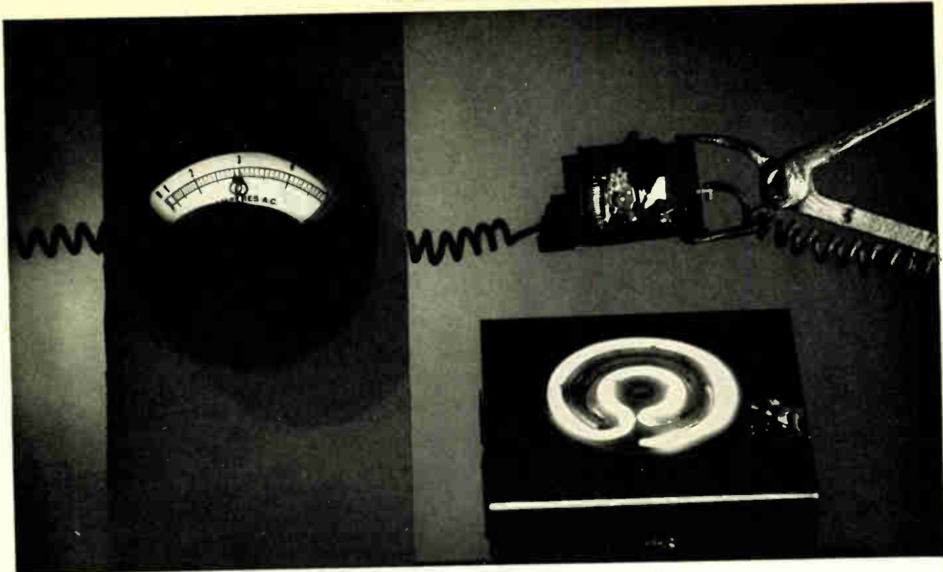
Laboratory demonstration shows 30 amperes continuously flowing through 30 ampere Heinemann Circuit Breaker held over hot plate.
