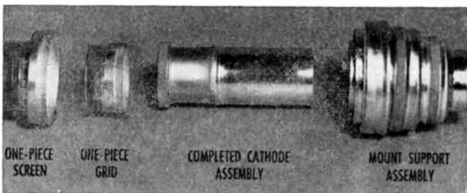
Fig. 5—Screen grid, control grid, cathode assembly, and mount support assembly.
