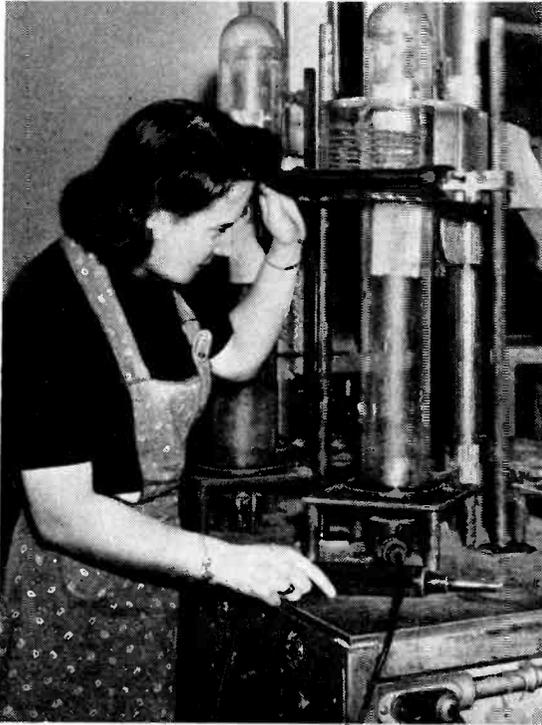
Fig. 5—Induction-heated vacuum firing station.
