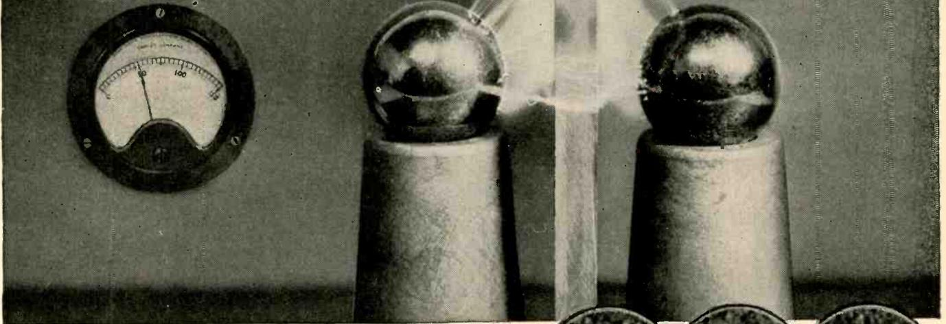
This high frequency insulation will not carbonize under arc, yet it possesses dielectric properties of the highest order. Made entirely of inorganic materials, Mykroy cannot char or turn to carbon even when exposed to continuous arcs and flashovers.
