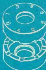
"TH" Type Powder is employed for cup shields in cores.
