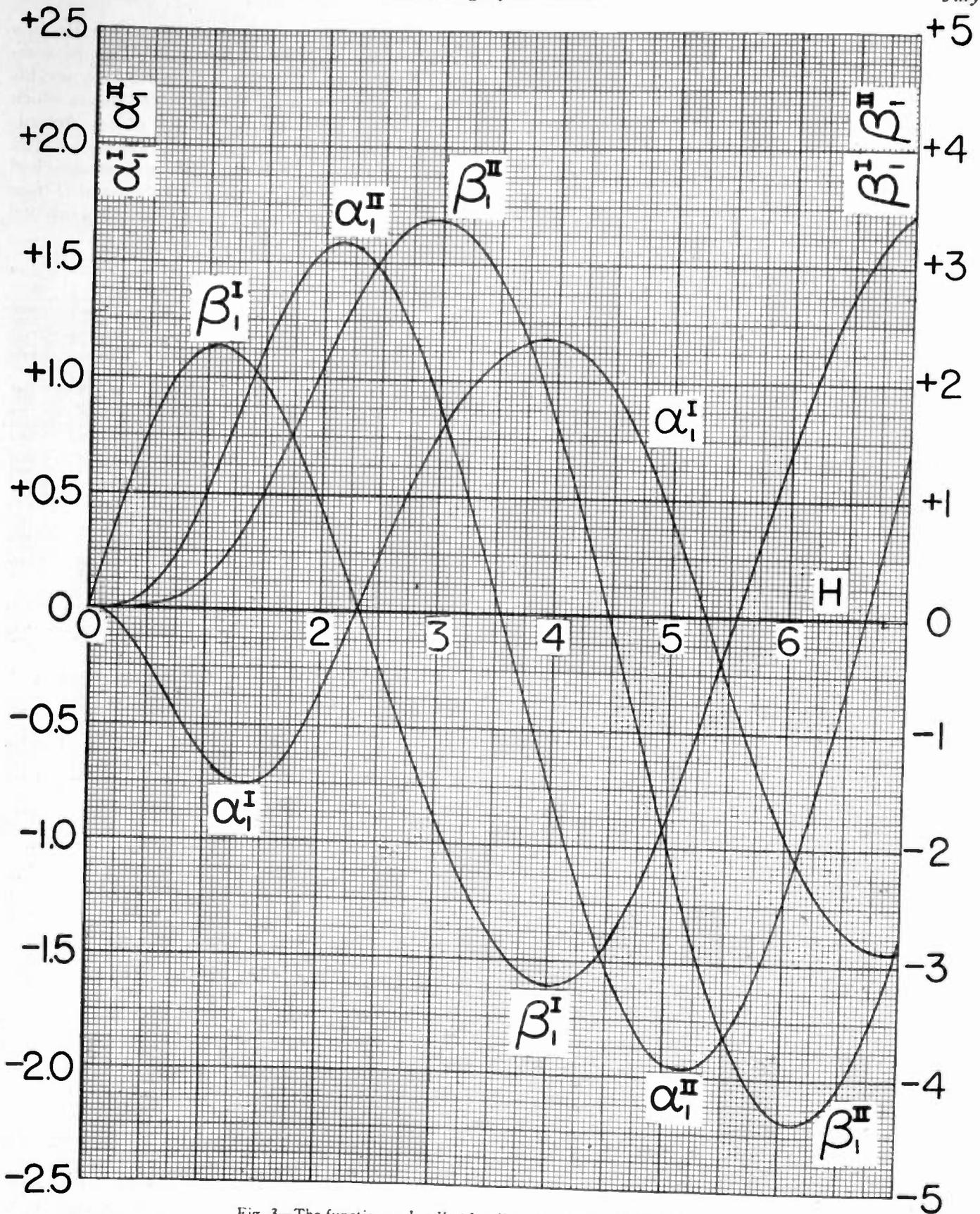
Fig. 3—The functions  $\alpha_1^I$ ,  $\alpha_1^{II}$ ,  $\beta_1^I$ ,  $\beta_1^{II}$  as functions of  $H = 2\pi h/\lambda$ .
