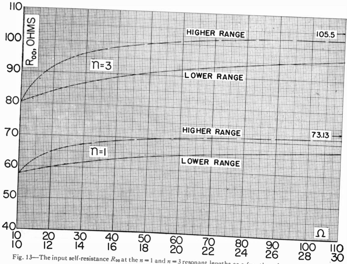
Fig. 13—The input self-resistance  $R_{00}$  at the  $n = 1$  and  $n = 3$  resonant lengths as a function of  $\Omega = 2 \log(2h/a)$ .
