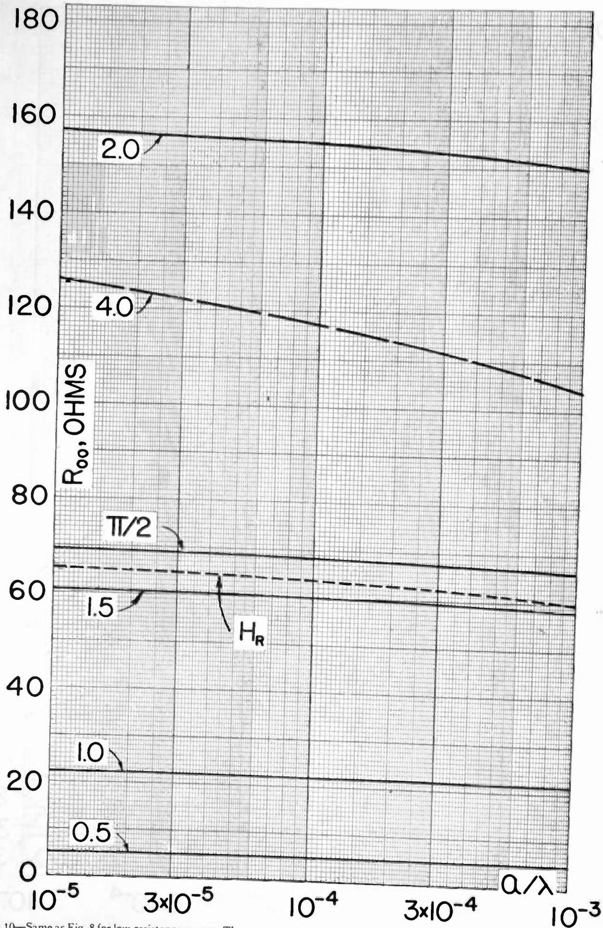
Fig. 10—Same as Fig. 8 for low-resistance ranges. The curve marked  $H_r$  is for values of  $R_{00}$  when  $H$  is adjusted to resonance near  $H = \pi/2$  for indicated values of  $a/\lambda$ .
