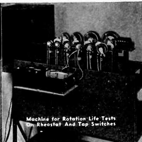
Machine for Rotation Life Tests on Rheostat and Tap Switches
