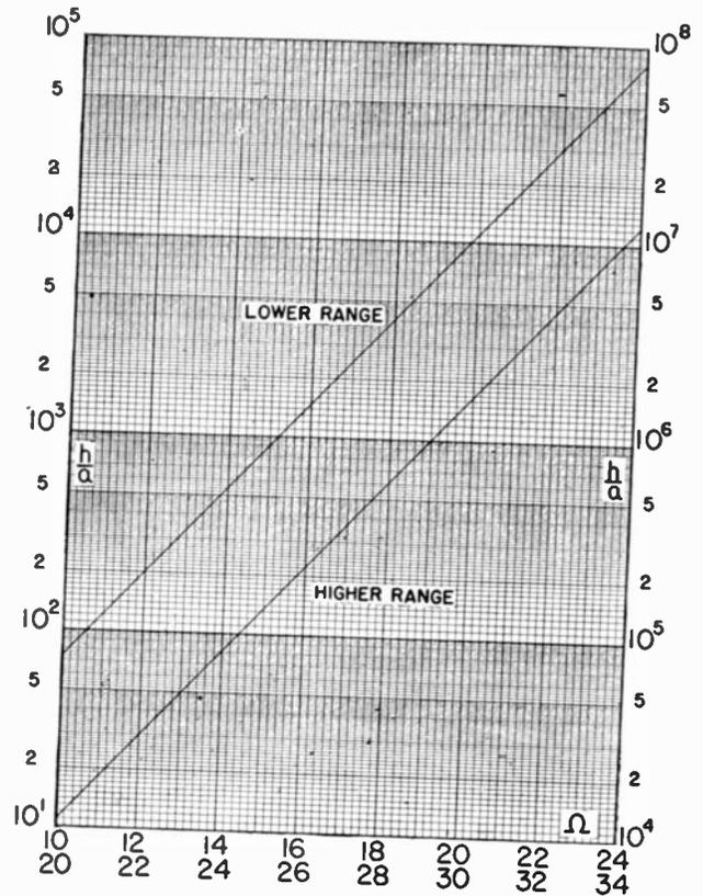
Fig. 1—The parameter  $\Omega = 2 \log (2h/a)$  expressed in terms of  $h/a$ .
