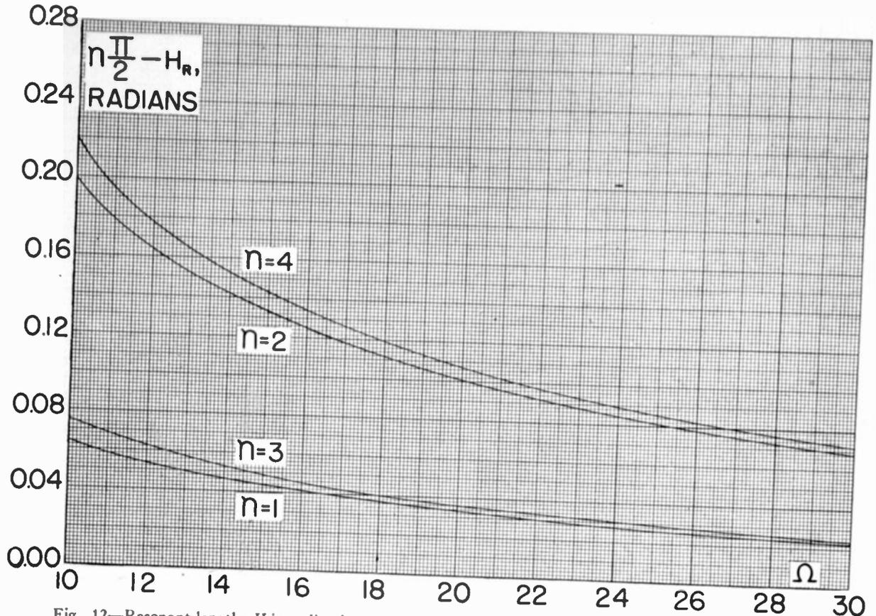
Fig. 12—Resonant lengths  $H$  in radius for zero radius minus resonant lengths in radians for nonvanishing radius; viz.,  $n\pi/2 - H_r = 2\pi(n/4 - h_r/\lambda)$ , as functions of  $\Omega = 2 \log(2h/a)$  for  $n = 1, 2, 3, 4$ .
