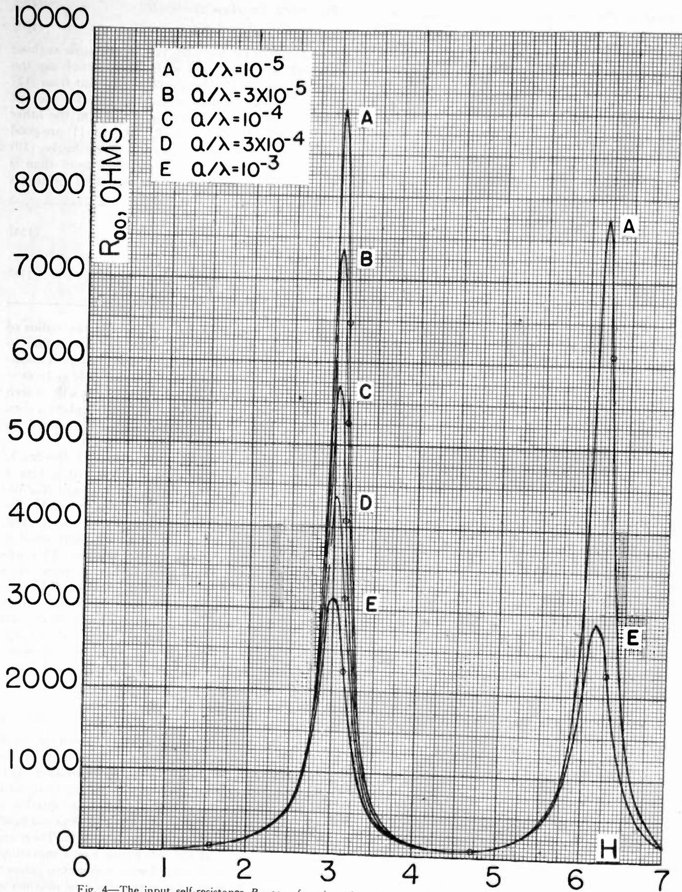
Fig. 4—The input self-resistance  $R_{00}$  as a function of  $H=2\pi h/\lambda$  with  $a/\lambda$  as parameter. Values at  $H=n\pi/2$  are indicated by a small circle.
