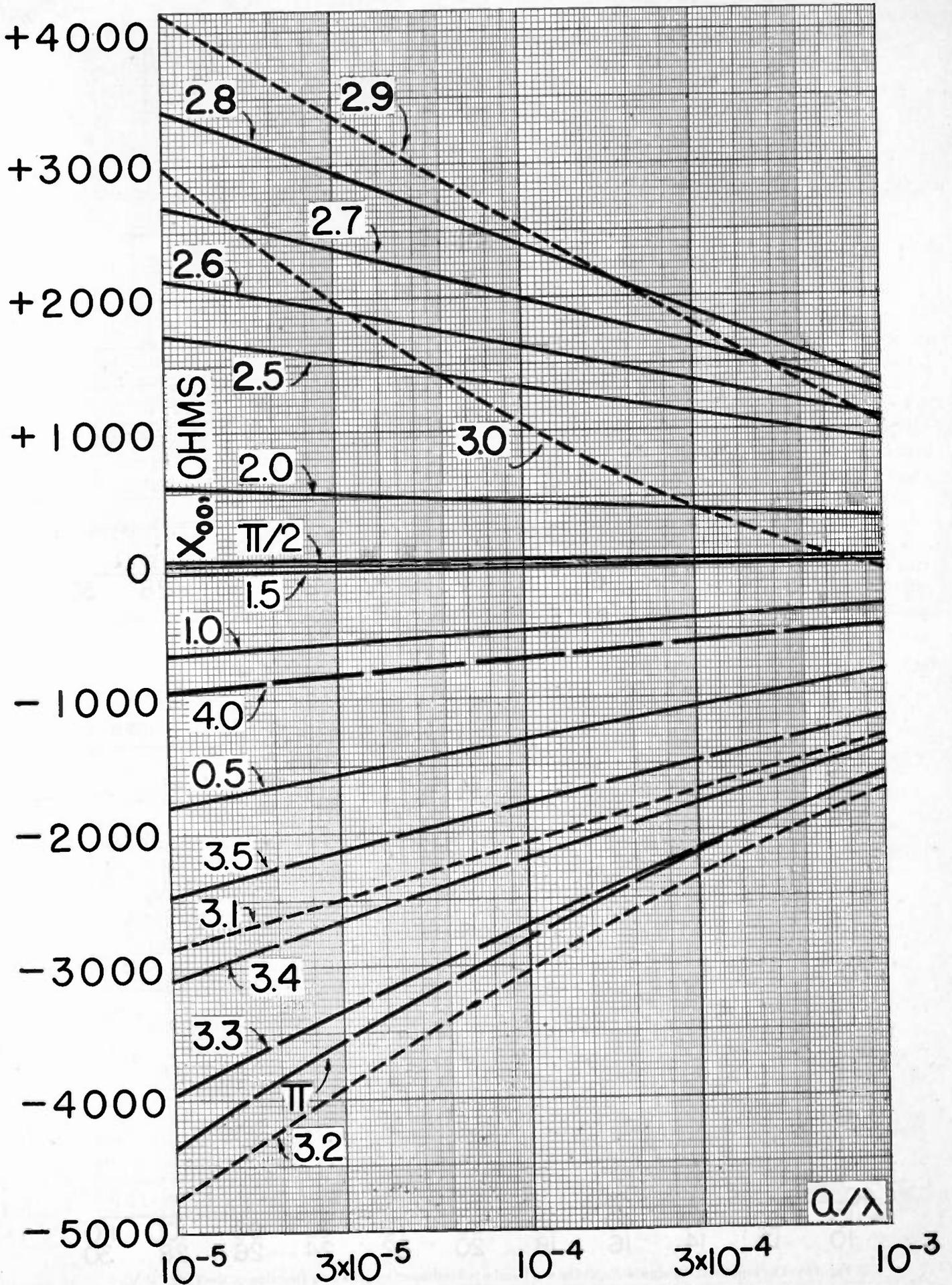
Fig. 11—The input self-reactance  $X_{00}$  as a function of  $a/\lambda$  with  $H=2\pi h/\lambda$  as parameter.
