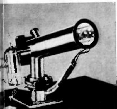
**ELECTRON MICROSCOPE** virtually gives a moving picture projection of the action of electrons being emitted from a heated filament. Such observations enable Eimac engineers to constantly produce better filaments.
