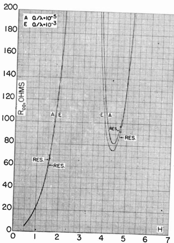
Fig. 7—Same as Fig. 3 for low-resistance ranges. Resonant points are denoted by an arrow.
