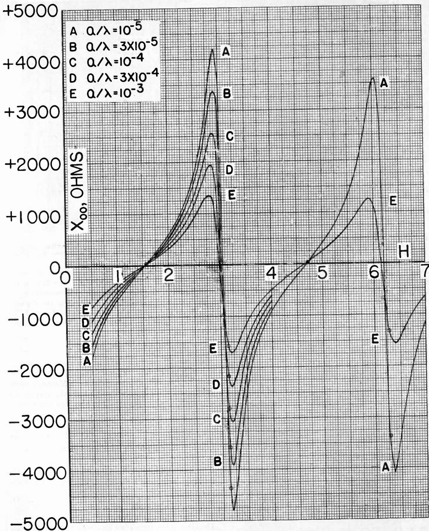
Fig. 5—The input self-reactance  $X_{00}$  as a function of  $H = 2\pi h/\lambda$  with  $a/\lambda$  as parameter. Values at  $H = n\pi/2$  are indicated by a small circle.
