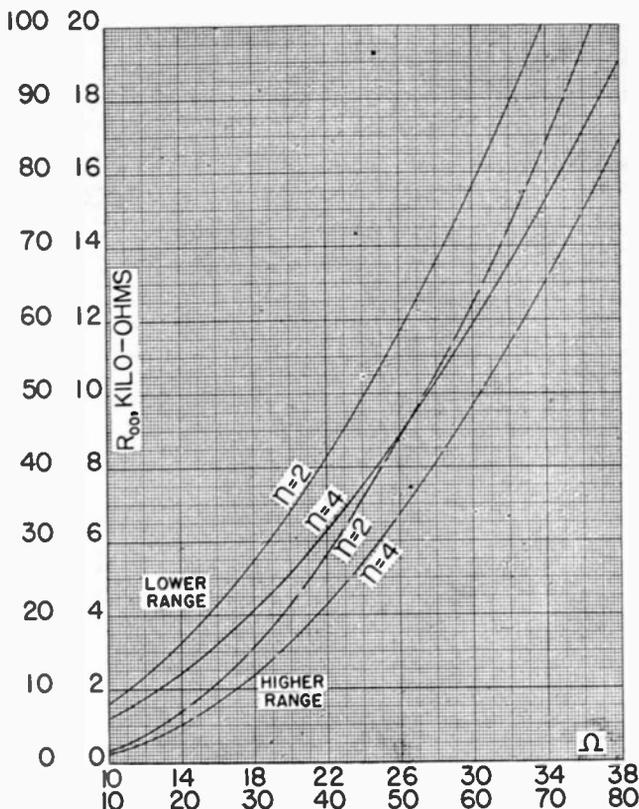
Fig. 14—The input self-resistance  $R_{00}$  at the  $n=2$  and  $n=4$  anti-resonant lengths as functions of  $\Omega = 2 \log(2h/a)$ .
