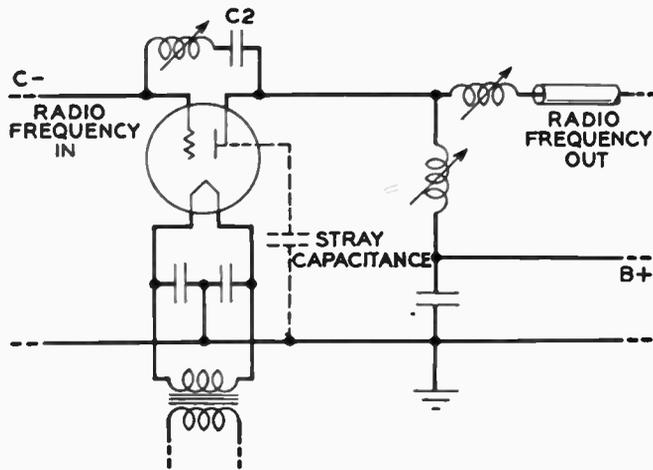
Fig. 2—Schematic diagram of conventional amplifier.
