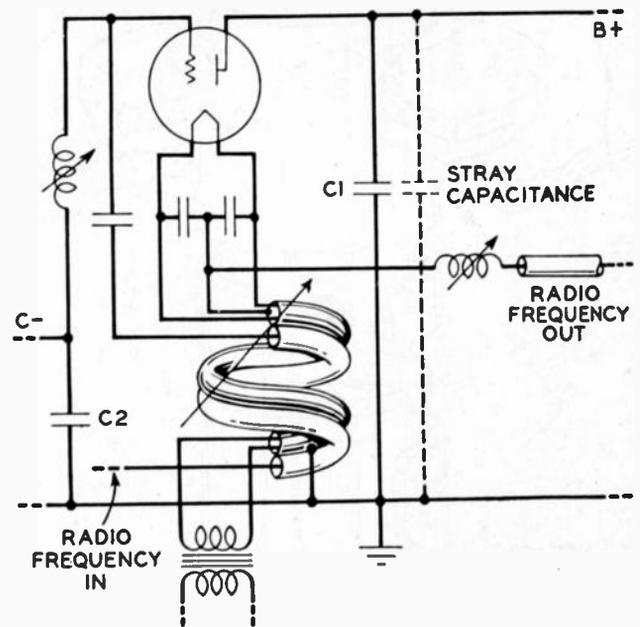
Fig. 3—Schematic diagram of grounded plate amplifier.
