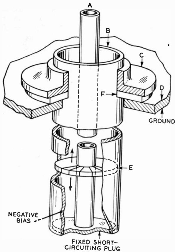
Fig. 4—Neutralizing line.
