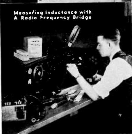
Measuring Inductance with A Radio Frequency Bridge
