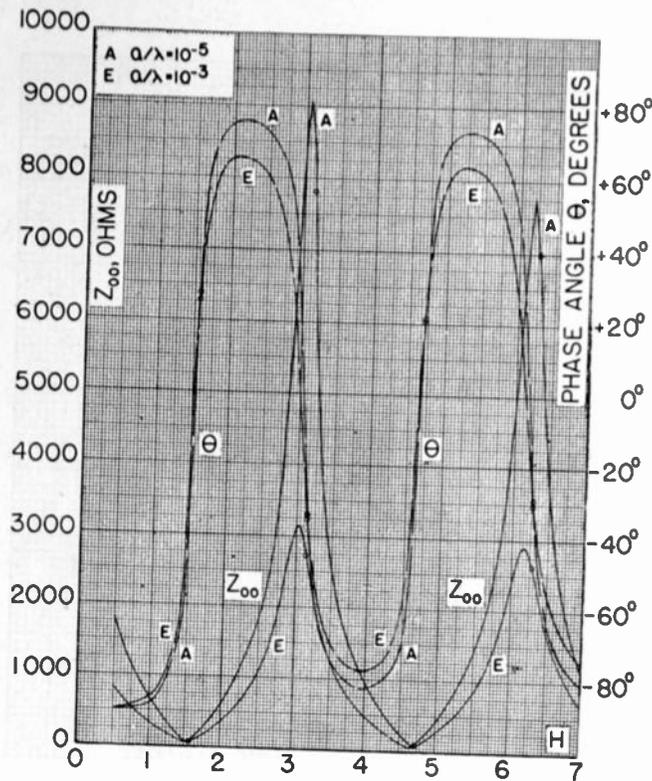
Fig. 6—The magnitude of the input self-impedance  $|Z_{00}|$  and its phase angle  $\theta$  as functions of  $H = 2\pi h/\lambda$  with  $a/\lambda$  as parameter. Values at  $H = n\pi/2$  are indicated by a small circle.
