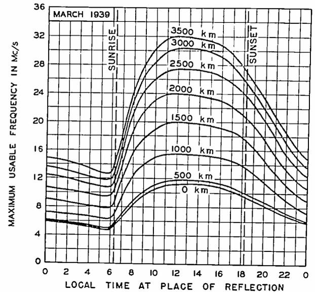
Fig. 2—Maximum usable frequencies for sky-wave radio transmission. Averages for March, 1939, for undisturbed days, for dependable transmission by the regular F and F<sub>2</sub> layers.
