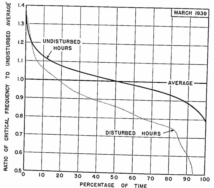
Fig. 3—Distribution of F and F<sub>2</sub> critical frequencies (and approximately of maximum usable frequencies) about monthly average. Abscissas show percentage of time for which the ratio of the critical frequency to the undisturbed average exceeded the values given by the ordinates. The graphs give data as follows: solid line, 399 undisturbed hours; dotted line, 140 disturbed hours listed in Table I.
