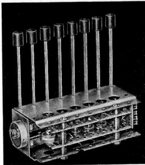
One adjustment controls the frequency of both the antenna and oscillator circuits in this 2-circuit push-button tuner assembly
