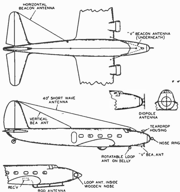
Fig. 6—Location of test antennas on laboratory plane.
