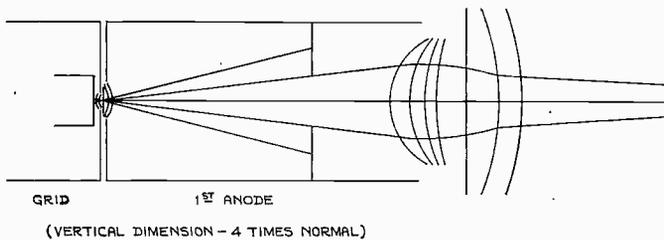
Fig. 8—Diagram of electron trajectories through the electron gun of Fig. 7. The electron lenses are represented by the lines of equal potential.
