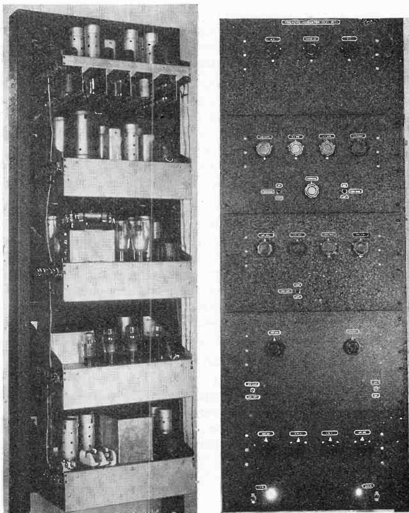
Fig. 12—Rear and front views of test equipment for studying Kinescope resolution.
