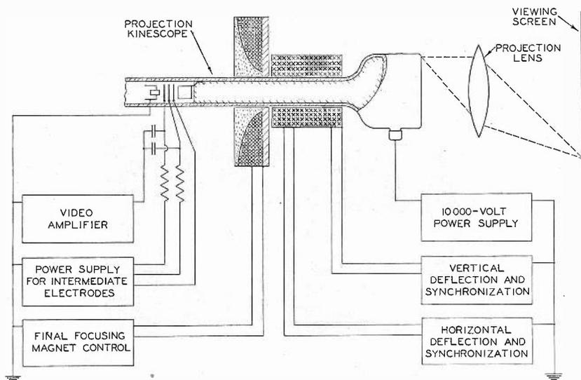
Fig. 14—Block diagram of a projection Kinescope and its associated equipment.
