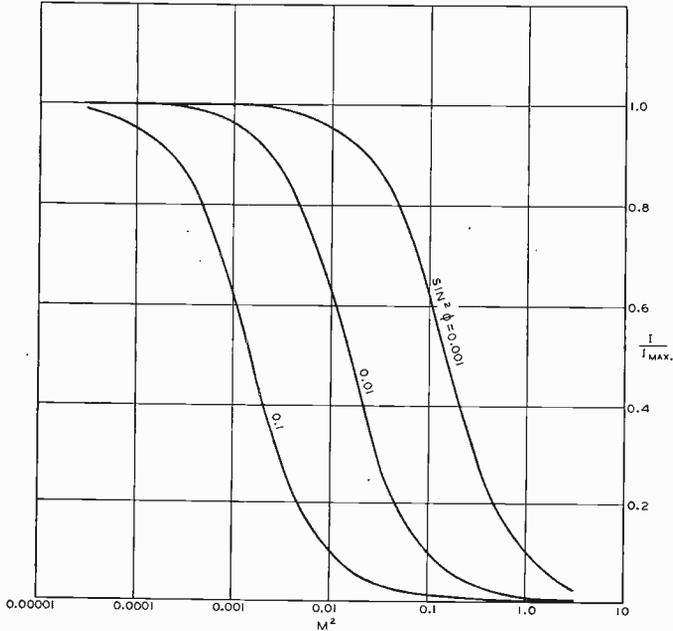
Fig. 2—Current density at image as function of magnification ( $M$ ) and half angle subtended by beam ( $\phi$ ) when  $E_2e/kT = 10,000$ .  $I_{max} = I_0((E_2e/kT) + 1) \sin^2 \phi$ .
