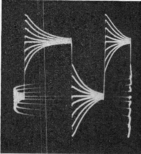
Fig. 13—Wave shapes obtainable during adjustment of attenuators. Final adjustment shown by square wave near center of range.
