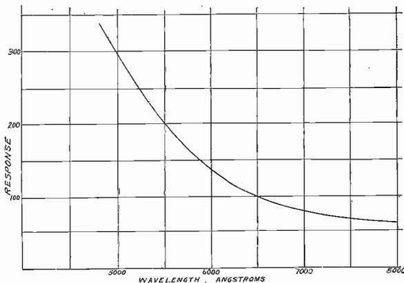
Fig. 9—Color response of standard Iconoscope No. 454.
