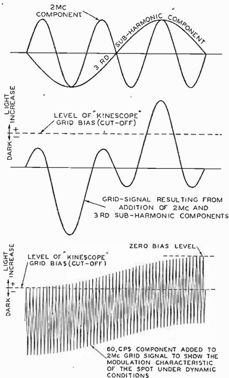
Fig. 1—Grid-signal components.
