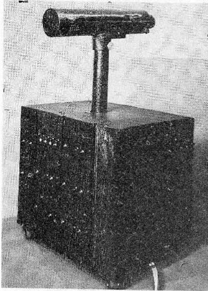
Fig. 15—Laboratory set for demonstrating projection Kinescopes.
