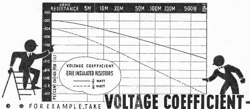
Exhaustive tests run on production samples of Erie Ceramic-Sealed Insulated Resistors show exceedingly low voltage coefficient. For example a 1,000 ohm 1/2 watt unit changes but .002% per volt, a 10,000 ohm unit drops only .0041% per volt, a 100,000 ohm resistor changes .0076% per volt, and a 1 megohm unit .011% per volt.
