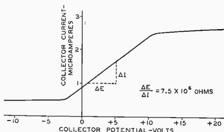
Fig. 7—Curve showing relation between collector voltage and collector current.
