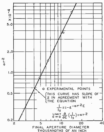
Fig. 10—Variation of  $ar^2$  with final aperture diameter.
