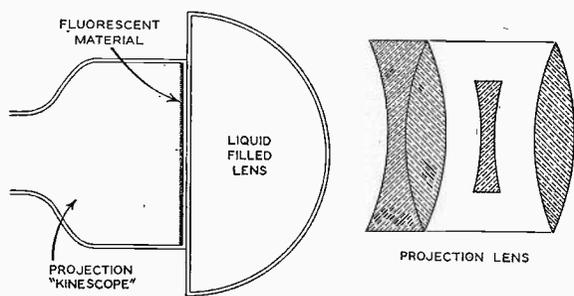
Fig. 11—A hollow shell filled with liquid and sealed to the face of a projection Kinescope will increase the amount of light entering the projection lens. Aberration is a serious defect in this system.
