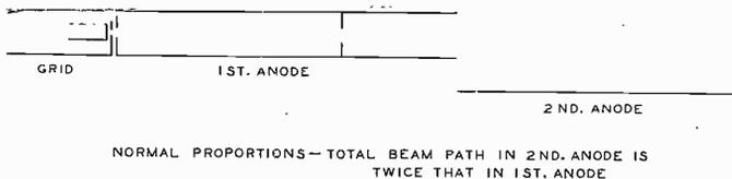
Fig. 7—Sectional diagram of the electron gun used in a projection Kinescope. The second anode is formed by a conductive coating on the bulb wall.
