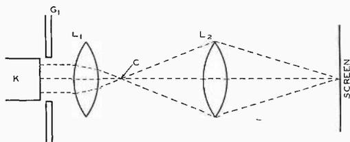
Fig. 1.—Schematic optical analogy of an electron gun.
