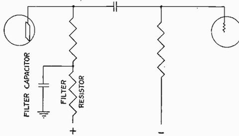
Fig. 5—Basic circuit for correction of relaxation transient.
