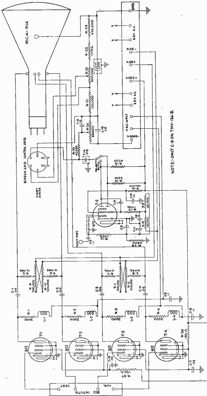
Fig. 7—Schematic diagram—oscilloscope mount of cathode-ray oscillograph.
