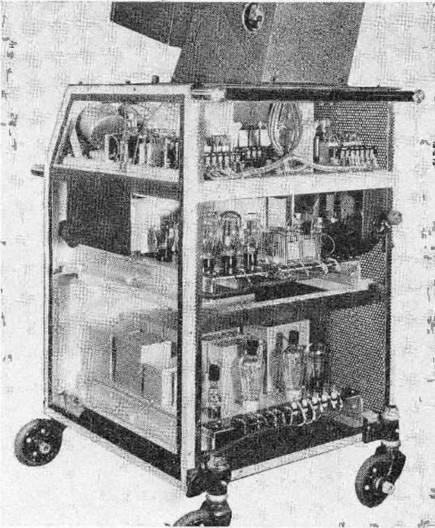
Fig. 2—Back view of cathode-ray oscillograph.
