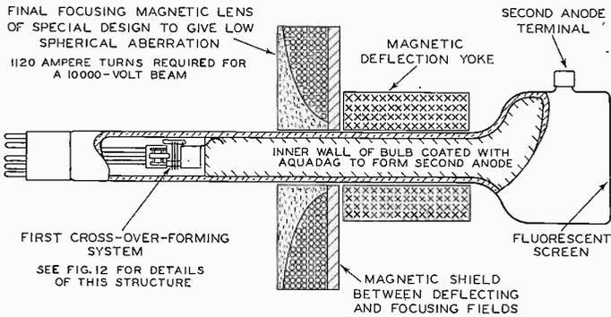
Fig. 11—General assembly of a developmental projection Kinescope.
