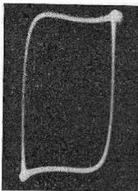
Fig. 18—Demonstration of time of transmission. Vertical deflection—input, wave shape as shown in Fig. 11. Horizontal deflection output.
