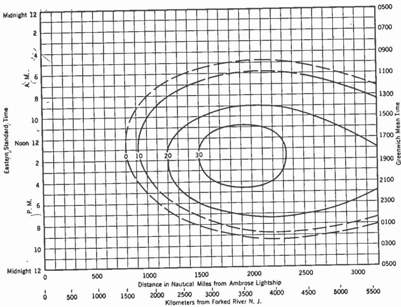
Fig. 31—Approximate variation of radio field strengths with distance and time of day. Contour lines indicate maximum expected field strengths in decibels above 1 microvolt per meter. Frequency 17.6 mc. Summer, 1930-1931. Corrected to 1-kw radiated power. Solid lines indicate portions of contours determined by ship-shore data. Information on diurnal characteristic at 3000 miles supplemented by point-to-point transmission.
