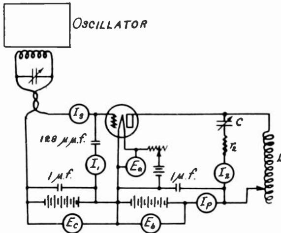
Fig. 6—Measuring arrangement.
