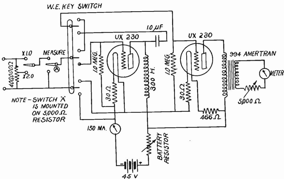
Fig. 2—Circuit of two-tube vacuum tube voltmeter.
