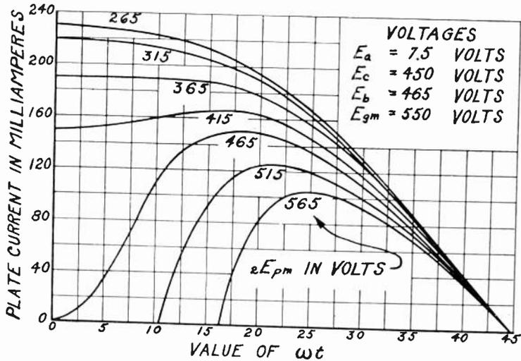
Fig. 5—Graphical solution to show instantaneous plate current vs. value of  $(\omega t)$  for a UX-210 as a doubler.
