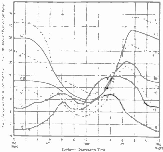
Fig. 10—Diurnal variation of radio noise measured in terms of signal field strength required for a commercial circuit. Simple vertical receiving antenna. Forked River, New Jersey—spring and fall months. Figures denote approximate frequency in megacycles.
