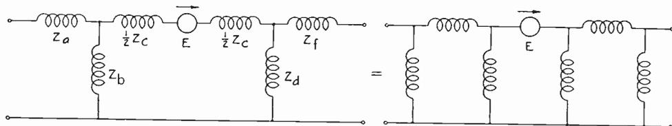
Fig. 3—Equivalent circuits (five independent impedances).
