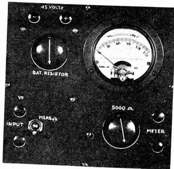
Fig. 4—Panel view of the one-tube vacuum tube voltmeter. (Output meter not shown.)
