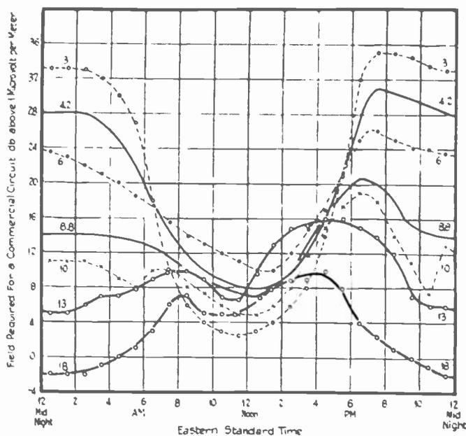
15. 10—Diurnal variation of radio noise measured in terms of signal field strength required for a commercial circuit. Simple vertical receiving antenna. Forked River, New Jersey—spring and fall months. Figures denote approximate frequency in megacycles.
