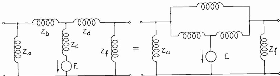
Fig. 2—Equivalent circuits (five independent impedances).
