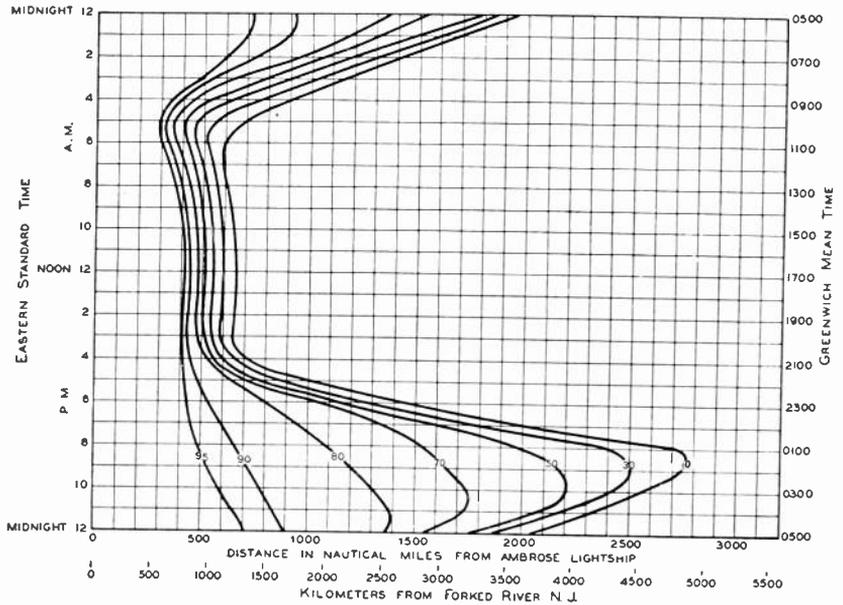
Fig. 17—Approximate variation of per cent commercial time with distance and time of day derived from idealized curves of signal field, data of diurnal variation of radio noise, and data on commercial circuits correlated with signal-to-noise ratios. Transmission from ships in north Atlantic shipping lanes to Forked River, New Jersey. Radiated power approximately 250 watts. Receiving antenna arrays used. Frequency 4.2 mc. Summer, 1930-1931.
