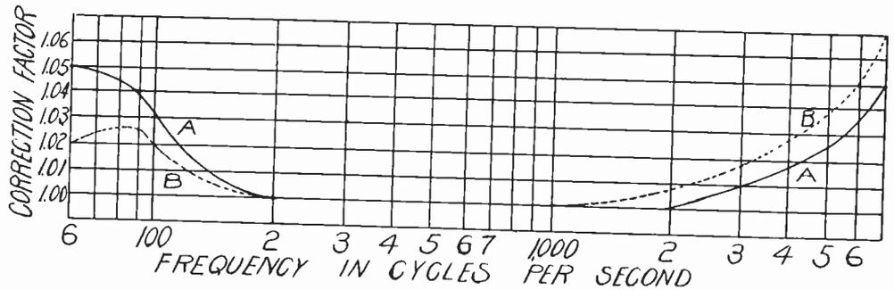
Fig. 3—Vacuum tube voltmeter correction curves. Solid line (curve A) for one tube; dotted line (curve B) for two tubes.
