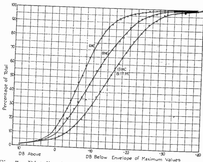
Fig. 7—Distribution of measured fields with respect to envelope of maximum values. 1930-1931.
