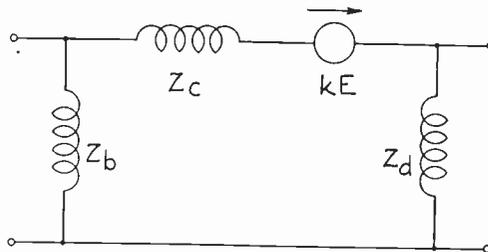
Fig. 8—Equivalent circuit for an active transducer.
