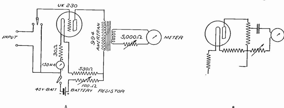
Fig. 1—(A) Circuit of one-tube vacuum tube voltmeter.
