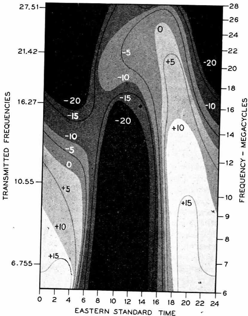
Fig. 1—Average field strength surface for October 12, 1928, to November 1, 1929. Decibels above  $1\mu\text{v}/\text{m}$  for 1 kilowatt radiated.
