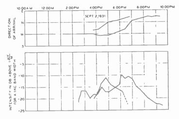
Fig. 9—Direction of arrival and intensity of local storm type static on 14.6 meters.
