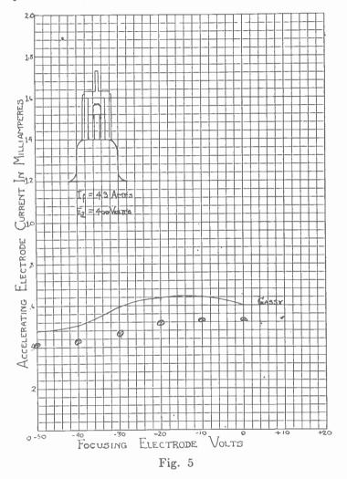
and the accelerating electrode current is proportionally higher, but the spot remains very nearly the same size as with the lower filament current with varying focusing electrode bias.
