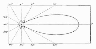
Fig. 3—Directional characteristic of array at 14.6 meters.
