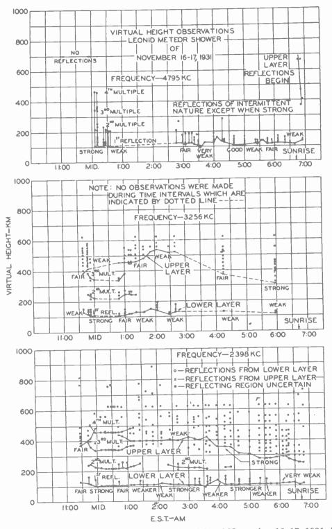
Fig. 1—Virtual height variations during the night of November 16-17, 1931, for frequencies of 2398, 3256, and 4795 kilocycles. Also note the variations in the intensity of reflections. From the behavior of the reflections from the lower layer it appears that there was a large increase in the effective ionization of the lower layer near midnight, and minor increases at about 2:45 and 4:30 A.M.
