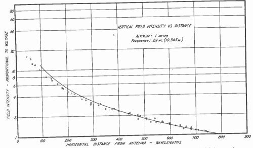
Fig. 2—Theoretical (Sommerfeld) and experimental vertical field intensity vs. horizontal distance from the antenna. Measurements made just over the surface of sea water.
