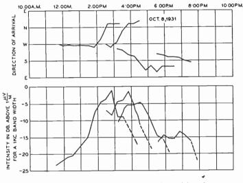
Fig. 12-Direction of arrival and intensity of local storm type static on 14.6 meters.
