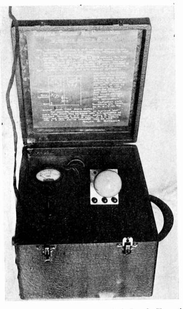
Fig. 1---Photograph of Portable Cathode Ray Oscillograph.
