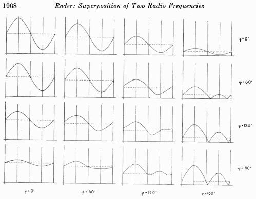
Fig. 3-Same as Fig. 2, but field strength ratio 1:1.5.
