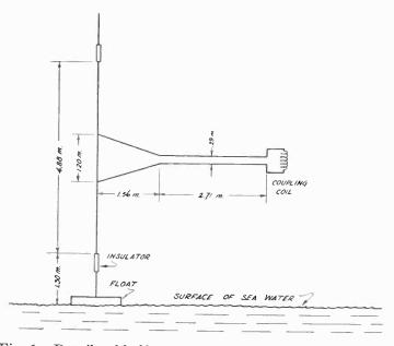
Fig. 1—Details of half-wave, vertical antenna used for the experimental work on 29 megacycles
