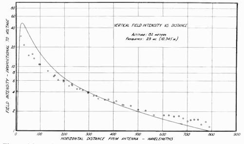
Fig. 4—Theoretical (Strutt) and experimental vertical field intensity vs. horizontal distance from the antenna for altitude of 82 meters.
