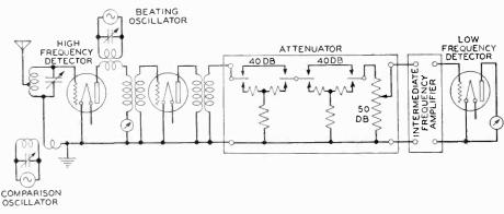
Fig. 1-Schematic diagram of field strength measuring set.
