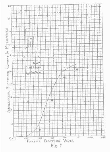
ing electrode and 400 volts applied to the second one located at a greater distance from the focusing electrode. The spot stays quite constant in size except when a high bias voltage is applied. This also shows the nonlinear curve obtained when the accelerating electrode is distributed.
