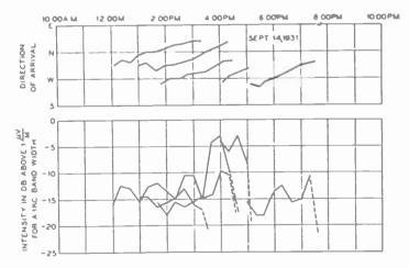
Fig. 10-Direction of arrival and intensity of local storm type static on 14.6 meters.
