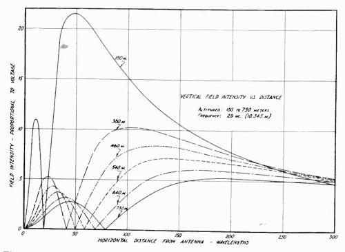
Fig. 18—Composite detailed theoretical (Strutt) vertical field intensity vs. horizontal distance from the antenna, curves for altitudes from 180 to 730 meters.
