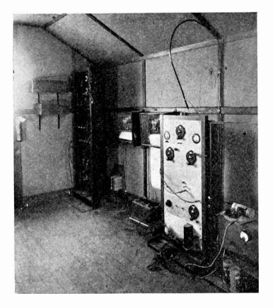
Fig. 5-Long- and short-wave static recording systems.
