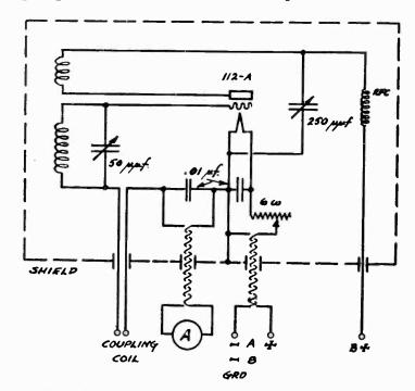
Fig. 21-Wiring diagram of standard signal generator for 29 megacycles.
