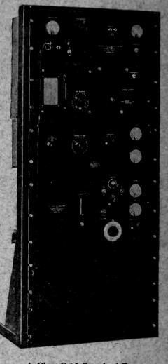
A Class C-10 Standard Frequency Assembly with a Type 616-AR Heterodyne Frequency Meter makes a frequency-measuring outfit that is complete except for the necessary radio receiver.
