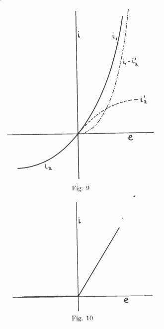
rent of the detector will differ more or less from the envelope of the input radio-frequency voltage. Only for the "linear detector" (Fig. 10) for which  $u_2$ ,  $u_3$ ,  $u_4 \cdots = 0$ , the audio output current will be congruent to the input radio-frequency envelope.
