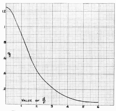
Fig. 6—Field constant for magnetic deflection coils.
