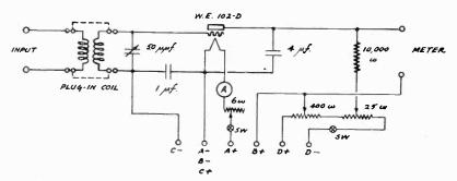
Fig. 23—Wiring diagram of vacuum tube voltmeter used for the calibration of the standard signal generator.
