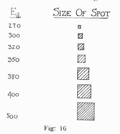
on the first, a minimum size of spot was again obtained. However, with 950 volts on the second accelerating electrode, a minimum size of spot was obtained with 270 volts on the first electrode. In this case the ratio between the two changed to 28 per cent instead of 23 per cent as with the higher voltages.
