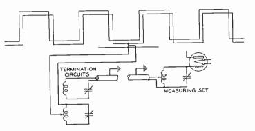
Fig. 4—Schematic diagram of array, termination, and pipe transmission line.
