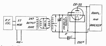
Fig. 1-Schematic diagram of apparatus used to measure detector distortion.
