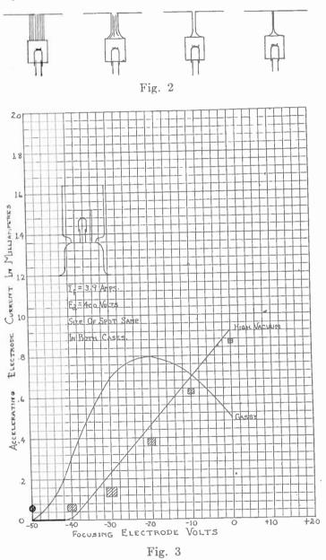
is applied between the focusing electrode and the filament, the electron beam is quite wide and parallel to the sides of the focusing electrode. As the potential applied to the focusing electrode is made negative
