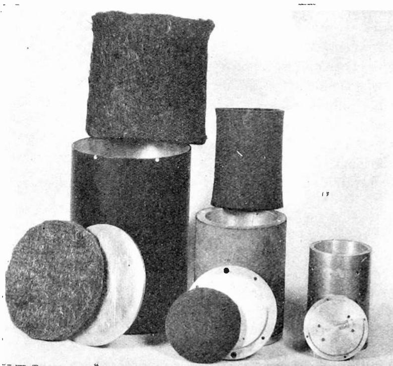
Fig. 2—Disassembled temperature control chamber.
