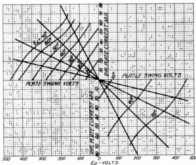
Fig. 5—Auxiliary  $I_p - E_p$  diagram. Two ER-245-type tubes in push-pull derived from Fig. 4.
