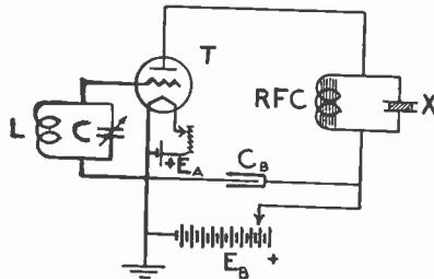
Fig. 21—The Pierce p-f circuit as tested.
