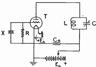
Fig. 14—The Pierce g-f circuit as tested.
