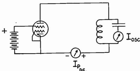
Fig. 5—A dynatron oscillator with no plate battery.
