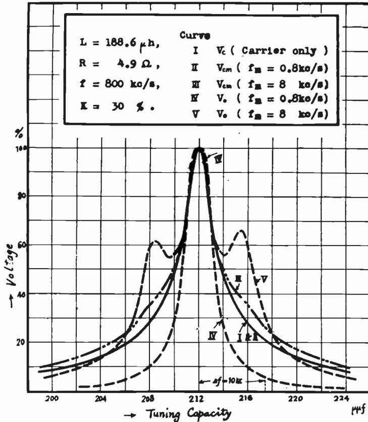
Fig. 15—Resonance curves, No. 1.
