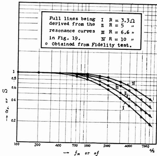
Fig. 20—Fidelity curves derived from the resonance curves.
