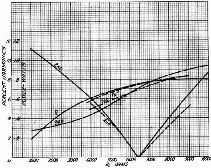
Fig. 3—Measured and calculated values of  $P_0$  and distortion vs.  $R_L$  for full input voltage ER-233 tube.  $E_b = E_{a0} = 135$  volts.  $E_{c0} = -13.5$  volts.
