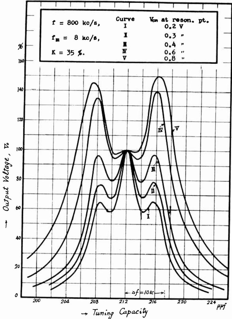
Fig. 18—Variation of the resonance curves due to the signal intensity. No. 2.
