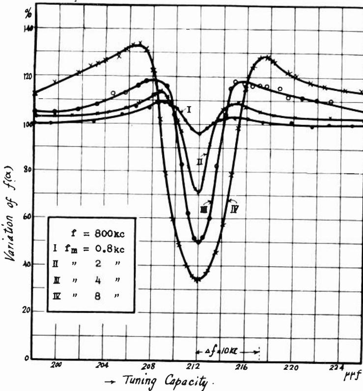
Fig. 11—Variation of  $f(\alpha)$  near the resonance point. (Direct observation, result No. 1.)
