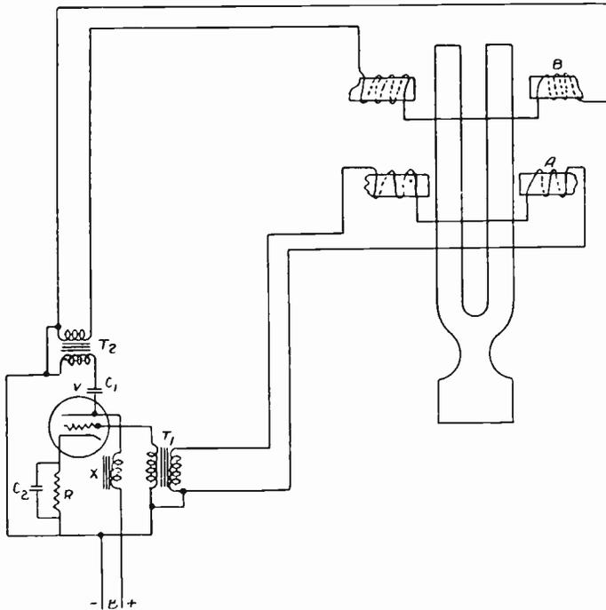
Fig. 1—Simple fork drive circuit.
