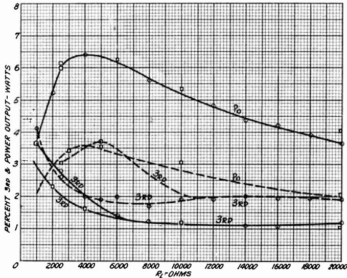
Fig. 6—Measured and calculated values of power output and distortion.
