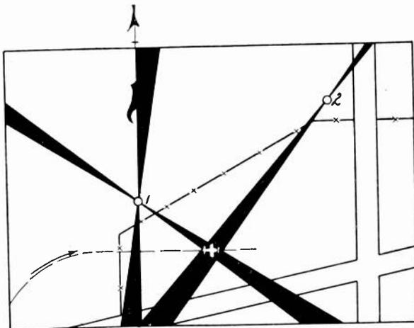
Fig. 3—Map carried in the airplane upon which the position of the airplane is indicated by the shaded segments intersecting above the airport.
