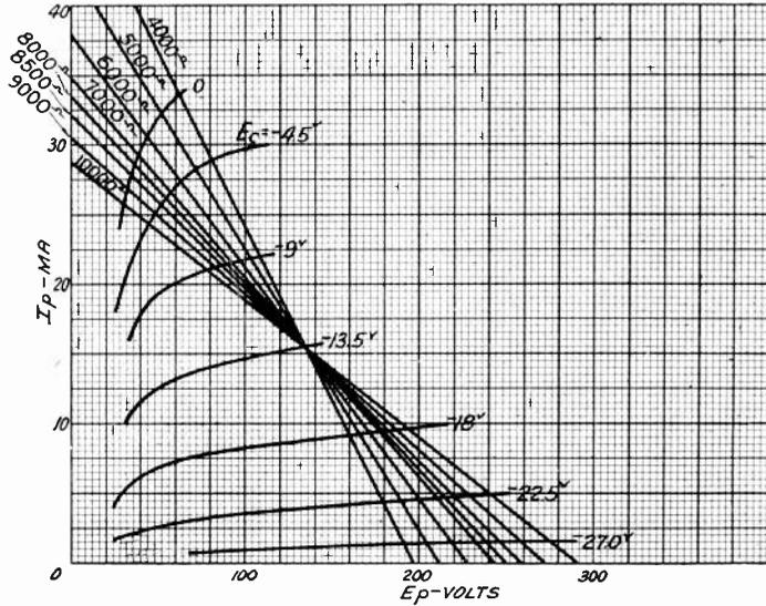
Fig. 1— $I_p - E_p$  characteristics of ER-233 tube.  $E_{sg} = 135$  volts.
