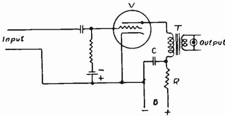
Fig. 9—Vacuum tube circuit for shortening impulses.
