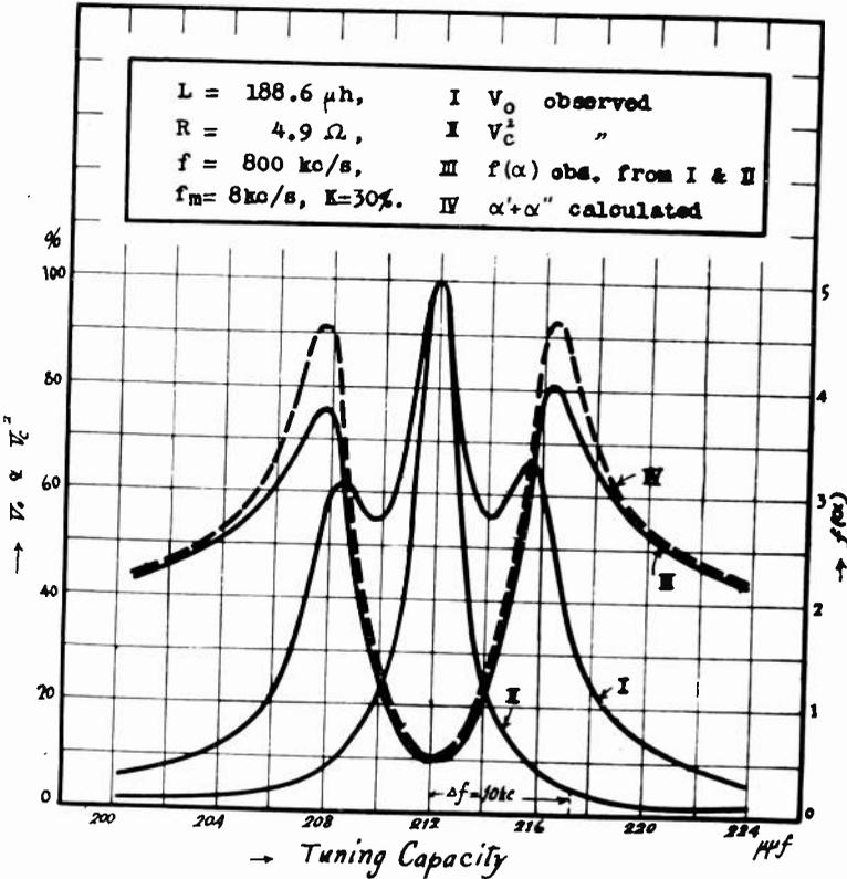
Fig. 13—Variation of  $f(\alpha)$  near the resonance point. (Indirect observation, result No. 1.)
