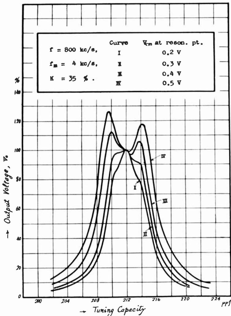
Fig. 17—Variation of the resonance curves due to the signal intensity. No. 1.
