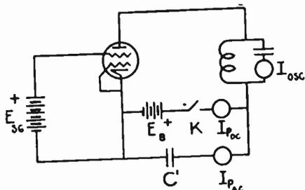
Fig. 7—A second dynatron oscillator with no plate battery.  $K$  is open when circuit is oscillating.
