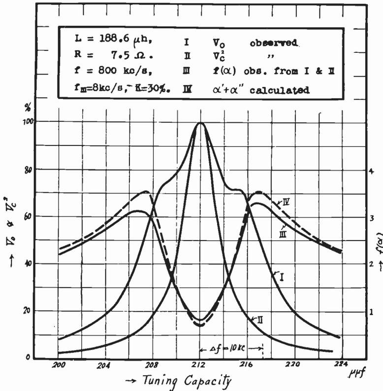
Fig. 14—Variation of  $f(\alpha)$  near the resonance point. (Indirect observation, result No. 2.)
