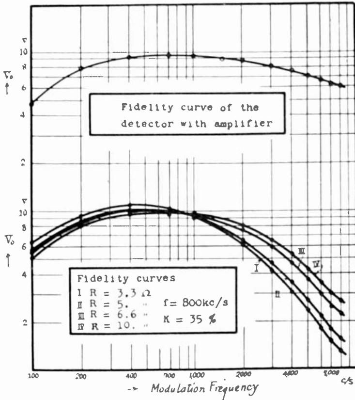
Fig. 21—Fidelity curves observed at the resonance points corresponding to the curves in Fig. 19.
