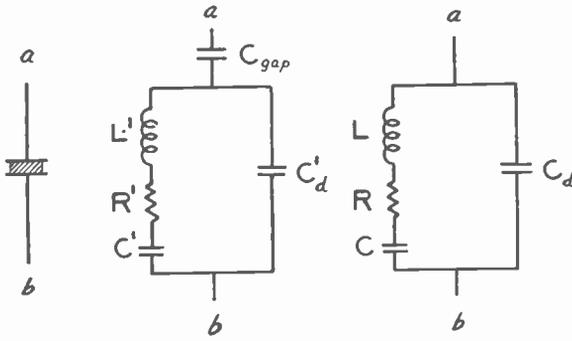
Fig. 9—From left to right, crystal in its holder, equivalent circuit according to Dye, equivalent circuit according to Watanabe.
