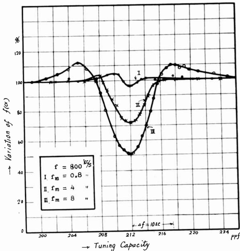
Fig. 12—Variation of  $f(\alpha)$  near the resonance point.
