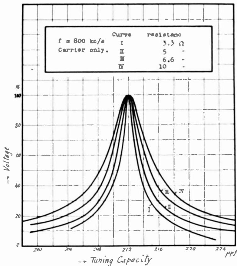
Fig. 19- Resonance curves of carrier voltage.
