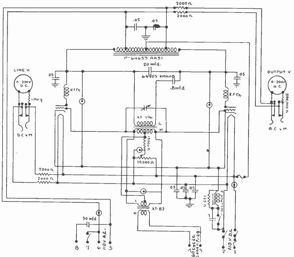
Fig. 7—Circuit diagram of fork controlled inverter.
