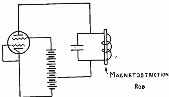
Fig. 13—The magnetostriction controlled dynatron.
