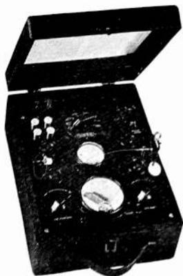
The Jewell Pattern 540 Portable Tube-Seller offers direct reading test facilities for home tests. Line voltage indicator with compensating adjustment and tube short tests are special features.
