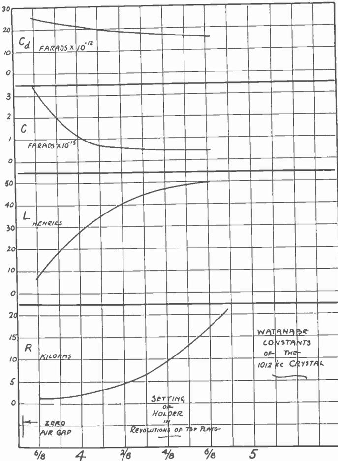
Fig. 10—Watanabe constants of the 1012-kc crystal used throughout the frequency stability measurements.
