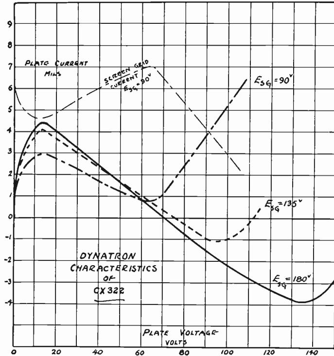
Fig. 6—Dynatron characteristic curves of a CX-322 tube.
