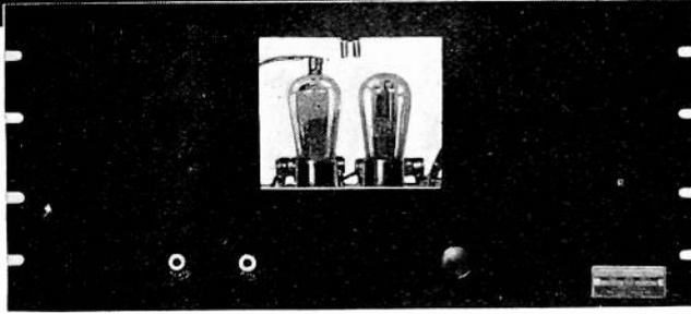
Type 41-A Microphone Amplifier (Door removed)
