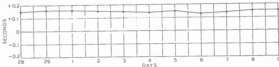
Fig. 12—Rate of one of the clocks driven by an alloy fork plotted against corrected time signals.
