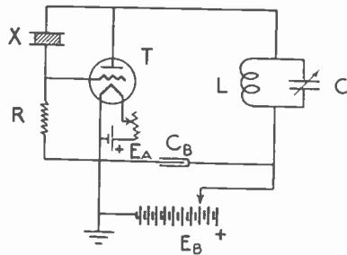
Fig. 18—The Pierce g-p circuit as tested.
