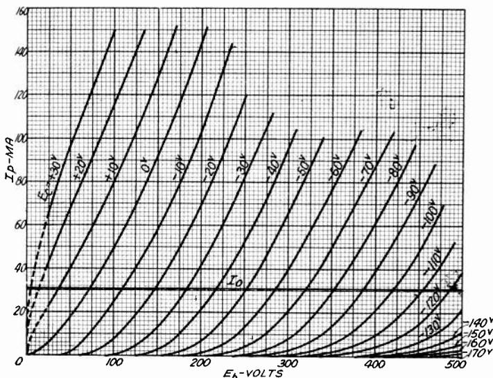
Fig. 4— $I_p - E_p$  characteristics ER-245 tube.
