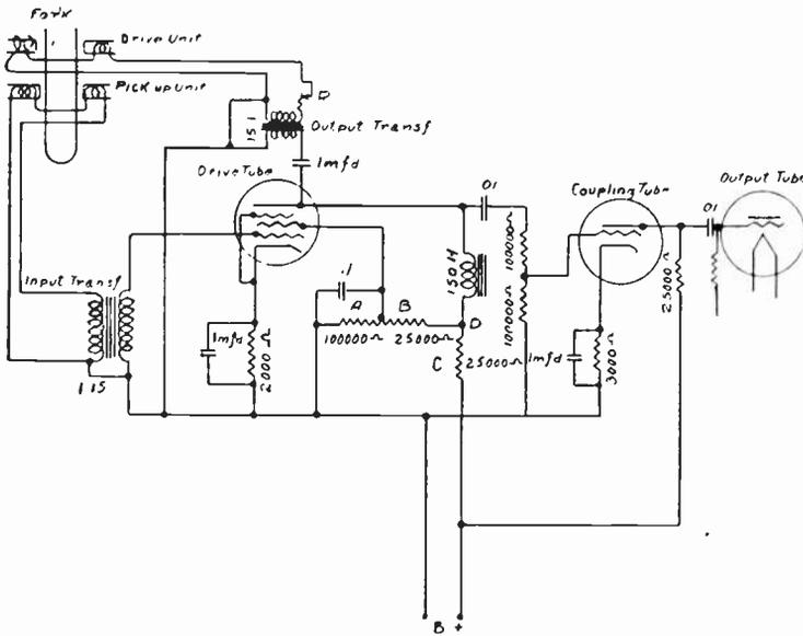
Fig. 4—Stabilized fork drive circuit.
