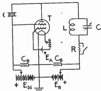
Fig. 23—The sg-p crystal controlled dynatron as tested.
