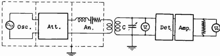
Fig. 10—Circuit arrangement for measuring the side-band coefficient.
