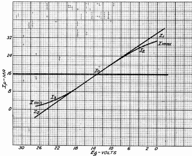
Fig. 2— $I_p - E_g$  dynamic characteristics of ER-233 tube.  $E_b = E_{sg} = 135$  volts.  $R_L = 6000$  ohms.
