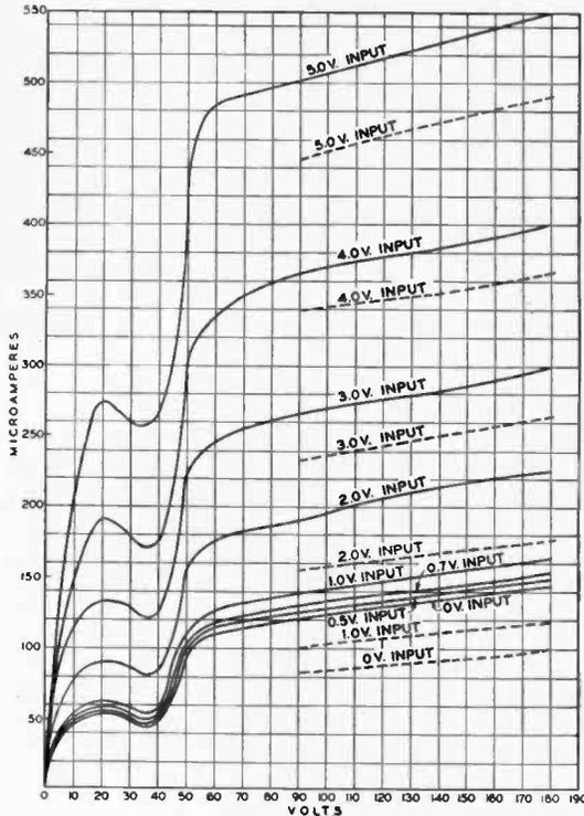
Fig. 6—Plate Current—Plate Voltage Characteristics of CX-322.
