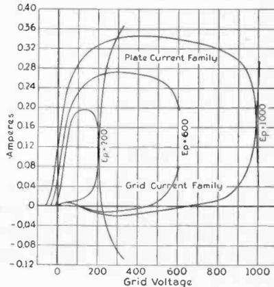
Fig. 1—Characteristics of a 250-Watt Pilotron.
