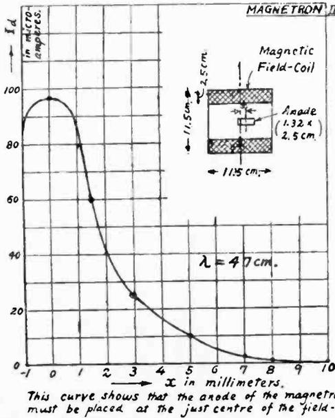
Fig. 26—Variation of Oscillation Intensity with Tube Position in Magnetic Field.
