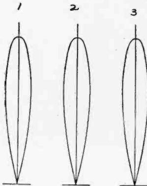
Fig. 36—Polar Curves. 1—Calculation; 2—Horizontal Observed; 3—Vertical Observed.
