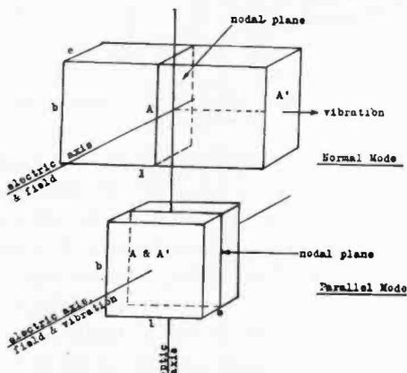
Fig. 2—Crystal Dimensions in Normal and Parallel Fundamental Modes
