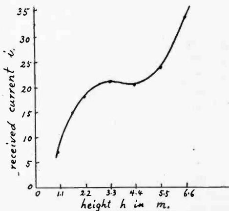
Fig. 5—The Effect of Providing Sending and Receiving Antenna in Fig. 4 with Trigonal Reflectors.
