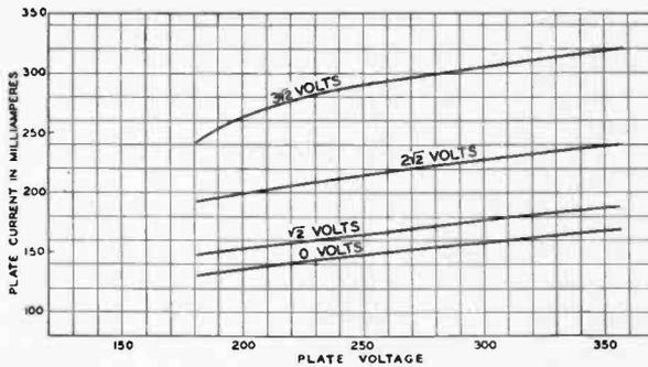
Fig. 8—Plate-Current, Plate-Voltage Characteristics of CX-322.
