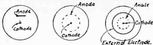
Fig. 23—Types of Diodes and Triode Used Experimentally.
