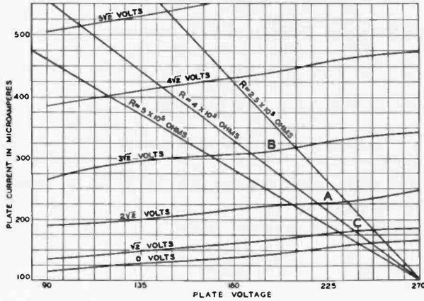
Fig. 7—Plate-Current, Plate-Voltage Characteristics of CX-322. Variable Input Voltages.
