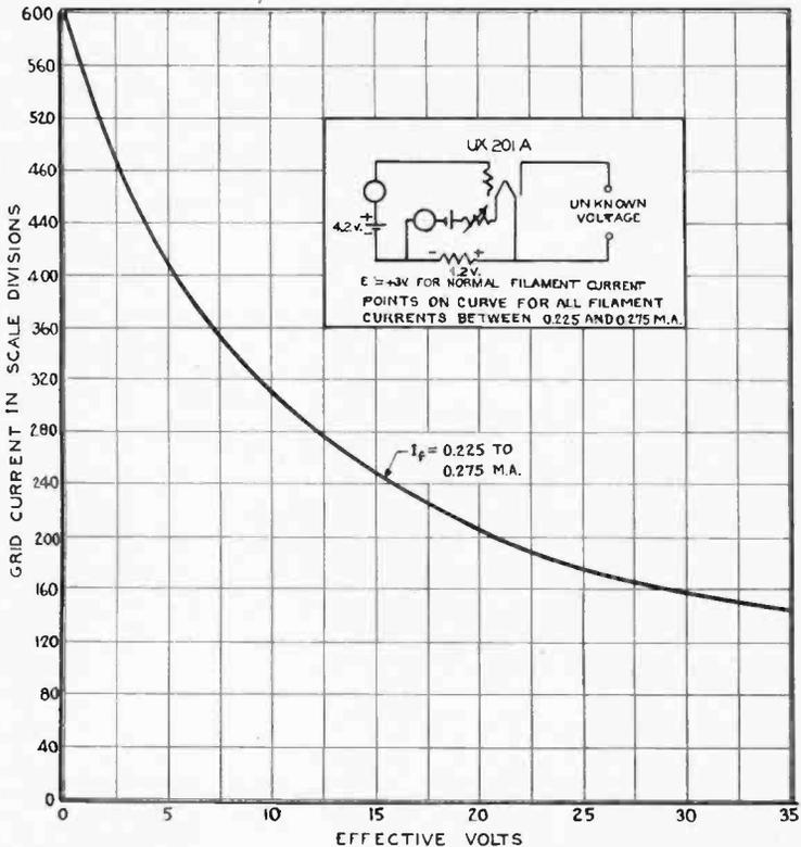
Fig. 2—Compensated Electron Tube Voltmeter; Grid Current Method.
