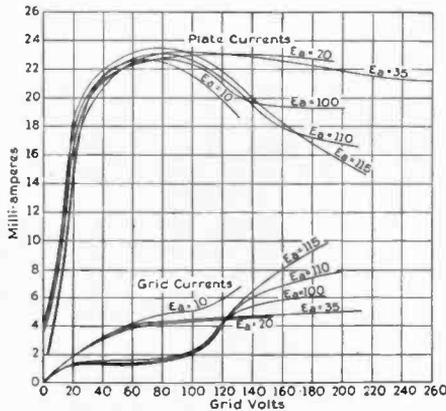
Fig. 2—Characteristics of Tube A with 125 Volts on Plate.  $E_a$  is the Anode or Outer Grid Potential.
