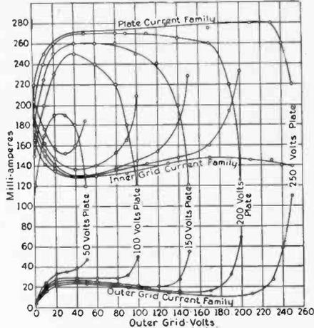
Fig. 3—Characteristics of Tube B with 250 Volts on Inner Grid and 15 Amperes Filament. Principal Dimensions: plate,  $3\frac{1}{4}$  in. long by  $1\frac{1}{2}$  in. in diam.; filament,  $6\frac{1}{8}$  in. of 18 mil. wire (V-shaped); outer grid  $1\frac{1}{4}$  in. in diam. 13 turns per inch of 10 mil. wire; inner grid,  $\frac{3}{4}$  in. in diam. 13 turns per inch of 10 mil. wire.
