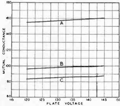
Fig. 4—Mutual Conductance—Plate Voltage Characteristics of CX-322.
