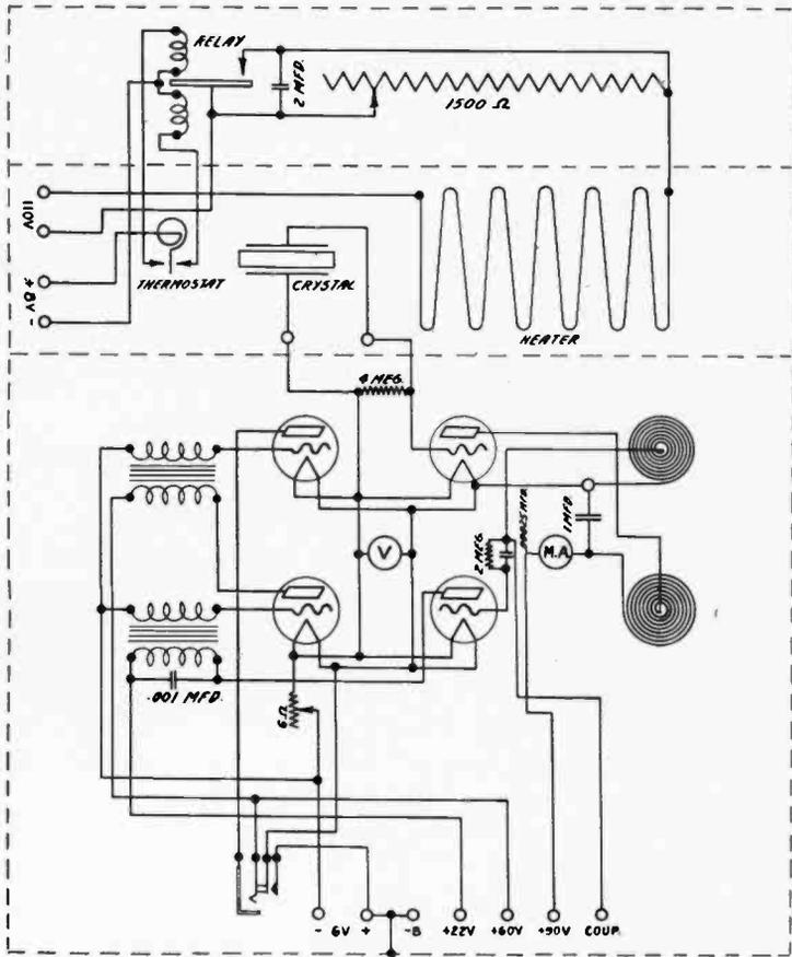
Fig. 4—Circuit of Crystal-Controlled Standard Oscillator Showing Heater Circuit.
