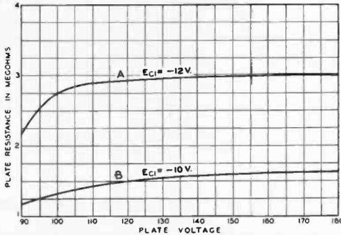
Fig. 5—Plate Resistance—Plate Voltage Characteristics of CX-322.
