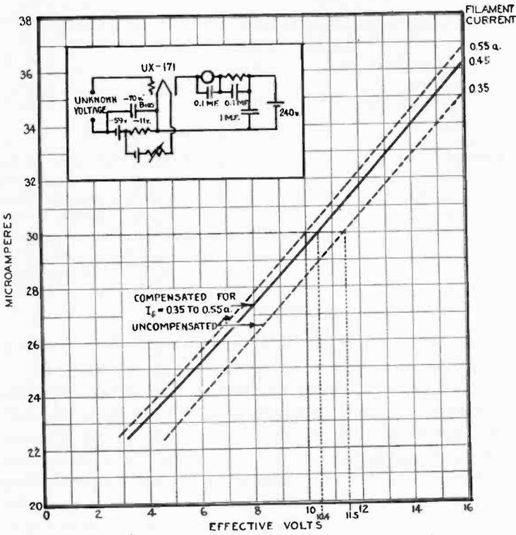
Fig. 3—Compensated Electron Tube Voltmeter; Plate Current Method.
