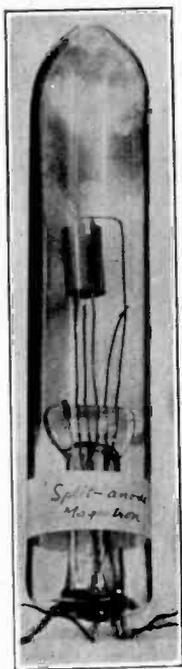
Fig. 29—Split-Anode Magnetron; 2-segment type.
