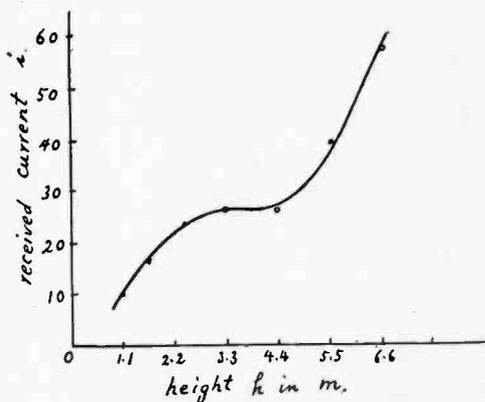
Fig. 4—The Effect of Varying Both Sending and Receiving Antenna Height Simultaneously.
