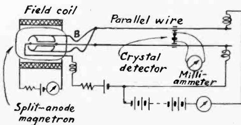
Fig. 31—Circuit Connection for Short Wave Oscillating Magnetron.
