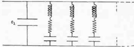
Fig. 3—Single Network Equivalent to Resonator at a Number of Its Natural Frequencies.
