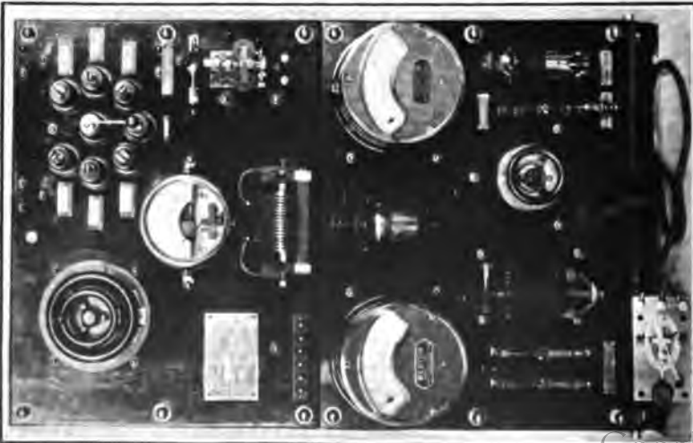
FIGURE 13—Front of 0.5. K.W. Panel Set
