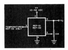
A similar reference source IC is offered by Motorola as the MC1404X and MC1504X devices. These use the same pin-outs as the REF-02 but are housed in 8-pin miniDIP packages instead of the 8-pin metal can of the REF-02. These devices are available in three different standard output voltages: 10 volts (MC1404U10), 6.25 (MC1404J6), and 5 volts (MC1404U5).
