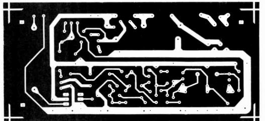
Fig. 3. Actual-size foil pattern is at left, with component placement above. Capacitors C12, C13, C14 and C15 are mounted on foil side.
