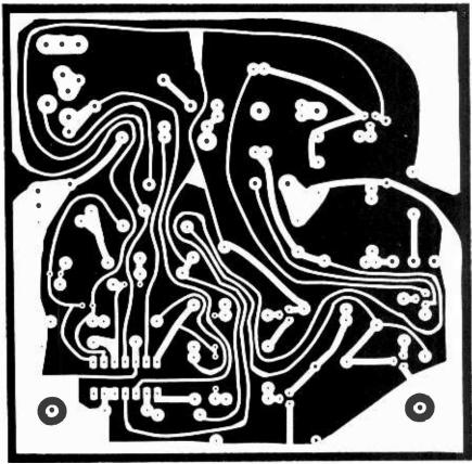
Fig. 3. Actual-size etching and drilling guide for a printed-circuit board for the controller is shown above. Component layout is at top. Note that there are sevral different options regarding components and construction, as outlined in text and Parts List.
