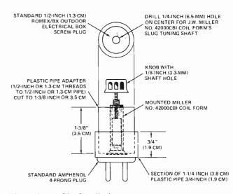
Fig. 5. Assembly details for each plug-in coil (L2).
