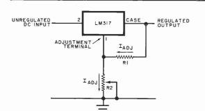
Fig. 1. Basic circuit showing the operation of the LM317 regulator integrated circuit.
