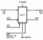
Fig. 3. The 8212, an 8-bit I/O port, and its truth table. This IC has tri-state provisions. That is, in one mode it can be electrically isolated from the system bus.
