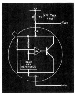
Fig. 5. The Ferranti Electric voltage stabilizers ZN404, ZN423T, and ZN458A/B are used as two-terminal devices.
