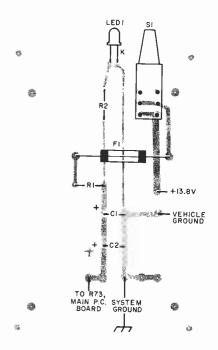
Fig. 10. Component placement for the dc power supply.
