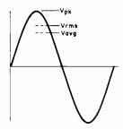
$V_{PK} = 1.414 V_{RMS} = 1.569 V_{AVG}$  $V_{RMS} = 0.707 V_{PK} = 1.110 V_{AVG}$  $V_{AVG} = 0.637 V_{PK} = 0.901 V_{RMS}$ VOMs read 1.110VAVG VTVMs read 0.707Vpk
