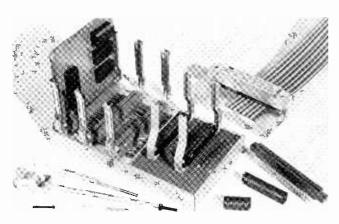
Fig. 8. Typical plug-in card chassis. Three large sockets are Vector Electronics R644-3 with mating BR27-D card guides. Smaller connectors are R644-2 with BR27 card guides. Wire-forming and chiseling tools are also shown.
