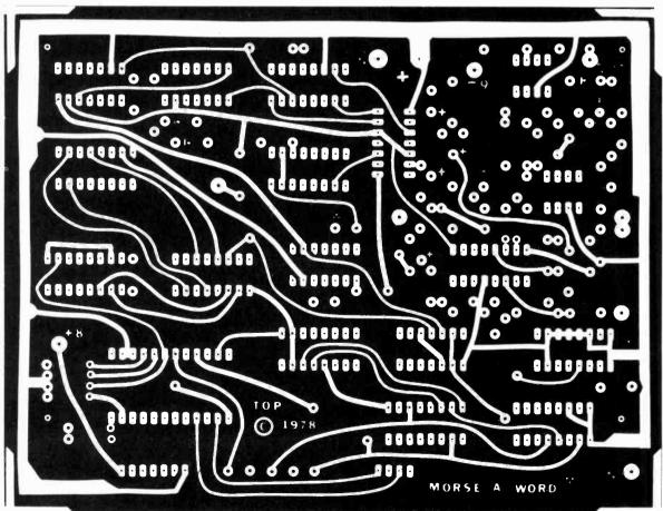
$Fig.\ 6.\ Actual\text{-}size\ etching\ and\ drilling\ guides\ for\ the\ double\text{-}sided\ main\ printed\ circuit\ board.$
