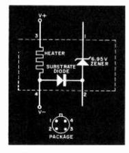
Fig. 4. The LM199 temperaturestabilized zener diode uses an on-chip heater.
