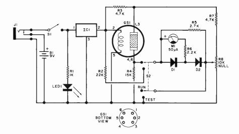
Fig. 1. The gas sensor forms one arm of a Wheatstone bridge. Pins 1, 2 and 3 can be interchanged with pins 4, 5 and 6. Once bridge is balanced by R8, a change in resistance of GS1 will cause meter pointer to swing upscale.
