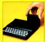
16K MEMORY MODULE: Like any powerful, full fledged computer, the ZX81 is expandable. Sinclair's 16K memory module plugs right onto the back of your ZX81 (or ZX80, with or without 8K BASIC). Cost is \$99.95, plus shipping and handling.
