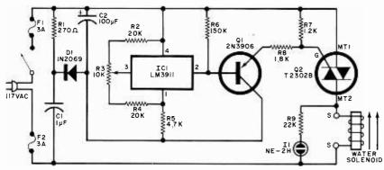
Fig. 1. Temperature sensor IC1, in furnace plenum chamber, determines when solenoid operates to spray fine water mist into chamber.
