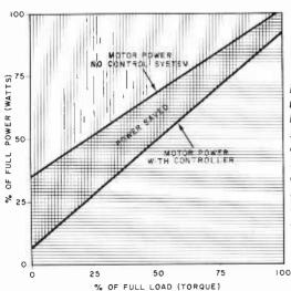
Fig. 1. These curves are the results of tests made by NASA on a ½-hp split-phase and ¼- and ¾-hp capacitor-start motors. Note that the power-factor controller reduced the no-load power demand by a factor of 6. Motor slowdown was less than 2%.
