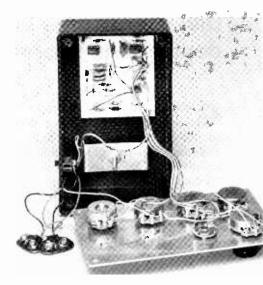
Photo of author's prototype shows pots on front and pc board at rear.
