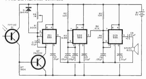
Fig. 1. Timing action of circuit is initiated by light striking Q1.
