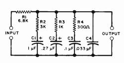
Fig. 1. Low-pass filter with -3-dB/octave response.
