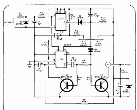
Fig. 1. Frequency discriminator IC1A triggers IC1B to sound alarm when input frequency from distributor points exceeds predetermined limit.
