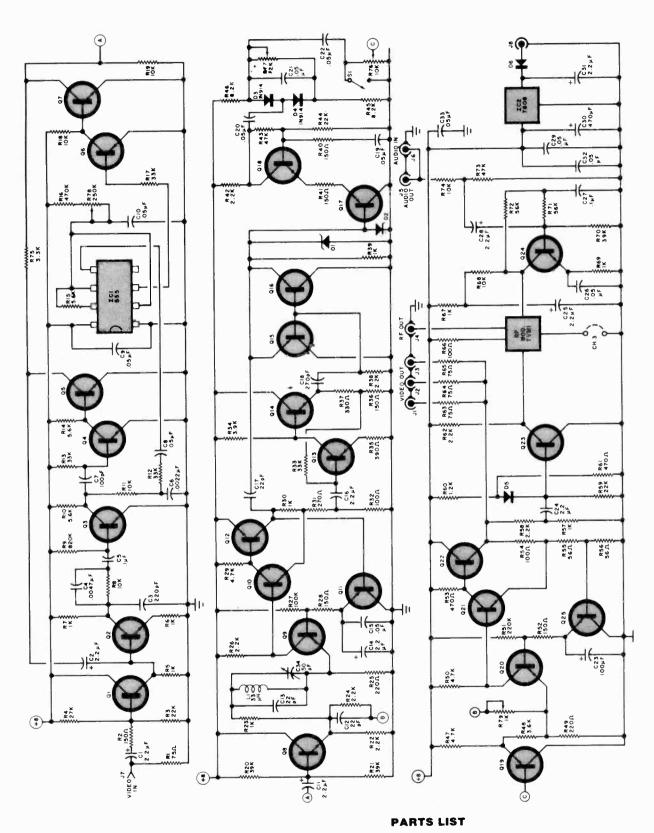
Fig. 6. Schematic diagram of Video Enhancer.
