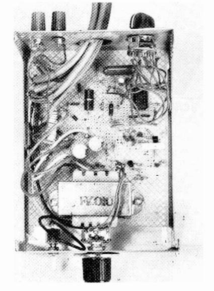
Photograph of the author's prototype which was built on perf board, though a printed circuit board is recommended. The binding posts and switch on the rear were used for testing during design.
