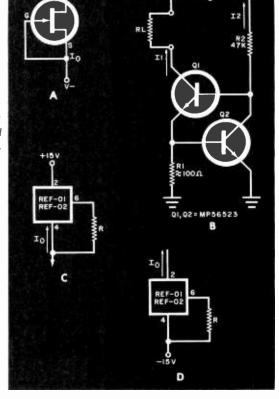
Fig. 6. The Precision Monolithics, Inc. REF-02 reference has a temperature/ voltage output on pin 3, for use as an electronic thermometer sensor.
