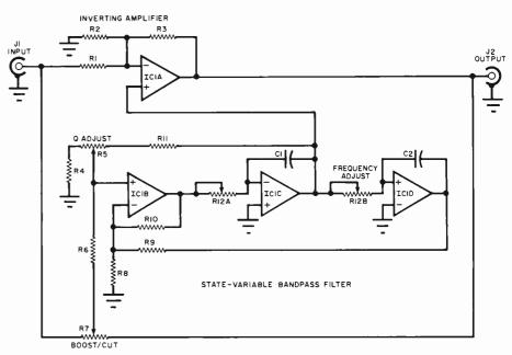
Fig. 1. Simplified schematic of one channel of equalizer shows that an inverting amplifier is interconnected with a modified state-variable active bandpass filter.
