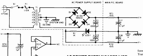
Fig. 3. Schematic of power supply to use with an ac source. It is a conventional fullwave circuit giving plus and minus 15 volts to ground.
