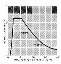
Fig. 3. The 20-watt safe-area curves for the LM317 regulator IC at three operating temperatures.
