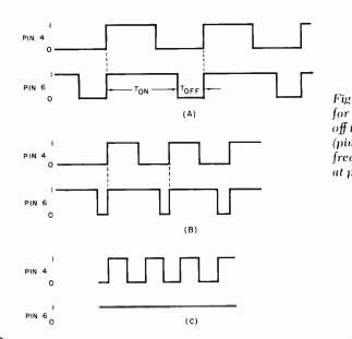
Fig. 2. Waveforms for IC1A show how off time of output (pin 6) varies as frequency of input at pin 4 increases.
