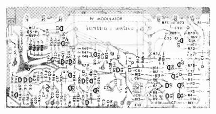
Fig. 7B. Componentsplacement guide for enhancer project.
