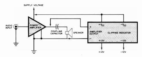
Fig. 3. Diagram showing details of interconnection for amplifiers with bipolar (A) and single-ended (B) power supplies
