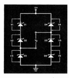
Fig. 2. Several zener diodes may be used in an attempt to stabilize variations in circuit operation due to changes in temperature.
