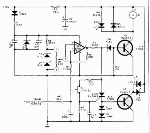
Fig. 2. Comparator IC1 turns on when fuel drops below some predetermined level, and sounds the alarm. The SCR circuit energizes a flashing LED during the Cancel mode.
