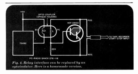
Basic Interface. A basic output interface, an inexpensive SN75492 MOS LED-driver IC, is shown in Fig.1. Six computer output-port pins connect directly to the inputs of the device which can sink up to 200 mA on each of its six outputs. This current is sufficient to directly drive a small relay, LED, or optoisolator. All of the interface circuits given in this article employ the SN75492 as the basic building block.
