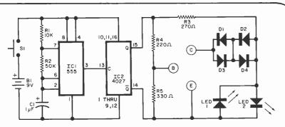
Fig. 1. As shown above, circuit is based on 555 timer operating as a 12-Hz multivibrator.
