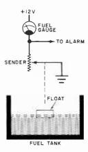
Fig. 1. Typical fuel-gauge circuit.
