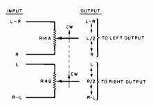
Fig. 3. The left and right signals and the composite are applied to R14 as shown.
