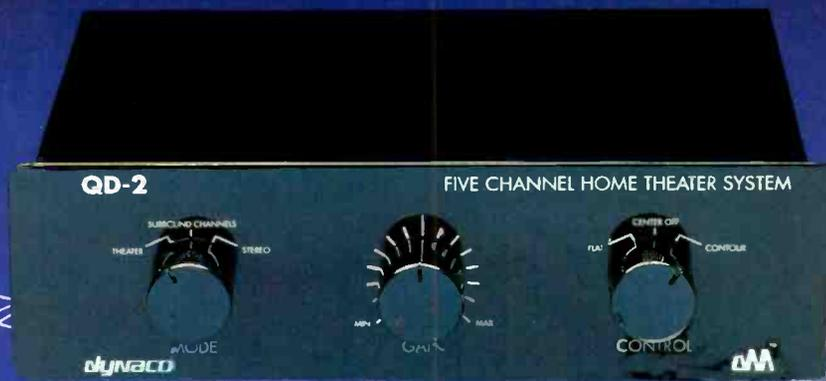
Dynaco's CD-2 (\$140) is a simple passive matrix decoder that routes the stereo difference signal (L - R) from music or a movie soundtrack to a pair of ambience speakers.
