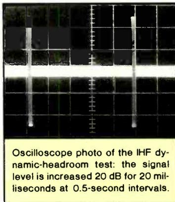
Oscilloscope photo of the IHF dynamic-headroom test: the signal level is increased 20 dB for 20 milliseconds at 0.5-second intervals.
