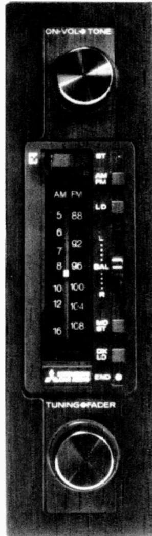
Able to fit "virtually any car on the road today, including X-body models," is Mitsubishi's RX-723 priced at \$150. The super-compact radio/cassette features auto-stop and a pinch-off mechanism that protects the pinch roller. A special nosepiece and faceplate permits both horizontal and vertical installation. Please circle number 137.
