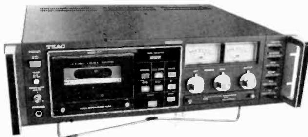
TEAC's C-1 cassette deck may be modified to record and play metal particle tape at a cost of \$150, freight charges included. Modification takes 2 to 3 weeks. The C-1 also offers pitch control, bias optimization modules, optional dbx module. \$1300. Circle Reader Service No. 10 for details.
