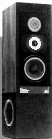
Acoustic Research's \$550 AR-90 includes two 10-inch side-firing woofers, an 8-inch lower midrange element, a 1½-inch upper midrange, and a ¾-inch tweeter in a walnut-veneer cabinet with 3 grilles. 50 watts of power min. is recommended. Crossover freq. are 200, 1200 and 2000 Hz. Level controls for the three high frequency drivers inc. Circle 60.
