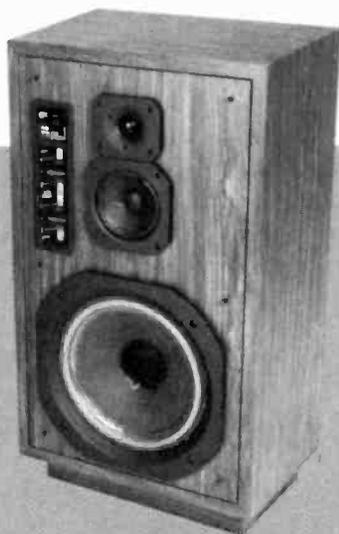
Avid offers the Model 230 speaker as part of its "Un-boxed" speaker line. Designed to minimize cabinet diffraction effects, its drivers include a 10-inch woofer with foam surround, a 4½-inch midrange, and a 1-inch fabric dome tweeter. Crossover points at 475 and 4,000 Hz. Min. recommended power is 15 watts, max. power is 150 watts. Price about \$225 ea. R. S. No. 132.
