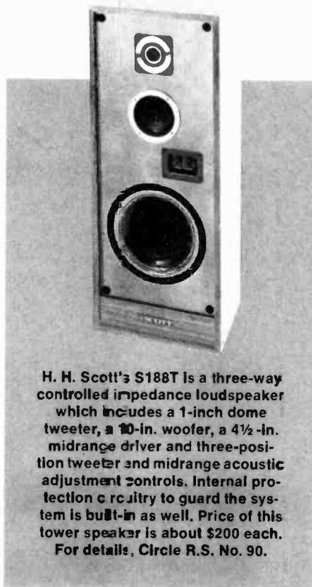
H. H. Scott's S188T is a three-way controlled impedance loudspeaker which includes a 1-inch dome tweeter, a 10-in. woofer, a 4½-in. midrange driver and three-position tweeter and midrange acoustic adjustment controls. Internal protection circuitry to guard the system is built-in as well. Price of this tower speaker is about \$200 each. For details, Circle R.S. No. 90.
