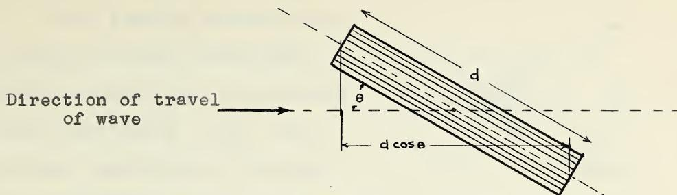
The phase difference between two points one wavelength apart is  $2\pi$  radians, and thus the phase difference between two points  $d \cos \theta$  meters apart is  $\frac{d \cos \theta}{\lambda} \cdot 2\pi$  radians. If the loop is placed at an angle  $\theta$  as shown, voltages of magnitude  $eNd \sin \theta$  are generated in the top and bottom wires, but as there is no phase difference they exactly cancel each other.
