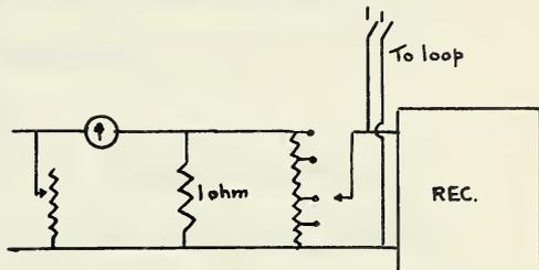
potentiometer. The next arrangement tried was simply a tapped low resistance forming the output resistance through which the known current flowed. The variable resistance was a General
