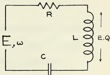
condenser. The loop, being tuned to the transmitter frequency acts as such a circuit and since the voltage generated in the loop by the signal is  $e \times h$ , the voltage that appears across the loop is  $e \times h \times Q$ .
