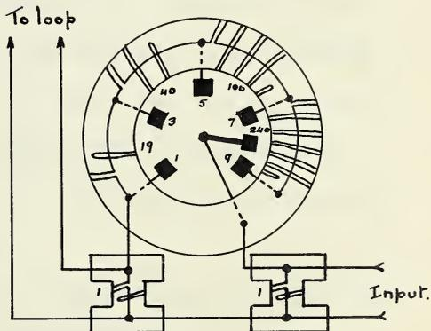
The connection from the rotating selector arm of the switch is soldered to another bolt through the toroid. By this means the toroid is firmly fixed to the switch
