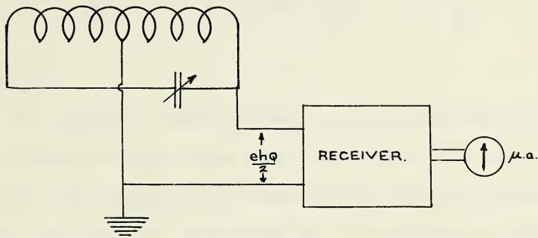
center of the loop to ground. This balances both halves of the loop with respect to ground and thereby eliminates the so-called "antenna effect" of the loop. The ordinary loop voltage is unaffected by this arrangement except that its useful value is reduced to one half of what it otherwise would be.
