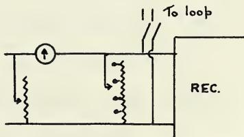
Radio decade box, and a considerable amount of time was spent in calibrating this box at radio frequency with a special type of vacuum tube voltmeter using a screen-grid tube. The decade box, however, was found to have too much inductance, so that it was discarded and a series of small resistors with low inductance was constructed to take its place.
