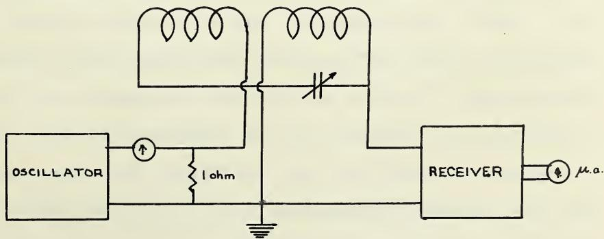
Thus when a known oscillating current is passed through this one ohm, a known voltage is generated in the loop,
