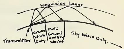
outwards from the transmitter and is vertically polarized since the electrostatic flux of a horizontally polarized wave would be short circuited by the semi-conducting earth. The ground wave is attenuated as it passes over the earth's surface, the amount of attenuation depending on the character of the surface and the frequency of the transmitter, but remaining practically constant as between night and day or from season to season.
