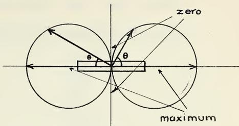
The effective height of a loop of ordinary size is usually small since  $l$  and  $d$  are small compared with the wavelength.
