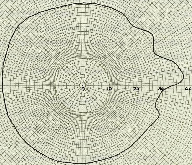
These readings were then plotted on polar paper, (see preceding page) so that the distance from the origin to any point on the curve represents the field strength in that direction at a point 1.69 miles from the transmitter. The curve in the southwest quadrant is estimated since at the time the readings were taken the roads in that area were impassible and observations could not be made on that portion of the circle.
