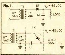
half-wave power supply. This simple circuit forms the basis for a complete family of voltage multiplying circuits, and is shown both in the standard schematic format and a simplified form that will facilitate the development of additional multiplier circuits.
