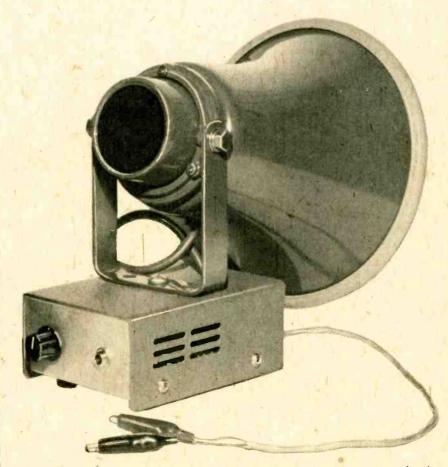
Suggested operating configuration when IC microphone pre-amp circuit is included. This is a 15-watt horn, but less expensive, lower power units will be well within the amplifier power output potential which is about 4 watts with a 20-volt DC supply.
