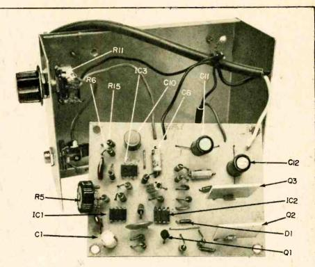
This X-ray view shows where to place parts on the circuit board. The view is of the top of the PC board where all parts but R11 fit.
