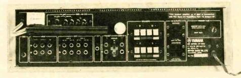
Rear view of the Yamaha CR800: There are stereo inputs for two magnetic phono, aux, and two tape, outputs for two speaker systems, two tape, and phones, as well as an FM detector output.
