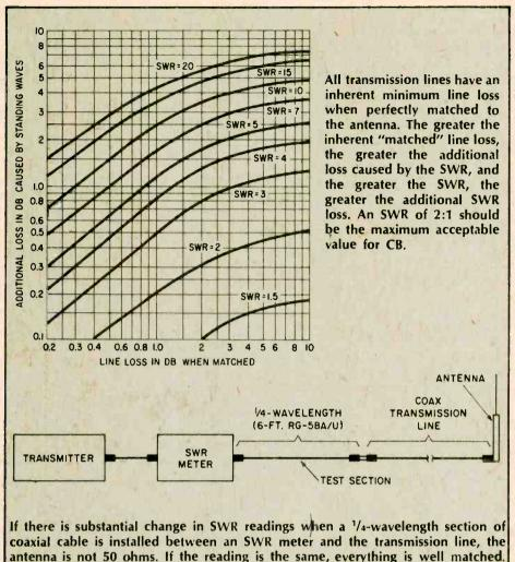
transmission line is an exact half-wavelength or multiple because, as we said, a half-wavelength line behaves as a "one to one" matching transformer. You could have a 10:1, 15:1 or 20:1 actual SWR and still get a 1:1 SWR reading with a half-wavelength line. So you must be certain to "break up" or "tune out" a half-wavelength line. This is done by inserting a ¼-wavelength section of transmission line after the SWR meter—the section indicated as "X" in Fig. 2.
