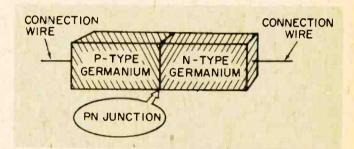
A solid-state diode consists of a section of P-type semiconductor material joined to an N-type section. The activity occurring at the junction of the materials is responsible for the unidirectional property of the diode. The contacting surface is called the PN junction.
