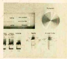
Touch the tuning control and the AFC is automatically disabled while the FM station is tuned for a center-scale indication on the tuning meter. The AFC/station panel lamp to the left of the tuning knob dims, indicating the AFC is off. When the tuning knob is released, the AFC/station lamp glows brightly, indicating the AFC has automatically switched on.
