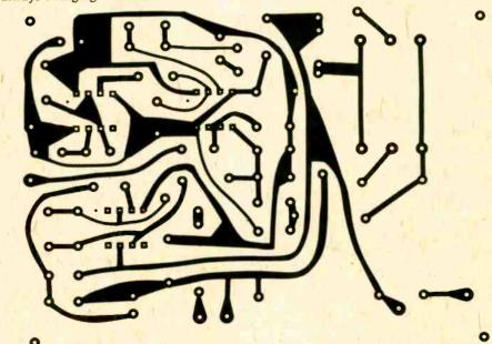
This is the bottom (copper) side of your PC board. You can either etch your own by placing this over a piece of carbon paper and a piece of copper
