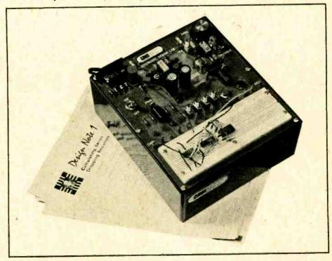
The Designer is a universal breadboarding system for both linear and digital circuits. Logic pushbuttons and switches plus LED indicators make logic operations simple. A decade counter with 7 segment LED display supplied with the program is shown wired on the breadboarding socket.
