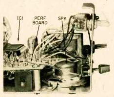
Perf board mounting is simple enough if you use spacers, screws, and nuts as shown. You can mount the display panel (Z1) with anything from double-sided tape to epoxy glue. If you select the alarm option, you must use a small speaker; it can face downward (as shown) or forward for more sound. The kit of basic parts includes the 28-pin IC socket—see parts list for details.
