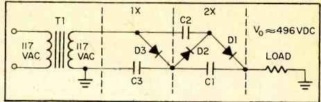
with a load is a function of the input voltage, the source impedance, the capacitor values, the forward voltage drop of the diodes, and the frequency of the input voltage. By assuming that the diodes are ideal (no voltage drop across them in the forward direction) and if the values of all capacitors are made equal (generally the best way to go) the approximate output voltage from a given circuit can be calculated using
