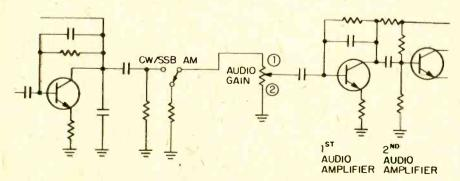
Nearly all of today's new receivers are transistorized. This typical schematic shows your audio take off points. Hook the inner conductor to 1, shield to 2.
