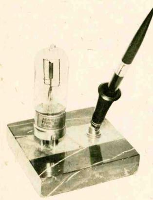
Here we have the famous Westinghouse Aeriotron (WD-11) triode tube which made a big hit in the early 1920s because you could heat the filament (1.1 volts) with a 11/2-volt drycell instead of using a 6volt storage battery. In this case, the author used a desk pen set purchased at a rummage sale for 50¢, and drilled four small holes for the tube base pins to fit in, and then used epoxy glue to hold it fast. Green felt was glued to the bottom of the marble to protect polished desk surfaces.
