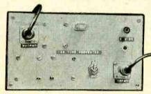
A front panel mounted crystal socket permits moderate shifting of the received frequency without internal retuning. If you use an external 6-volt supply, be sure to remove the dry cell.
