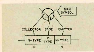
called a junction transistor. The symbol for this type of transistor showing the three elements (emitter, base, and collector) is shown. The three elements correspond to the cathode, grid, and plate, respectively, of a vacuum-tube triode.
