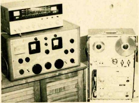
A Roberts 721 reel tape recorder is placed in a convenient spot next to this writer's Hammarlund HQ-150 and Realistic DX-150A. To the left is a B&W #370 SSB (single sideband) adaptor and some home-brew equipment.
