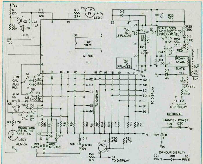
B1-pair of 9-volt transistor radio batteries. Note: required only when standby battery power option is included.
