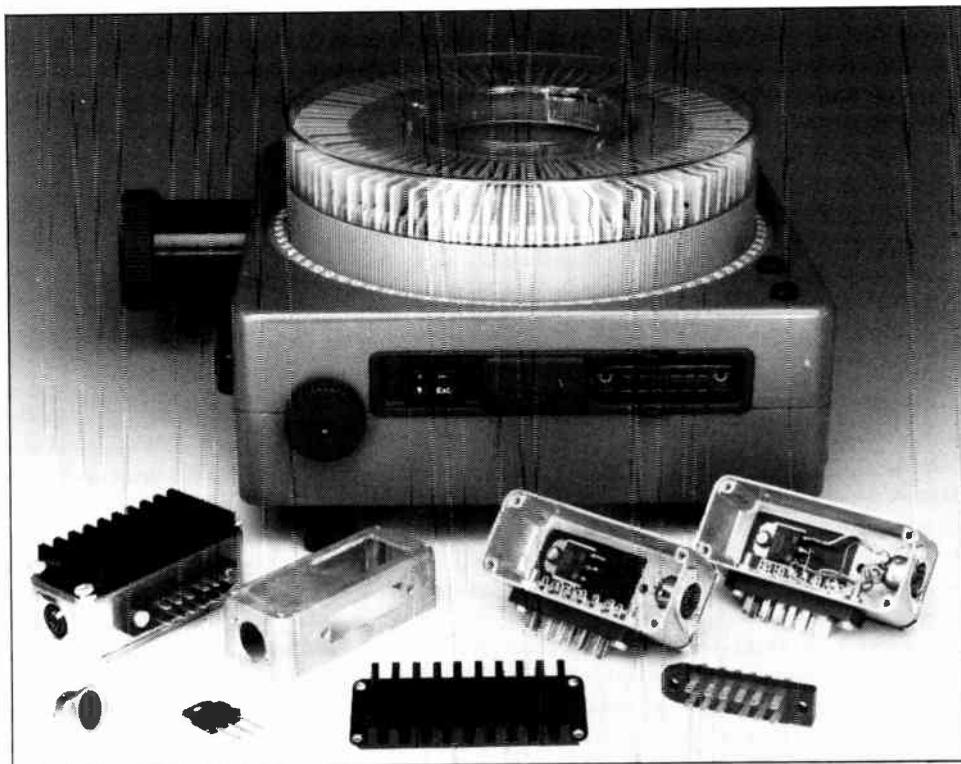
Fig. 14. This photograph illustrates how the triac module is constructed. Do not forget to fit the triac with a thermal insulation set.
