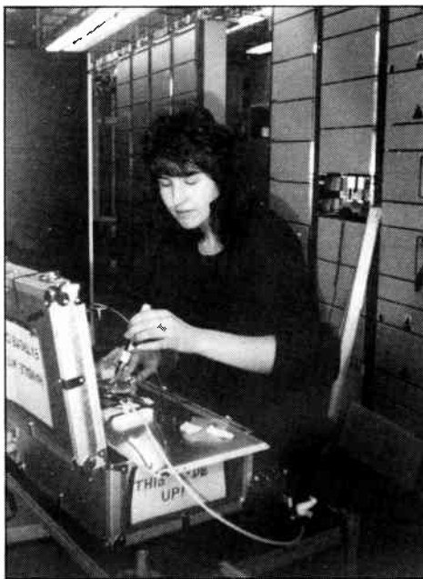
Tests in progress on the submarine optical link between the United Kingdom and the Channel Islands.
