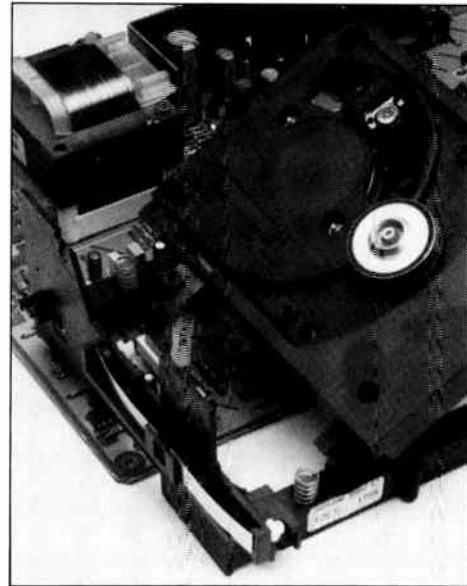
Fig. 9. Laser unit connected to motherboard.
