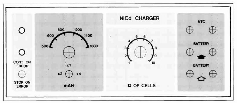
Fig. 10. A front panel foil for the battery charger (196×77 mm) is available through our Readers' Services. WorldRadioHistory ranged at 1:179, which reduces the average charging current of 1800 mA to 10 mA.
