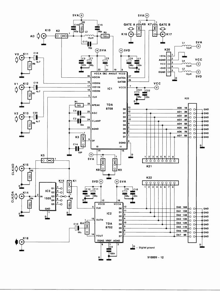
Fig. 10. Circuit diagram of the ADC/DAC converter card. You have the digitized video signal available at a resolution of 8 bits between connectors K21 and K22. A separate connector, K23, allows the card to be connected to a computer bus.
