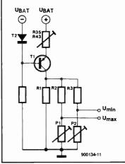
Fig. 6. Circuit for controlling the discharge current. The Dis output of the U2400B provides the reference voltage for IC3.
