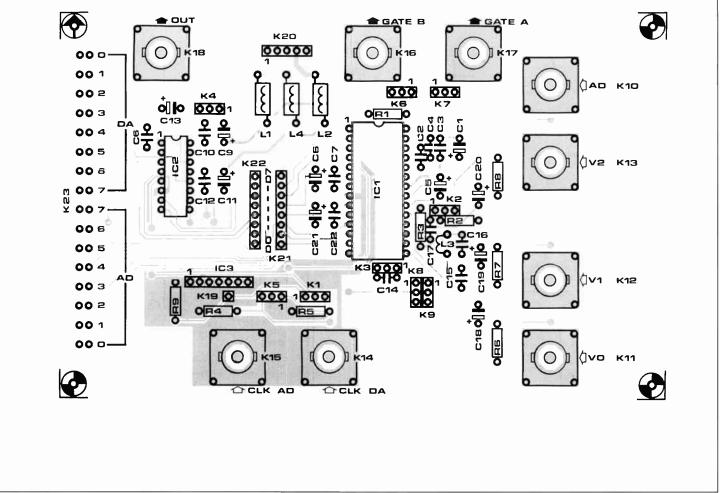
Fig. 11a. Component mounting plan of the double-sided printed circuit board. Note that the board is designed for PCB-mount BNC sockets.
