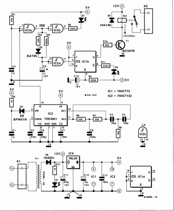
Fig. 4. Circuit diagram of the remote control receiver. The load to be switched is connected to the contact of relay Re1.
