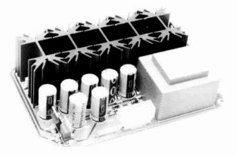
Fig. 18. The printed-circuit board for the power supply has the same dimensions as the busboard. It has no provision for Tr2.
