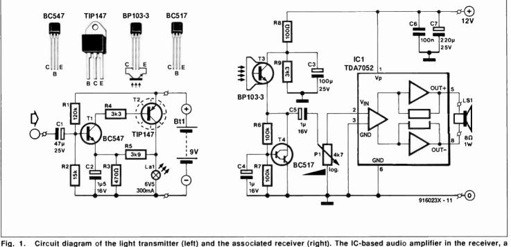
Fig. 1. Circuit diagram of the light transmitter (left) and the associated receiver (right). The IC-based audio amplifier in the receiver, TDA7052, is optional and may be replaced by any other amplifier you may have available.
