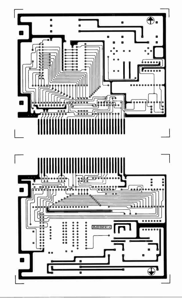
Fig. 3a. Track layouts of the component side and the solder side of the PC insertion card.
