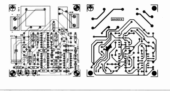
Fig. 5. Single-sided printed circuit board for the IR remote control receiver.
