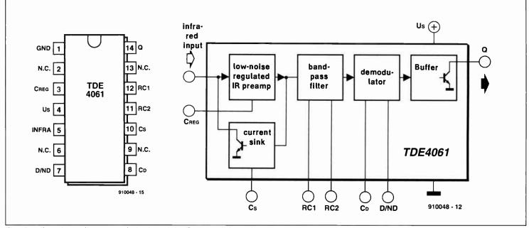
Fig. 3. Functional diagram and pinning of the TDE4061 infra-red receiver IC from Siemens.
