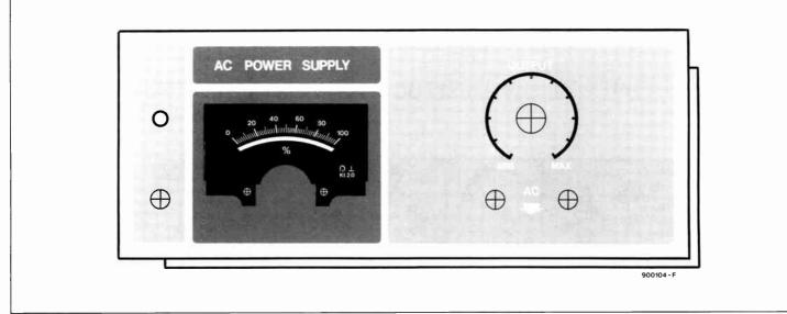
Fig. 6. Layout of the front panel foil (shown here at about 70% of true size). This foil is available ready-made through the Readers Services.
