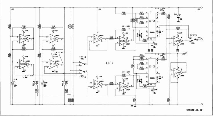
Fig. 10. Generator circuit for the left channel. The right channel is identical, with part numbers in the 200 range.
