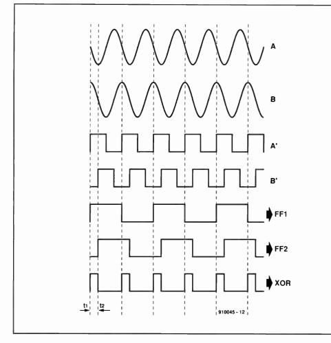
Fig. 2. Timing diagram of the analogue-to-digital conversion section.
