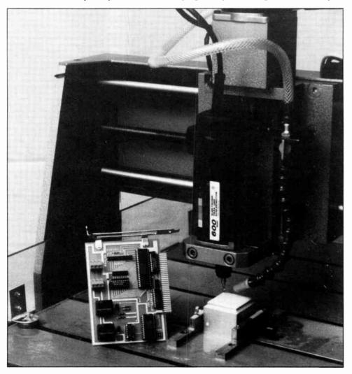
curate processing of aluminium, steel and plastic workpieces. When the project was initiated, there was the choice between (1) 'intelligent' motor control with relatively simple control software, and (2) a simpler controller with powerful, complex, software. To ensure the best possible results in regard of speed and accuracy of the system, the first option requires the motor control to be geared accurately to the specific features of the milling machine.
