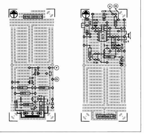
Fig. 2. Compinent mounting plans of the transmitter (left) and the receiver (right). Both are built on ready-made prototyping boards (see the components list).
