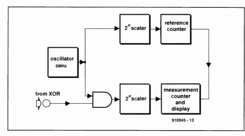
Fig. 3. Block diagram of the digital measuring section.
