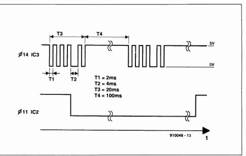
Fig. 2. Response of the TDE4061 to a typical datastream produced by a TV remote control.
