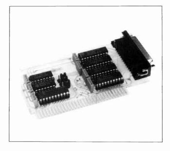
Fig. 28. Photograph of completed IBM interface board.
