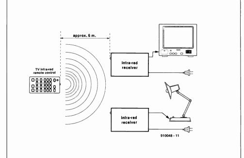
Fig. 1. The remote control supplied with the TV set is used to control a light.
