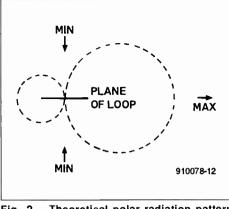
Fig. 2. Theoretical polar radiation pattern of the QTC loop.
