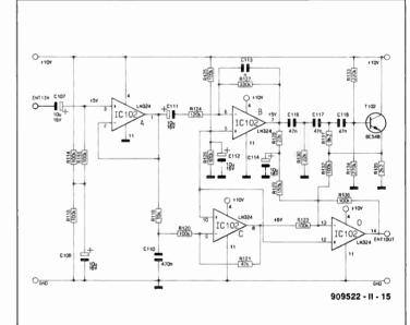
Fig. 11. Compressor circuit (left channel). The component numbers for the (identical) right channel are in the 200 range, and those for the microphone channel in the 300 range.
