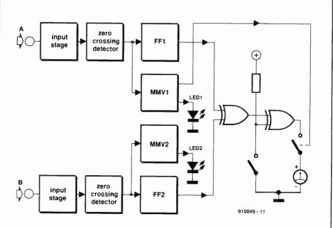
Fig. 1. Block diagram of the digital phase meter.
