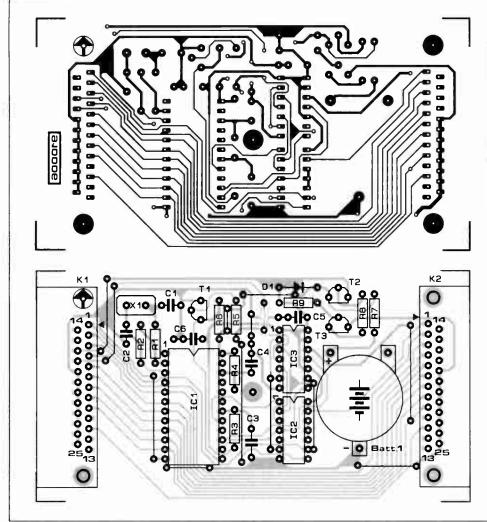
Fig. 2. Single-sided printed circuit board for the real-time clock.
