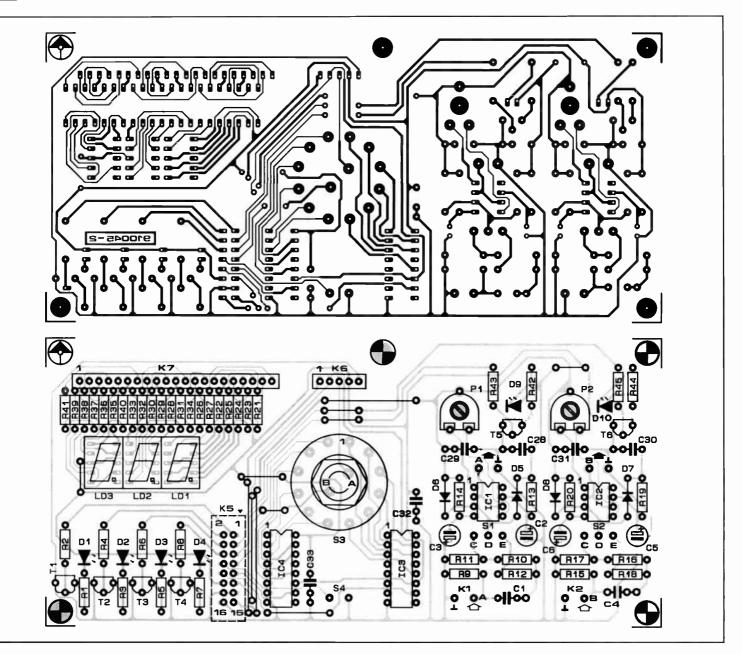
Fig. 8. Printed-circuit board for the displays, input stages, and selector switches.
