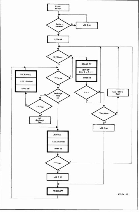
Fig. 2. Flow diagram of the battery charger.
