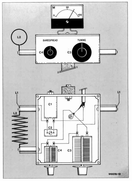
Fig. 3. Mechanical outline of the antenna tuning unit and the field strength indicator.
