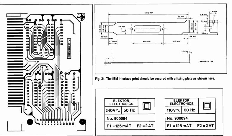
Fig. 25. Suggested labels for the rear panel of the logic analyser.
