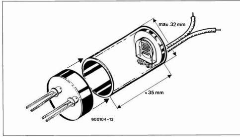
Fig. 5. Basic construction of the home-made optocoupler.
