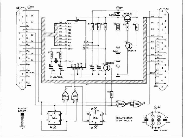
Fig. 1. Circuit diagram of the real-time clock.
