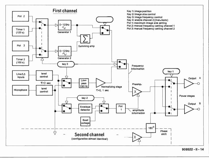
Fig. 8. Block diagram of the laser control unit.
