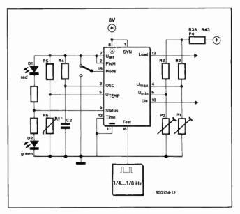
Fig. 1. Basic circuit for the U2400B processor.
