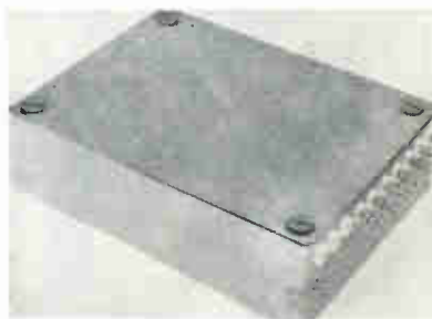
HEAT SINK for module is completed with mounting of metal covers, which also protect encapsulating gel
