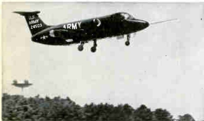
AUGMENTED JET aircraft, designed for VTOL operation is shown in conventional take-off. Lockheed Aircraft Corp. research vehicle is undergoing vertical-take-off tests this year
