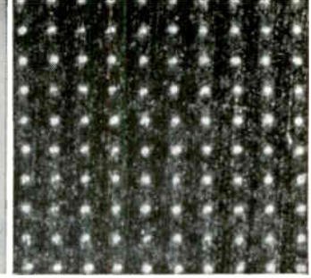
Grid screen of .003" diameter holes on .010" centers drilled in .020" stainless steel sheet.
