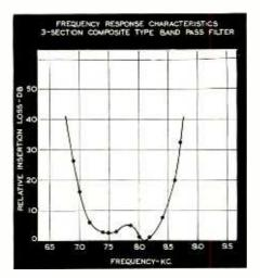
Fig. 9—Response characteristic of three-section bandpass filter used in circuit in Fig. 8
