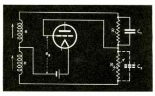
Fig. 3—The operation of the indicator depends upon the balance or unbalance between  $R_1$  and  $R_2$
