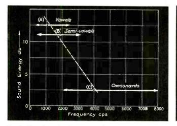
Fig. 1—The relationship between the frequency components and the corresponding power levels associated with various speech sounds, on which Mr. Csepely's scheme is based
