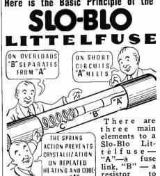
HEATING AND COOL ING OF "A" resistor to furnish heat inertia, and "C" a spring for tension. This Slo-Blo Littelfuse protects equipment having high inductive or capacitative surges. It gives extra value to intermittent duty circuits where frequent cycles of operation would crystallize and break a simple fuse element.
