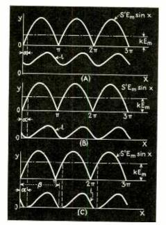
Fig. 4-Voltage and current curves of the rectifier shown in Fig. 3 for the condition of no current cut off
