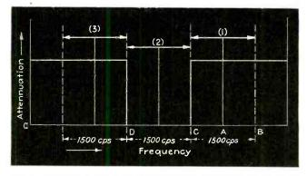
Fig. 3—Characteristic of an ideal 1500-cps bandpass filter, showing how a region 4500 cps wide may be shifted into the pass region
