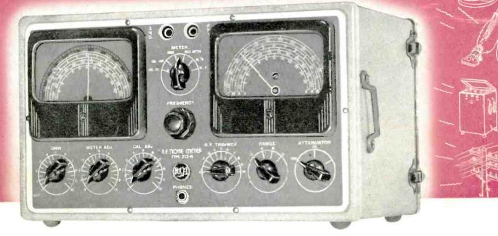
THE NEW RCA 312-A Noise Meter answers a need for a meter to measure radio interference felt by utility companies, manufacturers of electrical appliances, and broadcast stations. It is a flexible instrument designed in accordance with the recommendations of the Joint Committee of the Edison Electric Institute, the Radio Manufacturers Association, and the National Electrical Manufacturers Association.
