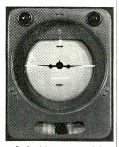
Details of luminous traces which show plane's direction and speed. The traces from top to bottom are gyro compass indication, artificial horizon, blind landing (or altimeter, in center) and air speed
