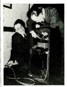
Natural gas drives an electric generator to power the radio receiver shown above. This experimental unit, sponsored by H. Carl Wolf, Natural Gas Company executive, has not yet been developed to a point of practical use in the home
