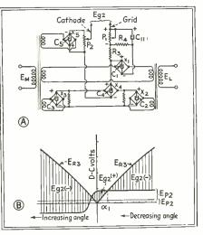
Fig. 3—Grid control circuit for the tube  $T_2$  and the grid control voltage phase difference characteristics
