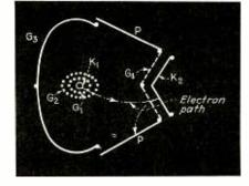
Fig. 3—High mutual conductance tube which makes use of secondary emission and permits the high gain necessary in television receivers
