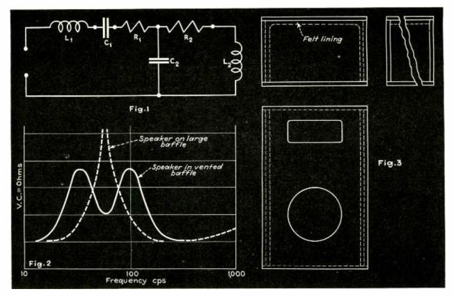
Fig. 1—Equivalent electrical circuit of the mechanical operation of the speaker diaphragm in the vented enclosure. Fig. 2—Impedance-frequency characteristic of the vented enclosure using a 2-ohm voice coil. Note the peaks on either side of the speaker resonant frequency. Fig. 3—The enclosure is lined with material to reduce internal reflections
