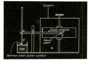
Fig. 7—As the water level changes the frame A also changes causing α deviation in the curve being drawn on the rotating drum
