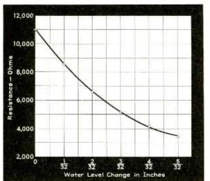
Fig. 5—Curve showing the change in resistance  $R_{\rm 2}$  as the pointer is immersed in the water
