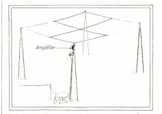
Rhombic receiving antenna and relay amplifier (on tower)
