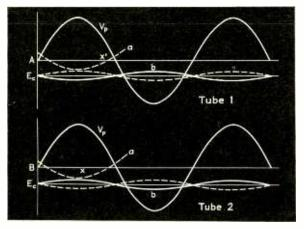
Fig. 4—Curves of the voltages which are applied to the thyratron rectifier
