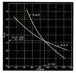
Fig. 8—Curves which determine the duration of current flow through the rectifier elements of Fig. 7 as calculated in Example 3
