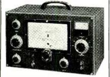
The model CR-6-A beat frequency stand-ard signal generator supplies a reliable signal of known potential and frequency over the wide ranges of from 10 micro volts to 100 volts any where in the range from 10 cycles per second to 50 kilocycles per second.
