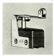
which rests on the plunger of the switch. A case hardened roller is mounted on the end of the lever arm. An 0.008 inch movement at the end of the lever arm moves the switch plunger 0.001 inch and a pressure of 2 ounces at the end of the arm will exert a pressure of 16 ounces at the actuator point. Minor adjustments can be made by slightly bending the lever arm.
