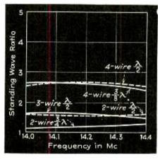
Fig. 4—The standing wave ratio is quite constant over the operating range from 14.0 to 14.4 Mc. A 570 ohm line was used
