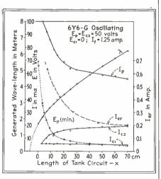
Fig. 3—Oscillation characteristics of the 6Y6-G tube at high frequencies when used in the circuit of Fig. 2
