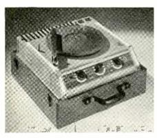
and tubes are readily accessible through a hinged door. The other item is Model 1420 combination 6 volt d.c.—115 volt a.c. PA system. The power output of 20 watts is obtained at a distortion of less than 5% total harmonic content. When used on a 115 volt line, the circuit is of conventional design. A plug arrangement permits operation on a 6 volt storage battery and a heavy duty vibrator changes the d.c. to a.c. Provision is made for either microphone or phonograph reproduction.
