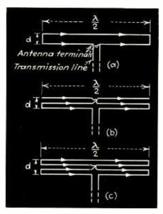
Fig. 1—Two, three and four wire half-wave antennas. The instantaneous currents are in phase with each other and their directions are indicated by the arrows
