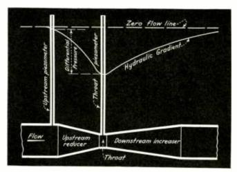
Fig. 1—Venturi tube, in which the hydraulic pressure at the throat is less than at other points
