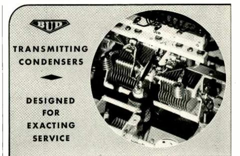
Here is a BUD Junior Transmitting Condenser (No. JC-1569) as installed in a special amplifier designed to operate from 2 to 32 megacycles. This particular unit was selected because it has the valuable Maximum-to-Minimum Capacity ratio of OVER 22-to-1 in addition to many other outstanding BUD features including Center-of-Rod Rotor Contact, Ceramic Insulated Tie Rods, Fitted Cone Bearings, Alsimag 196 Stator Insulation, and many others.
