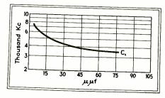
Fig. 3—Values of C<sub>1</sub> required for constant 500-kc bandspread
