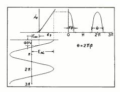
Fig. 4—Voltage and current relationships in the rectifier.  $\Theta$  represents the time of current flow in the rectifier
