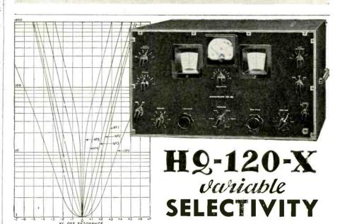
The selectivity curves above indicate overall selectivity at six different positions of the crystal selectivity switch. This feature allows the operator to adjust selectivity to conform with various degrees of interference. Uniform output is maintained throughout the entire selectivity range. Details of circuit are contained in a 16-page booklet.
