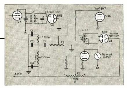
Fig. 4—Schematic diagram of the differential modulation meter. The outputs of the r-f and a-f rectifiers are applied to the opposite ends of the resistor R
