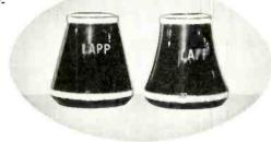
Left, early Lapp Compression Cone. Right, curved side compression cone—same dimensions, wall thickness and weight—twice the compression strength of the straight side cone—the design used in all footing and guy insulators (see below) since 1932.
