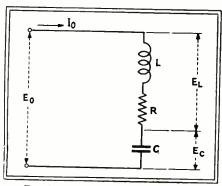
Fig. 1—Basic series circuit used for inductance measurement
