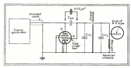
Circuit for determining tube capacitances with a signal generator and radio receiver as measuring equipment
