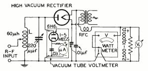
Fig. 2—Practical rectifier circuit for r-f power measurement
