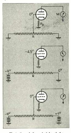
Illustration of the principle of the differential modulation meter. Fig. 1—Top, both ends of the resistor are grounded and the grid bias is zero. Fig. 2—Center, a negative voltage is applied to the left end of the resistor and the bias is one-half the applied value. Fig. 3—Bottom, a positive voltage is applied to the right end of the resistor and the bias is returned to zero
