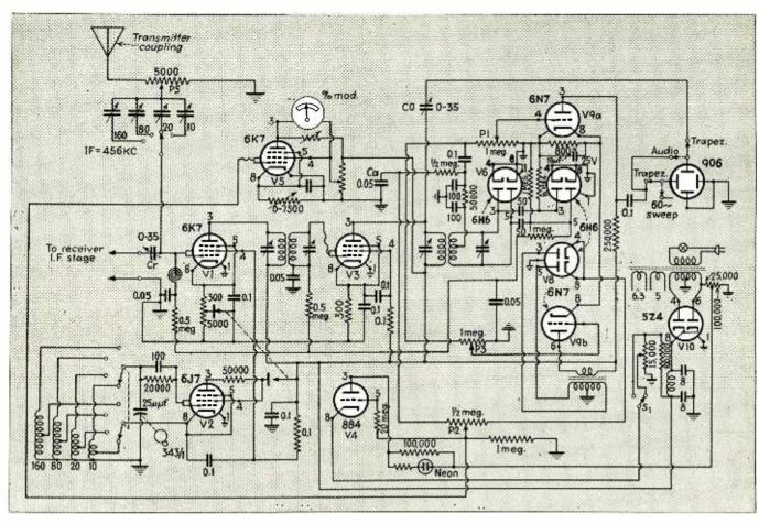
Fig. 6—Circuit diagram of the complete modulation monitor. It is connected to the final i-f stage of a receiver. For measuring a transmitted signal, the 5000-ohm portion of the  $V_1$  cathode resistor is cut in and the plate and screen circuits of  $V_2$  are closed
