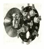
Coil assembly mounted on mycalex disc attached to switch system. Polystyrene coil insulation with unwound plug-in coil form for any additional frequency range desired; excellent electrical contact between silver-plated switch blades and contact springs.
