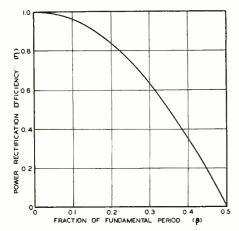
Fig. 5—Theoretical curve of power rectification efficiency versus the fraction of the fundamental period of flow during which current flows
