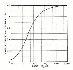
Fig. 7—Theoretical curve of the power rectification efficiency versus the ratio of the rectifier load resistance to internal plate resistance of the rectifier
