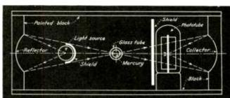
Figs. 3 and 4—Vertical and horizontal sections of the measuring unit. The height of the mercury column determines the amount of light reaching the phototube
