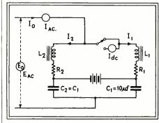
Fig. 3—Working circuit diagram for inductance measurement
