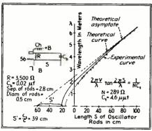
Fig. 1—Diagram showing the experimental and theoretical relations between the length of the oscillator rods and the wavelength of the generated oscillations for triodes
