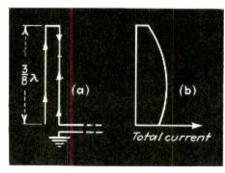
Fig. 5—A three-eights wave vertical antenna working against ground and its total current distribution
