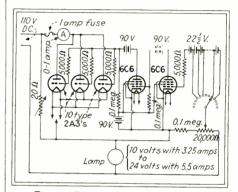
Fig. 1-Circuit of 5-ampere voltage regulator
