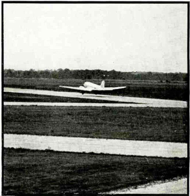
At the Indianapolis Airport, the test plane is being landed "blind" during tests of equipment built for the Civil Aeronautics Authority by the International Telephone Development Company. By keeping the cross-pointer meter (above, left) on center the pilot can reach the runway safely (above, right) even though the visibility is zero. The cover shows the control equipment of the installation, which includes 16 transmitters in all.
