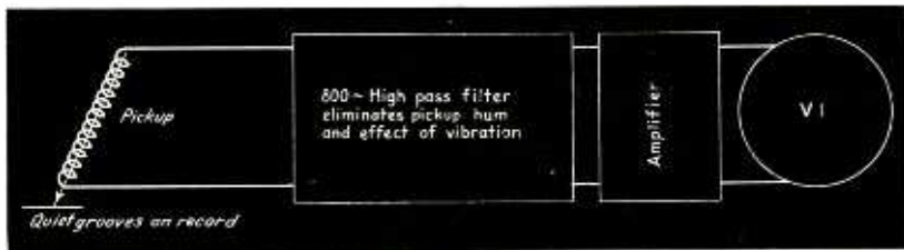
Basic method of measuring disc noise level, using a high-pass filter to eliminate low frequency effects
