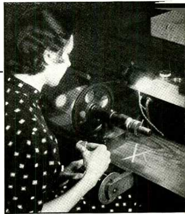
Closeup view of winding operation in voice-coil production
